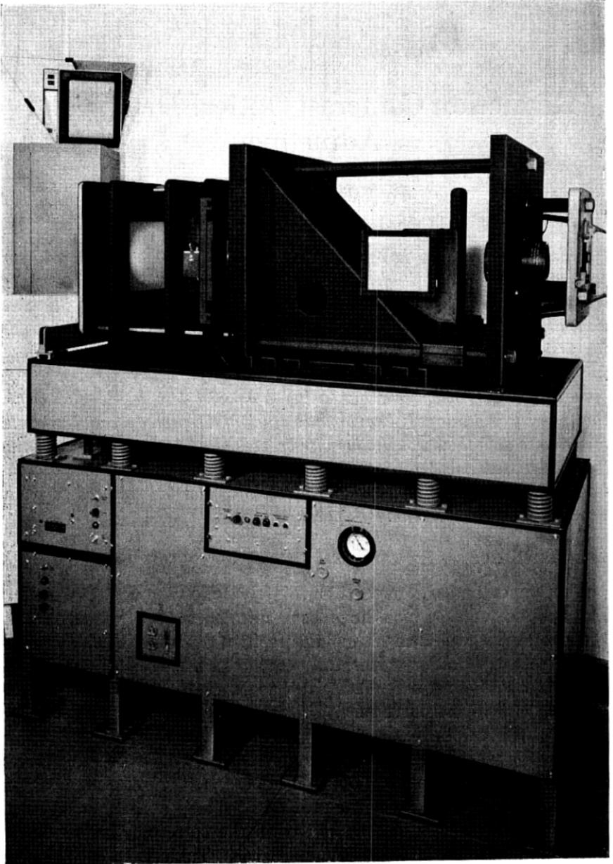
Fig. 1—The 3.5 $\times$  reduction camera.
