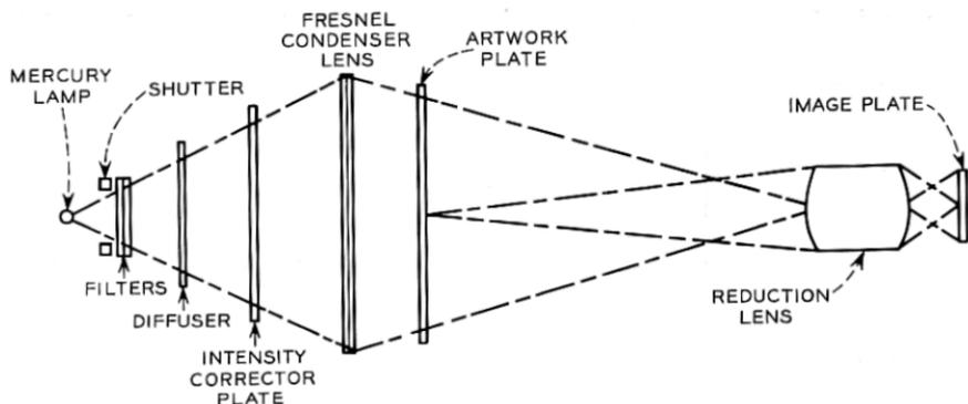
Fig. 2—Optical layout of the reduction cameras.
