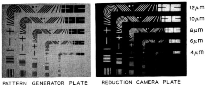
Fig. 8—Photomicrographs of an artwork resolution test pattern (left) and the corresponding image plate (right) taken with the 3.5 $\times$  camera. The image-plane linewidths are indicated at the right. The finest image linewidth required in normal use is 10 $\mu$ .
