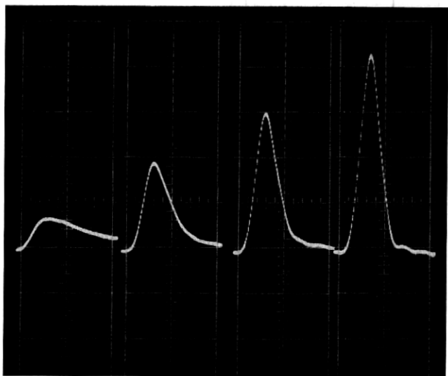
Fig. 26 — Pulse response of Schottky barrier photodiode at 0-volt, 4-volt, 15-volt, and 50-volt back bias. Horizontal scale 1 nsec/cm, vertical scale 25 mvolt/cm.
