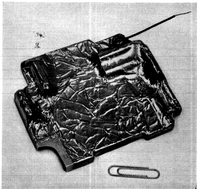
Fig. 10 — Electrostatic shield to isolate subassemblies of modem.
