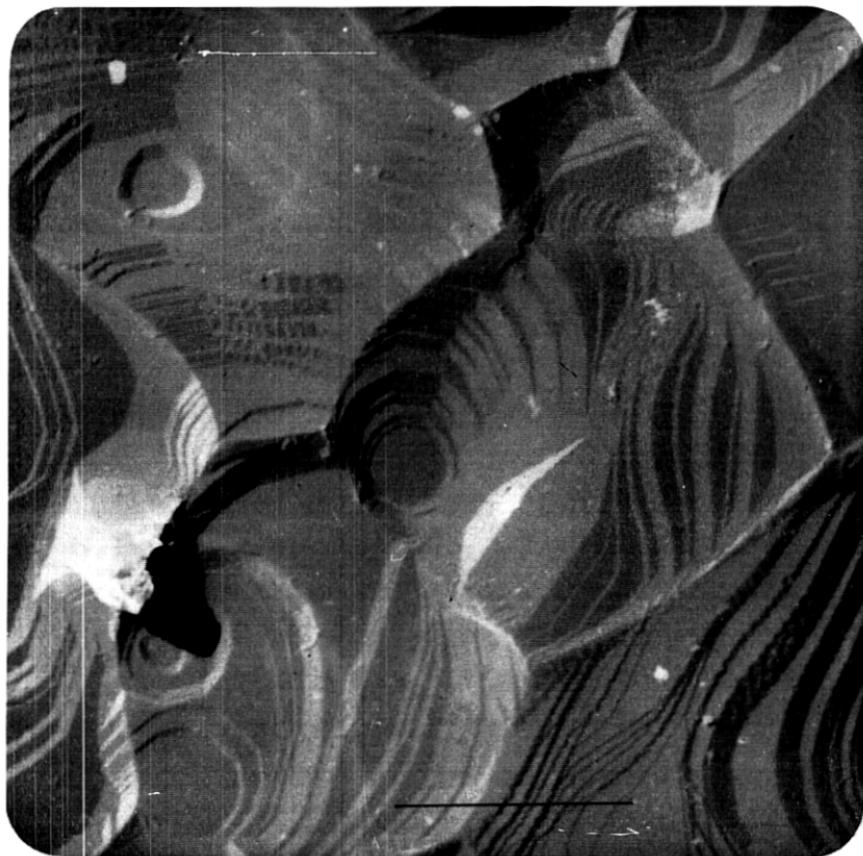
Fig. 14—Germanium replica ( $t_e \approx 150\text{\AA}$ ,  $\theta_a = 35^\circ$ ) of near optimum thickness. Resolution about  $75\text{\AA}$ . Ruptured film evident in shadow.
