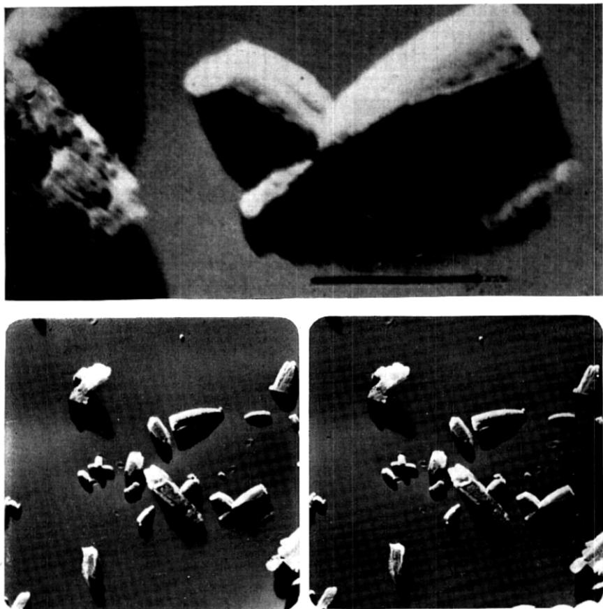
Fig. 3—Silica replica of particles and associated shadows.  $\theta_a = 60^\circ$ . Diffusing component replicates particles within shadows. Oval hole shows presence of film in shadow. Black lines =  $1 \mu$ .
