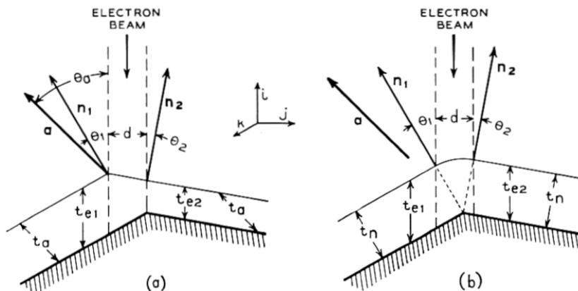
Fig. 2—Diagram showing resolution of replica film at a sharp corner. (a) Every atom sticks where it strikes. (b) All atoms diffuse, finally condensing into film of uniform local thickness.
