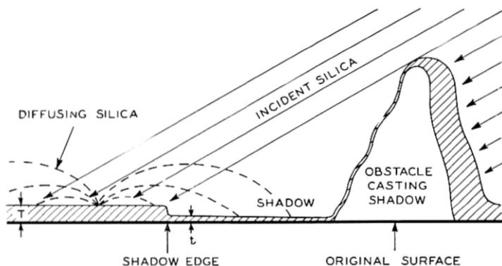
Fig. 4—Diagram illustrating diffusion of silica into shadowed regions.
