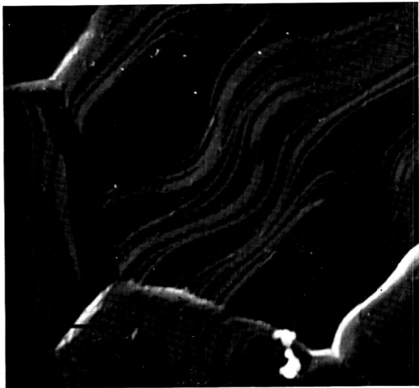
Fig. 13—Germanium replica ( $\bar{l}_e \approx 300\text{Å}$ ,  $\theta_a = 30^\circ$ ) of thermistor flake surface. Resolution about 150Å. Over-exposed appearance shows replica is thicker than optimum.
