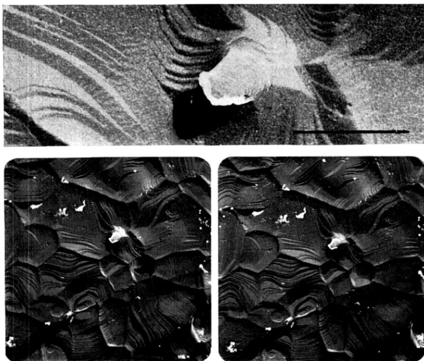
Fig. 10—Gold-manganin replica ( $t_e = 150\text{\AA}$ ,  $\theta_a = 20^\circ$ ). Resolution about  $100\text{\AA}$ . Replica is much thicker than optimum. A film in the shadow, clearly evident in the original micrograph, does not show except for two whitish areas where it has torn and curled.
