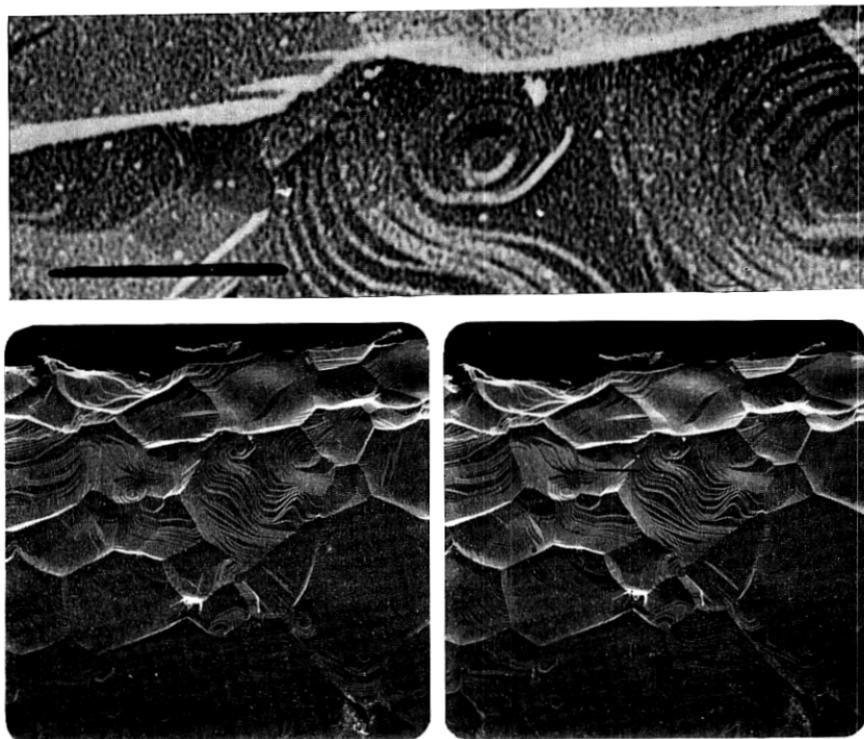
Fig. 9—Aluminum replica ( $l_e = 180 \text{ \AA}$ ,  $\theta_a = 30^\circ$ ) showing granularity due to recrystallization. Local curling of replica has resulted in "negative shadows" in upper left region of stereogram. Resolution about  $100 \text{ \AA}$ .
