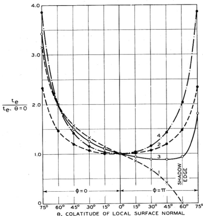
Fig. 16—Contrast-determining curves. (1)  $\theta_a = 30^\circ$ , every atom sticks where it strikes. (2)  $\theta_a = 0^\circ$ , half the atoms diffuse. (3)  $\theta_a = 30^\circ$ , half the atoms diffuse. (4)  $\theta_a = 0^\circ$ , all atoms diffuse over surface.
