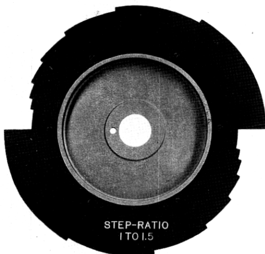
Fig. 6—Step sector disk used for plate calibration.
