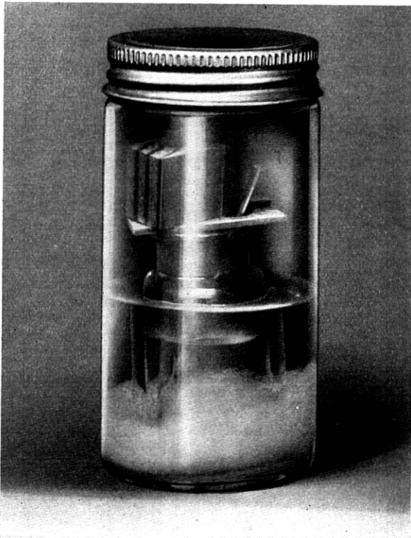
Fig. 4—Assembly of apparatus required for modified wood-block method of assay.
