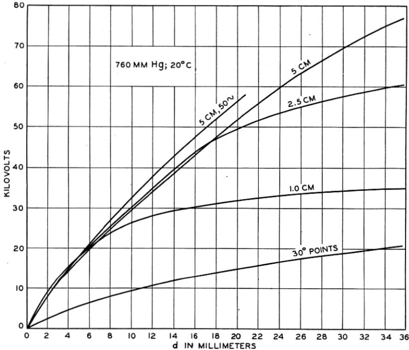
Fig. 14—Curves of sparking-potential vs. gap-width, in air, between spherical electrodes of the indicated radii, at frequencies of the order  $10^5$  (except the top-most). (Kampschulte, *Arch. f. Elektrotech.*)
