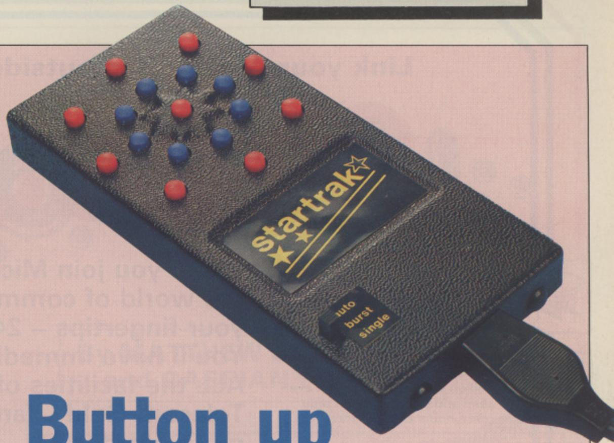
**JOYSTICKS** can cause endless problems – they don't move quickly enough and they also wear out rapidly. Star-Trak is a small hand-held pad which puts all possible stick-position and firebutton combinations on to individual keys to overcome these problems. So, for example, you can select "up-left" or "up-left-plus-fire" with a single touch.
