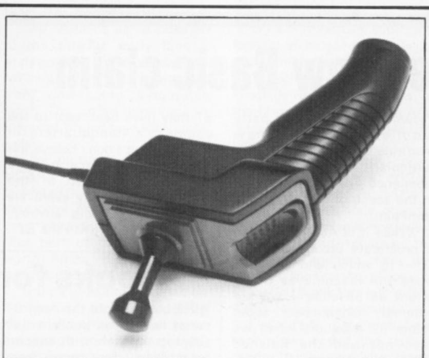
*ABANDONING conventional mechanical switching, Mastertronic has based its new joystick for the Atari range around micro-switches.*
