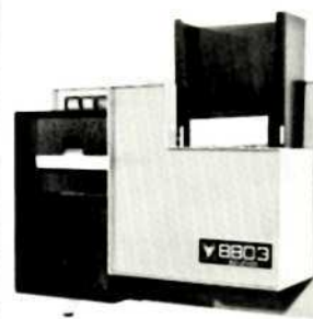
Model 8803-6: 80-column card, 51-column stub, 96-column card, and 96-column (Topless) stub reader for System/3 Mod 6. Identical to 8803-0, except that it connects to Mod 6.
