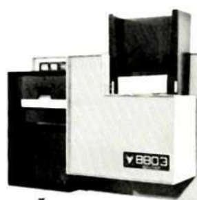
Model 8803-0: 80-column card, 51-column stub, 96-column card, and 96-column (Topless) stub reader for System/3 Mod 10. One reader reads all. Connects directly to the Mod 10 Central Processing Unit (CPU). With the MFCU, it gives you a third input hopper to the Mod 10. Operator changes from 80-column cards to 96-column cards within 30 seconds by changing the hopper and stacker.
