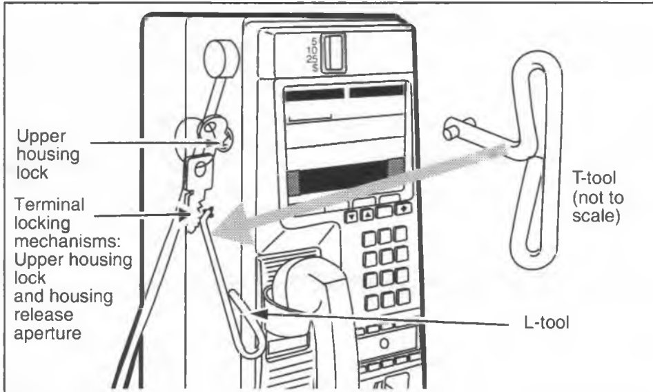
Figure 7-1: Locating the locking mechanisms for the upper housing
