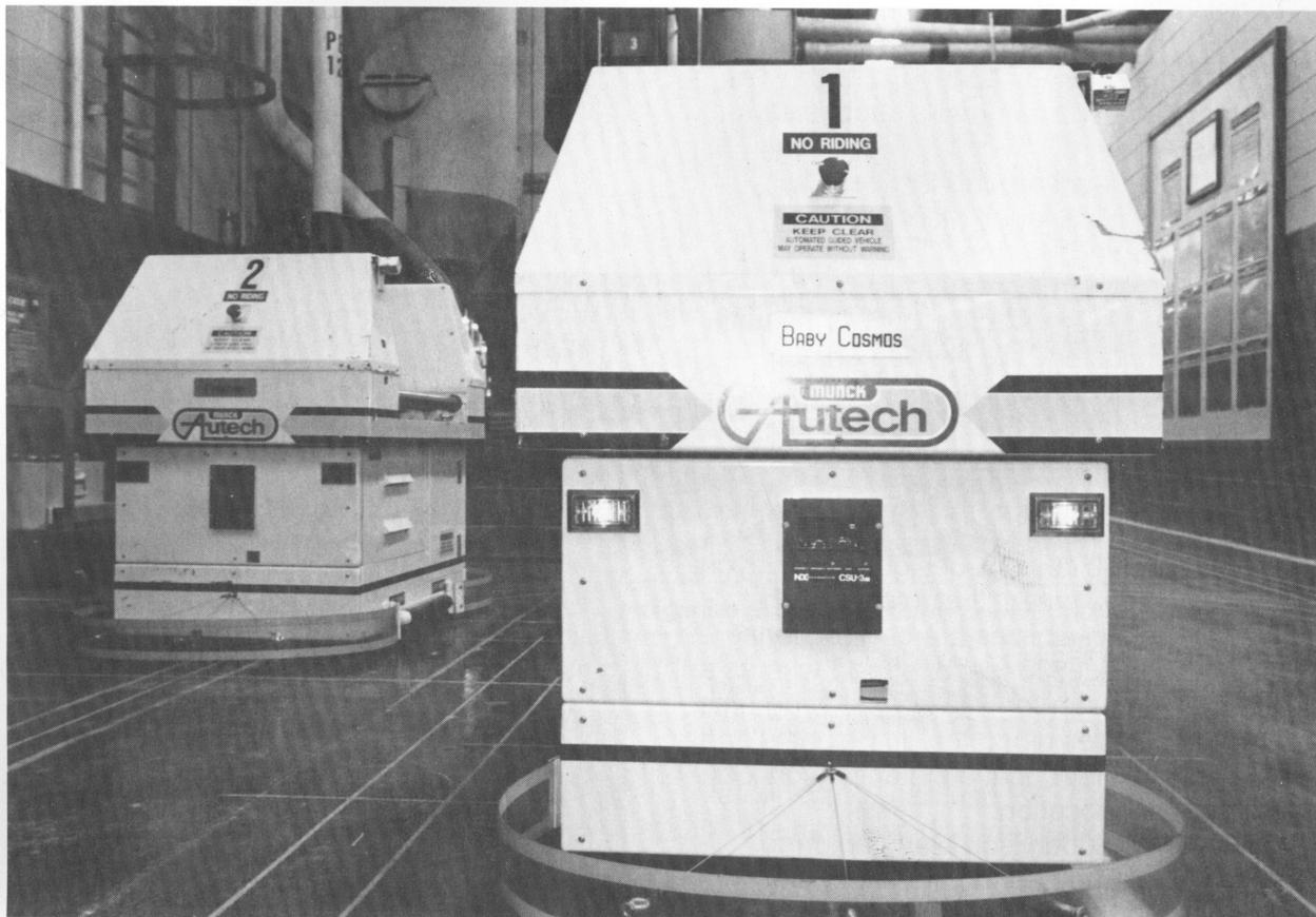
*Baby Cosmos (right) and Marathon stand ready to move assembly components from one work area to another. These units are GTE's first Automatic Guided Vehicles to serve printed circuit board fabrication and fine-line departments.*
