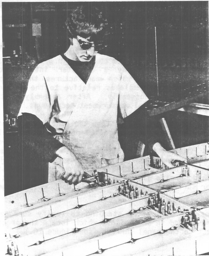
Figure 8. Fabrication of Reflector Panel in Panel Fixture
