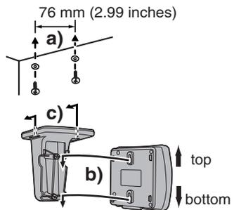
b), c): Fix the unit tightly by sliding it.
