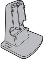
A camera stand with a base and a vertical support for the camera.          |
