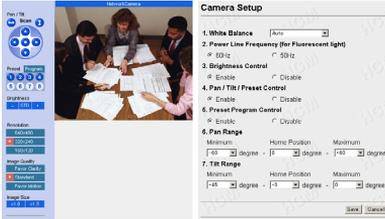
4. Adjust the Pan operation on the Single Camera screen and select **[Current]** in the minimum value data field of the Pan range on Camera Setup window. The data field refreshes to read the current value of the Pan range.
