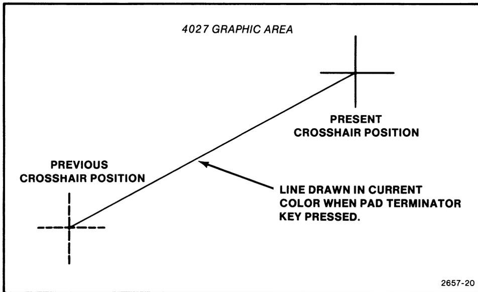
Figure 8-6. Drawing a Line in INK mode.
