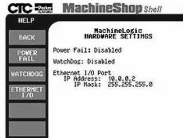
**Power Fail** The Power Fail feature is designed to protect the system in the event of an uncontrolled power loss. The power fail detection circuit on the MLSC monitors the system voltage. When the +5 Volts supply drops below 4.75 Volts, it will generate an interrupt to shutdown the I/O and de-energize the MCR. This relay can be used as an external indicator as part of an emergency stop circuit.
