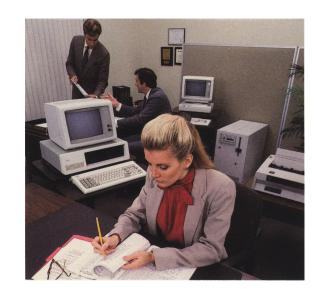
System/36 storage media include fixed disks, diskettes and a tape capability for inexpensive storage of information that is not needed on a daily basis. To help ensure smooth, non-disruptive system growth, System/36 memory and disk capacities can be expanded as your information and application requirements change. And, System/36 equipment is simple enough for you to set up yourself. So you can put it where you want to, when you want to —and move it easily as your business grows and changes.
