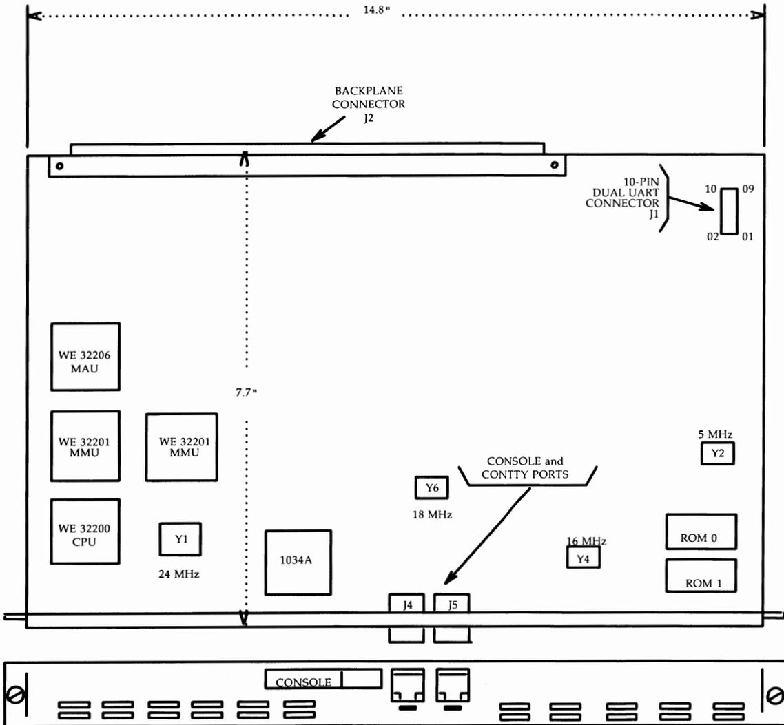
Figure B-5: CM518C System Board Layout
