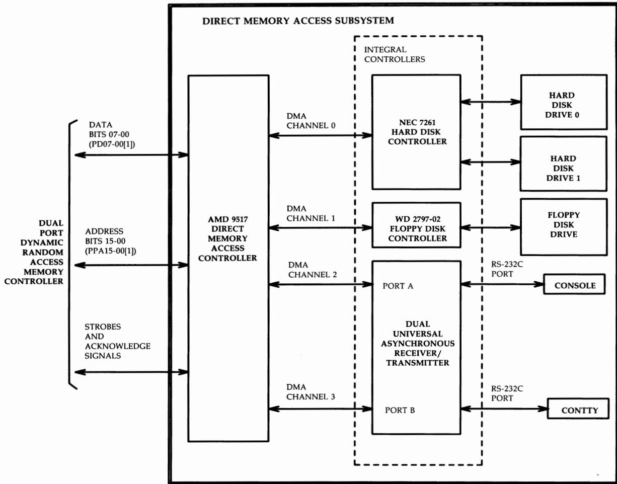
Figure 3-26: Direct Memory Access Subsystem — Functional Block Diagram
