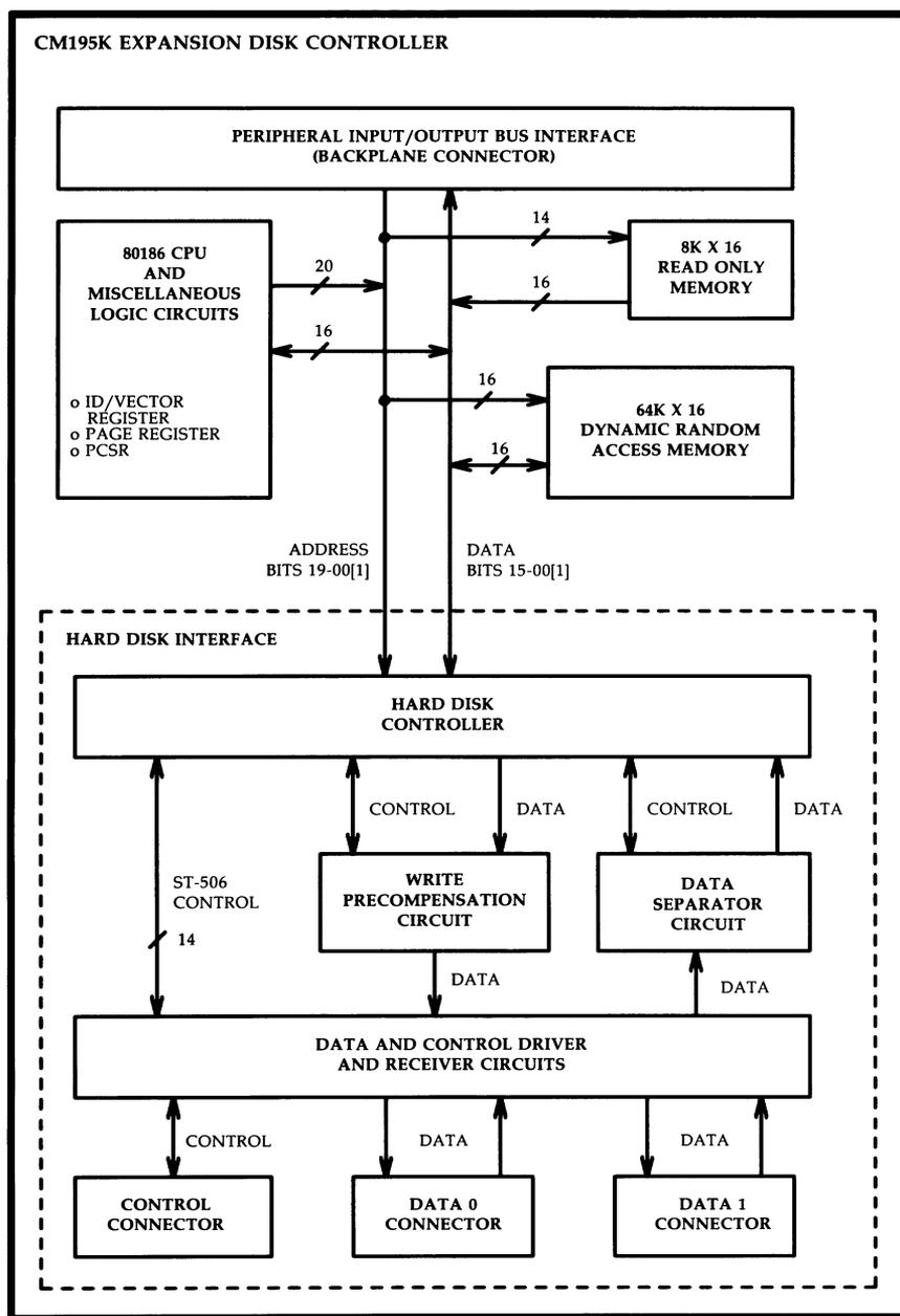
Figure 3-67: CM195K XDC Card — Functional Block Diagram
