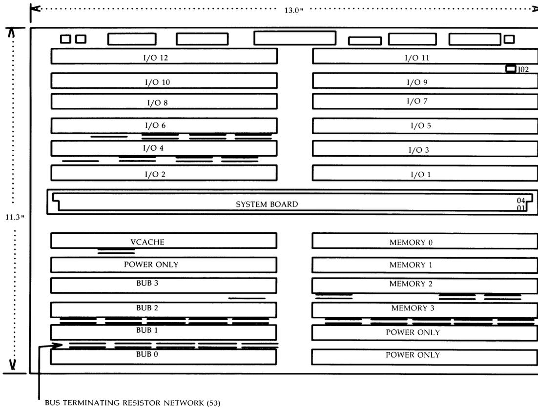
Figure 2-39: CM519A Backplane Board Layout
