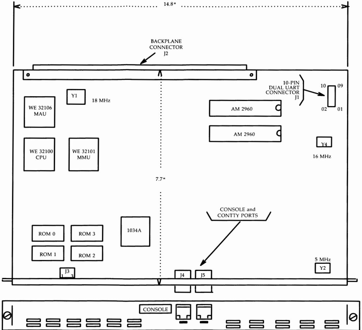
Figure B-3: CM518A System Board Layout
