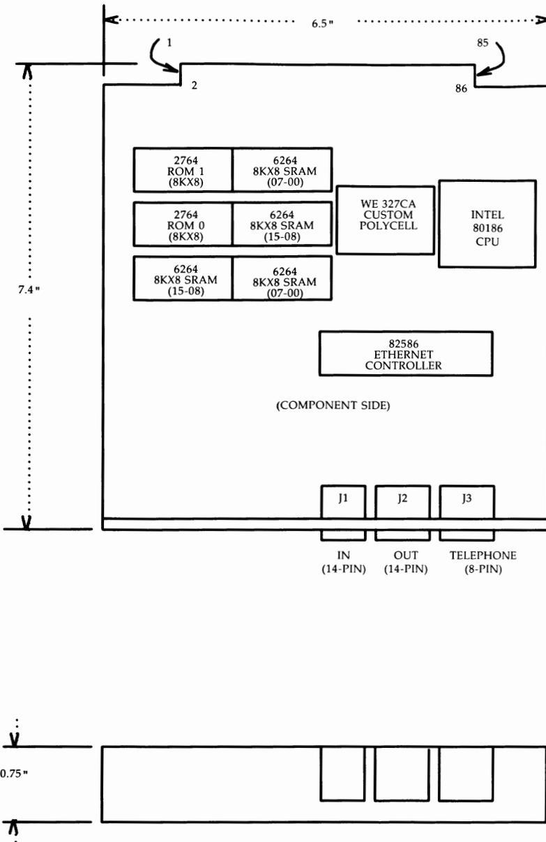
Figure B-29: CM195U STARLAN Interface Card Layout
