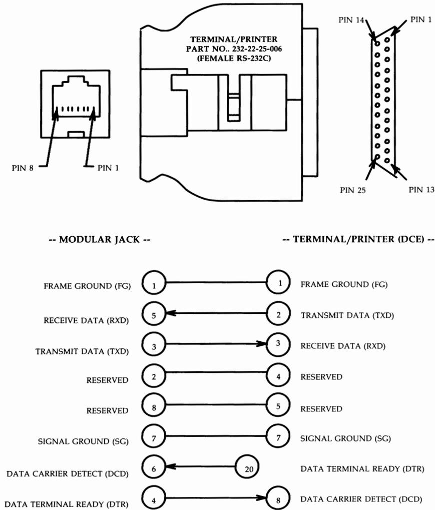
Figure B-38: Terminal/Printer Female Connector (232-22-25-006) Pin Identification
