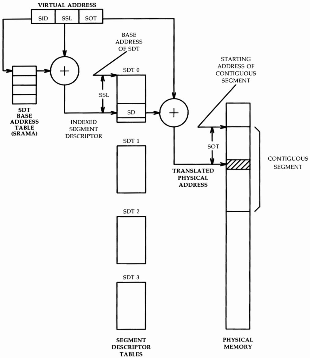
Figure 3-18: Virtual Address to Physical Address Translation for Contiguous Segments
