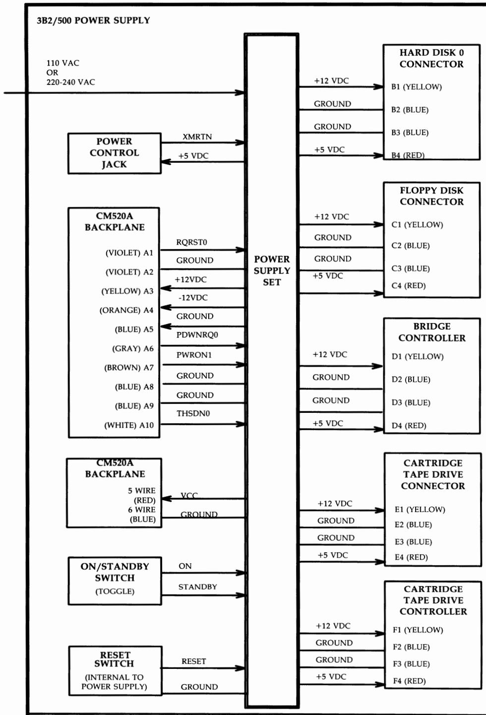
Figure 3-100: 3B2/500 Computer Power Supply — Functional Block Diagram
