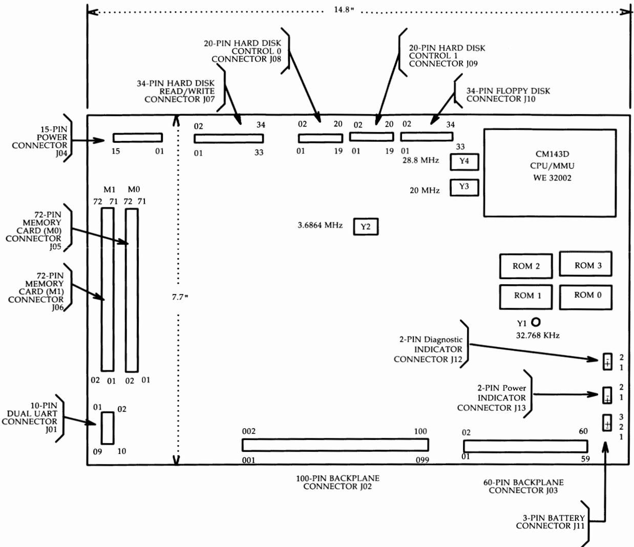
Figure B-1: CM190A System Board Layout
