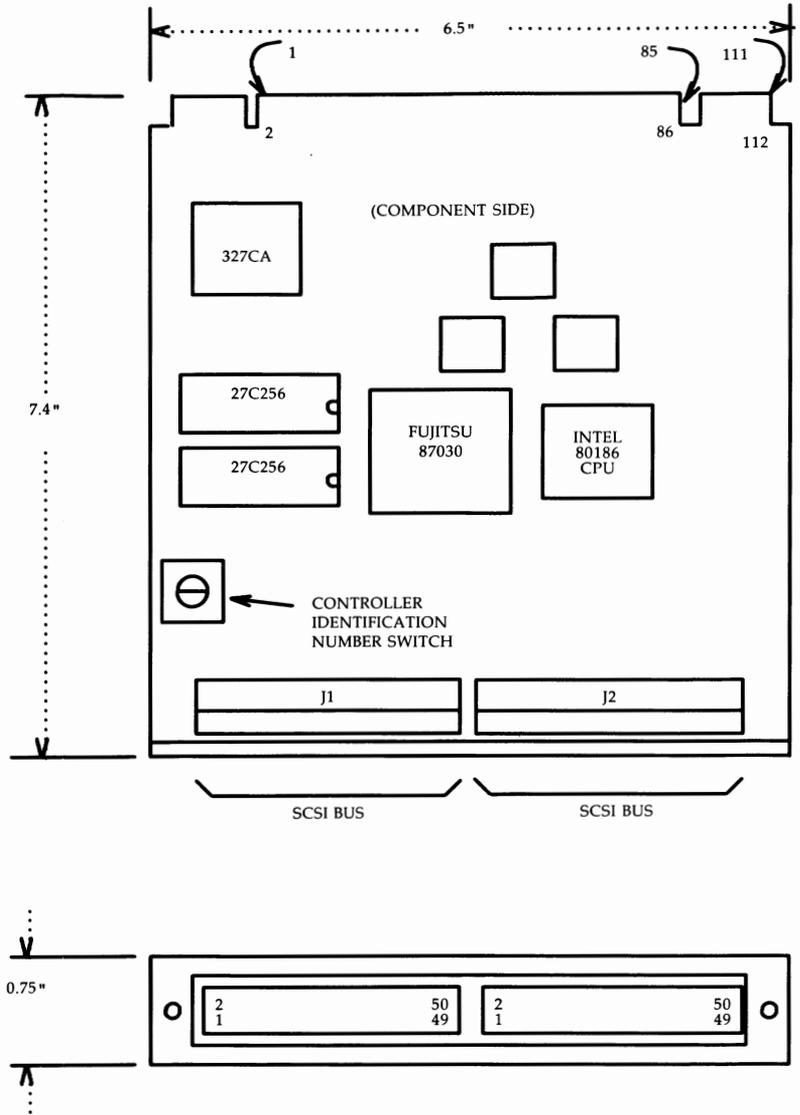
Figure B-31: CM521A Differential SCSI Host Adapter Card Layout
