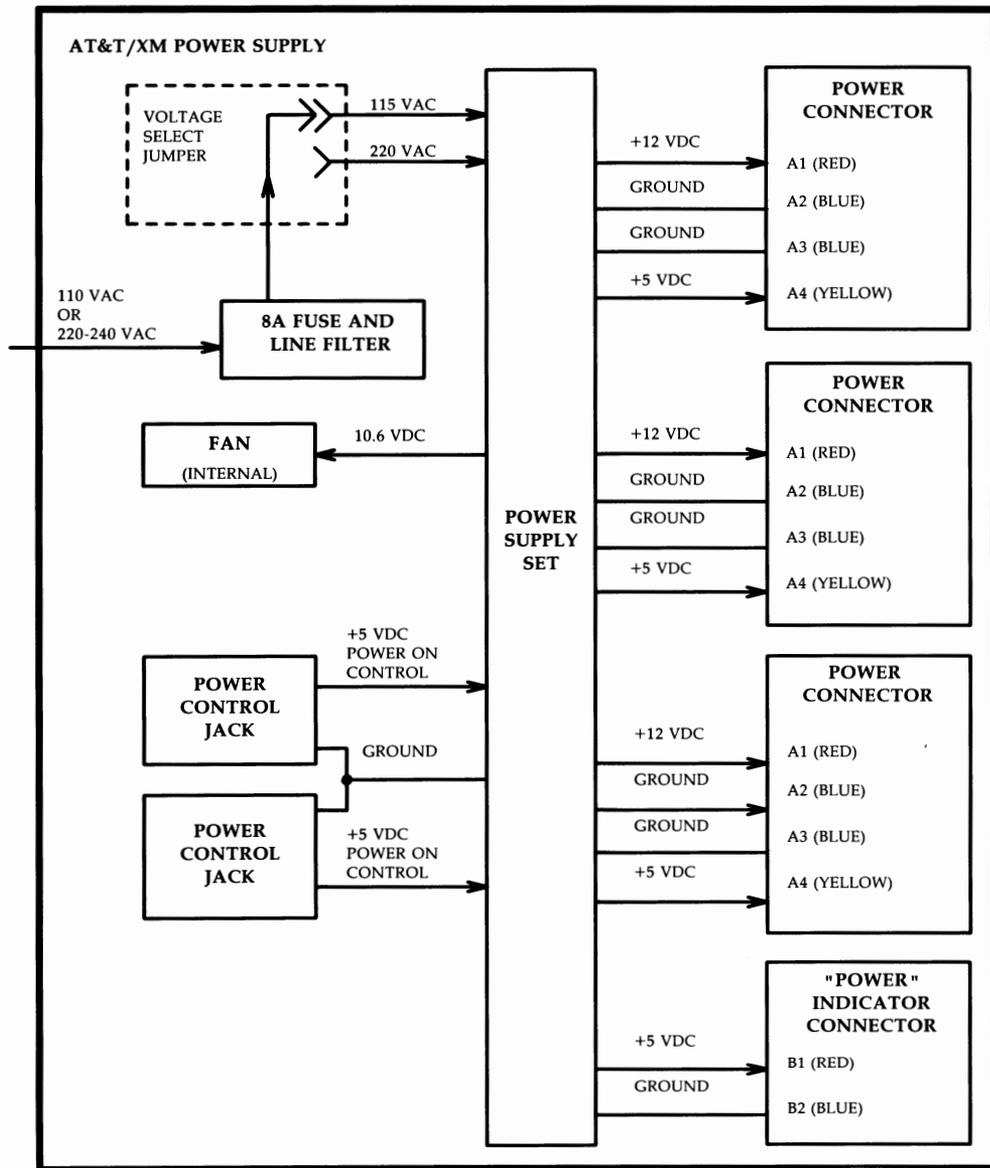
Figure 3-104: AT&T/XM Power Supply — Functional Block Diagram
