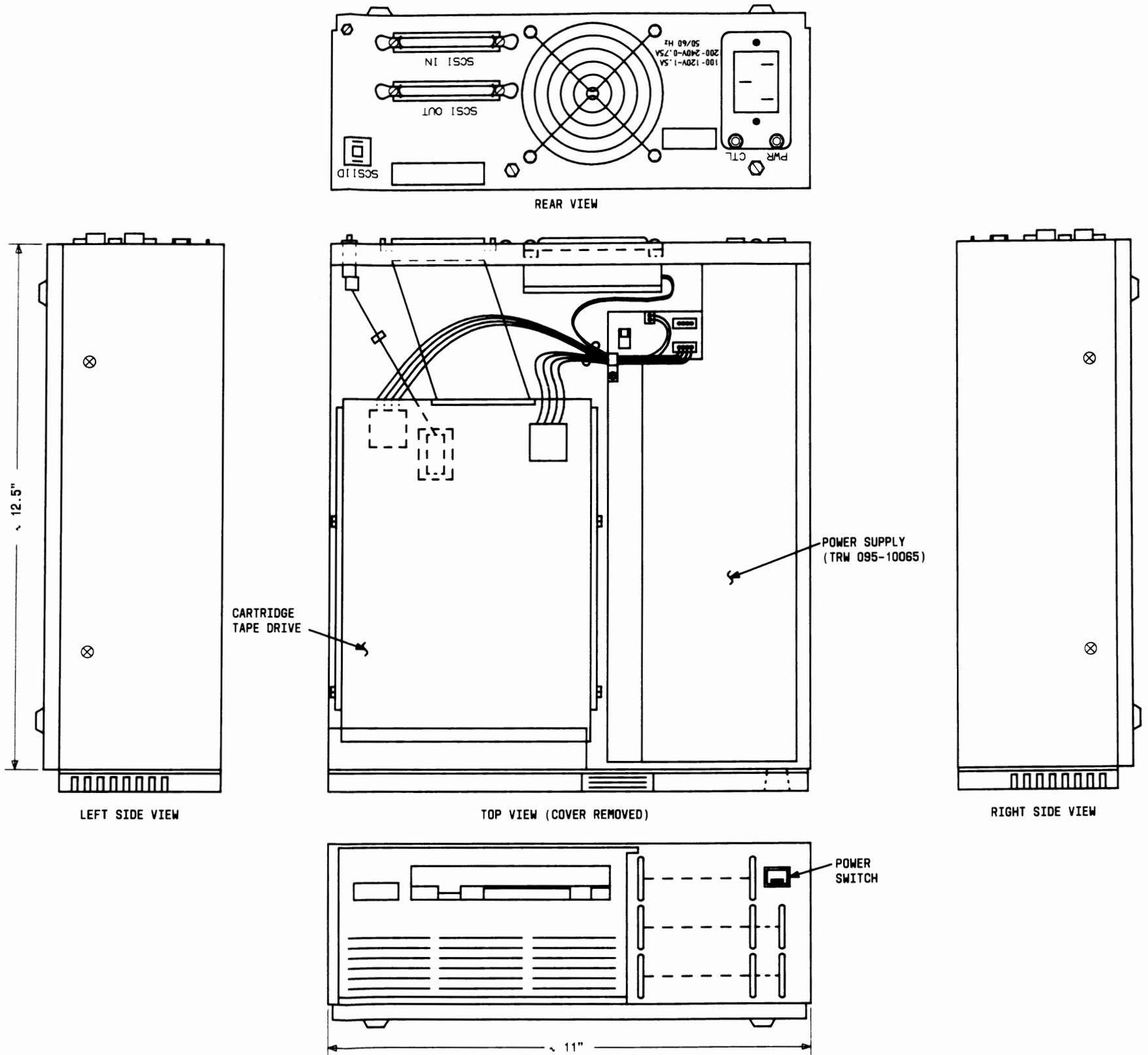
Figure 2-21: AT&T SCSI TM Cabinet Assembly Drawing (ED-3T011-30, G4, G7)
