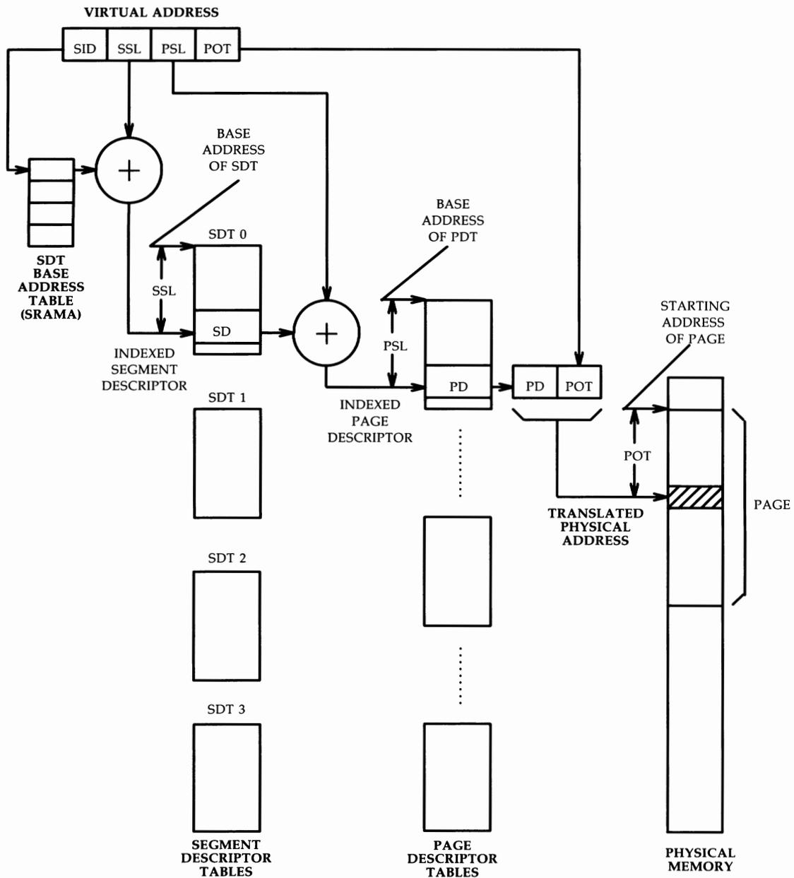
Figure 3-19: Virtual Address to Physical Address Translation for Paged Segments
