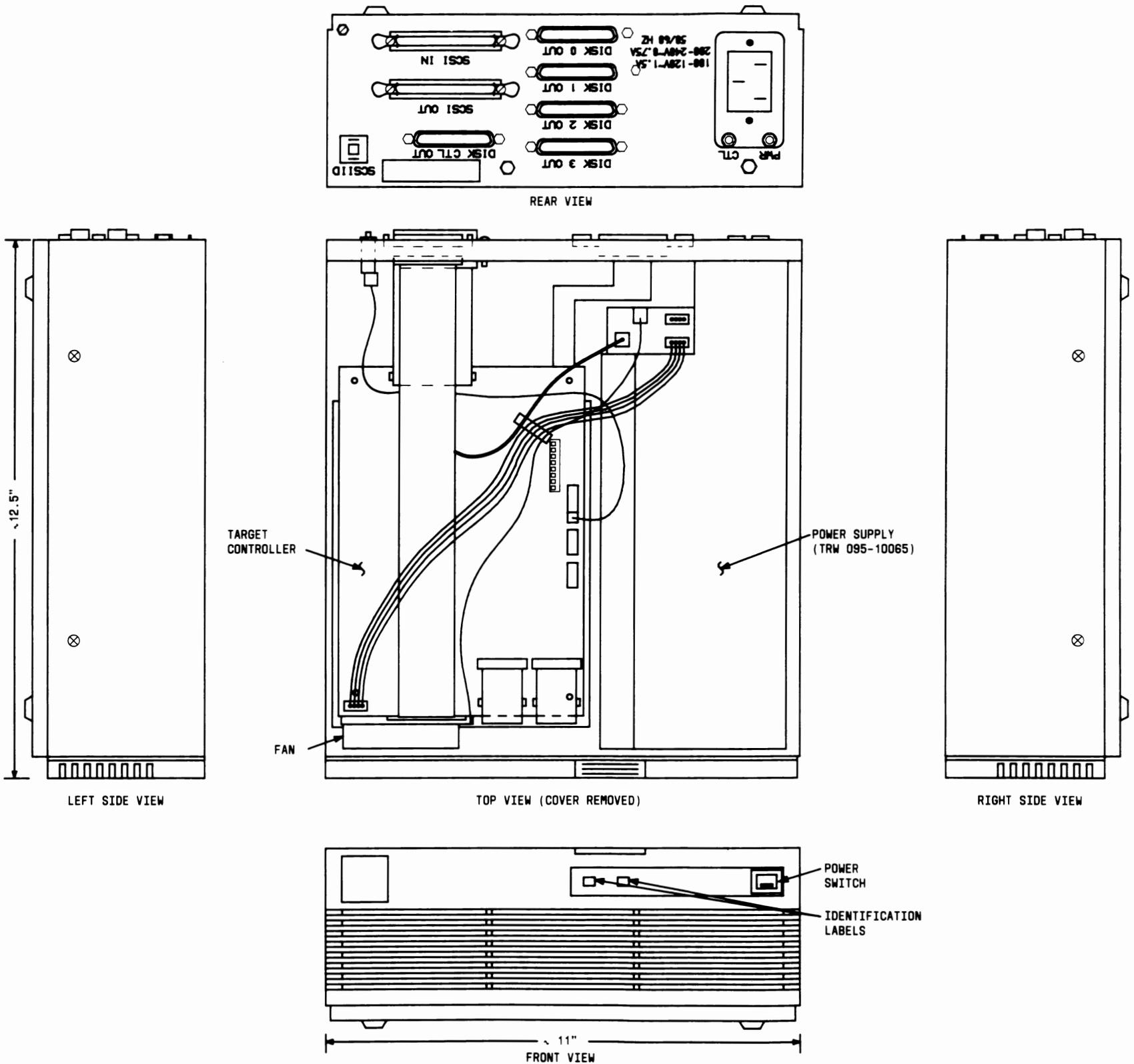
Figure 2-15: AT&T DCM/4E Cabinet Assembly
