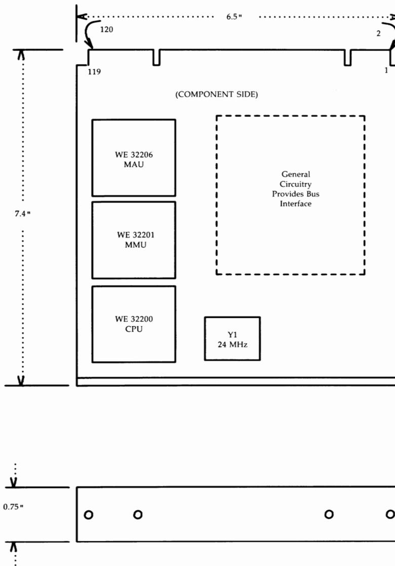
Figure 2-60: CM524A PE Card Layout
