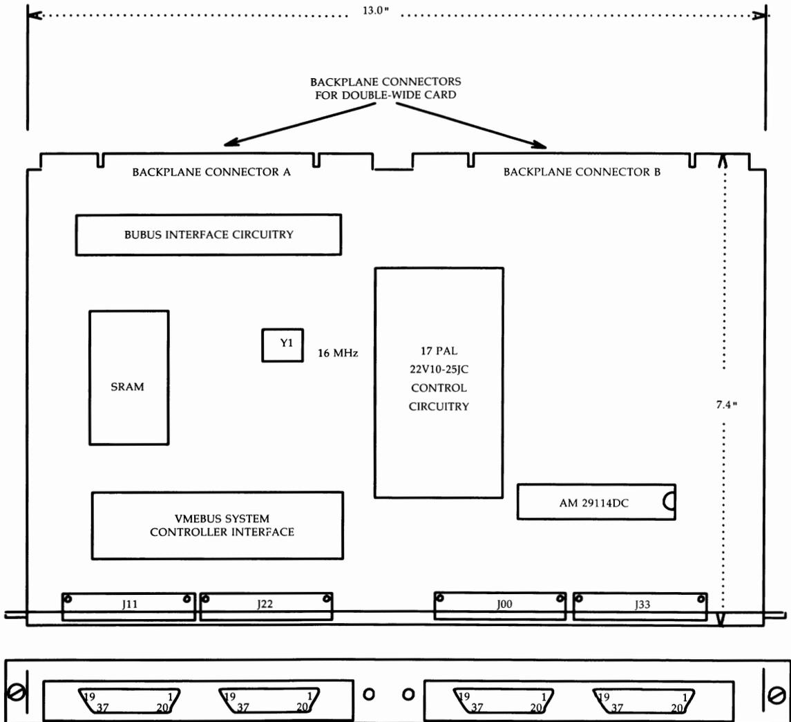
Figure B-34: CM525B VMEbus Card Layout
