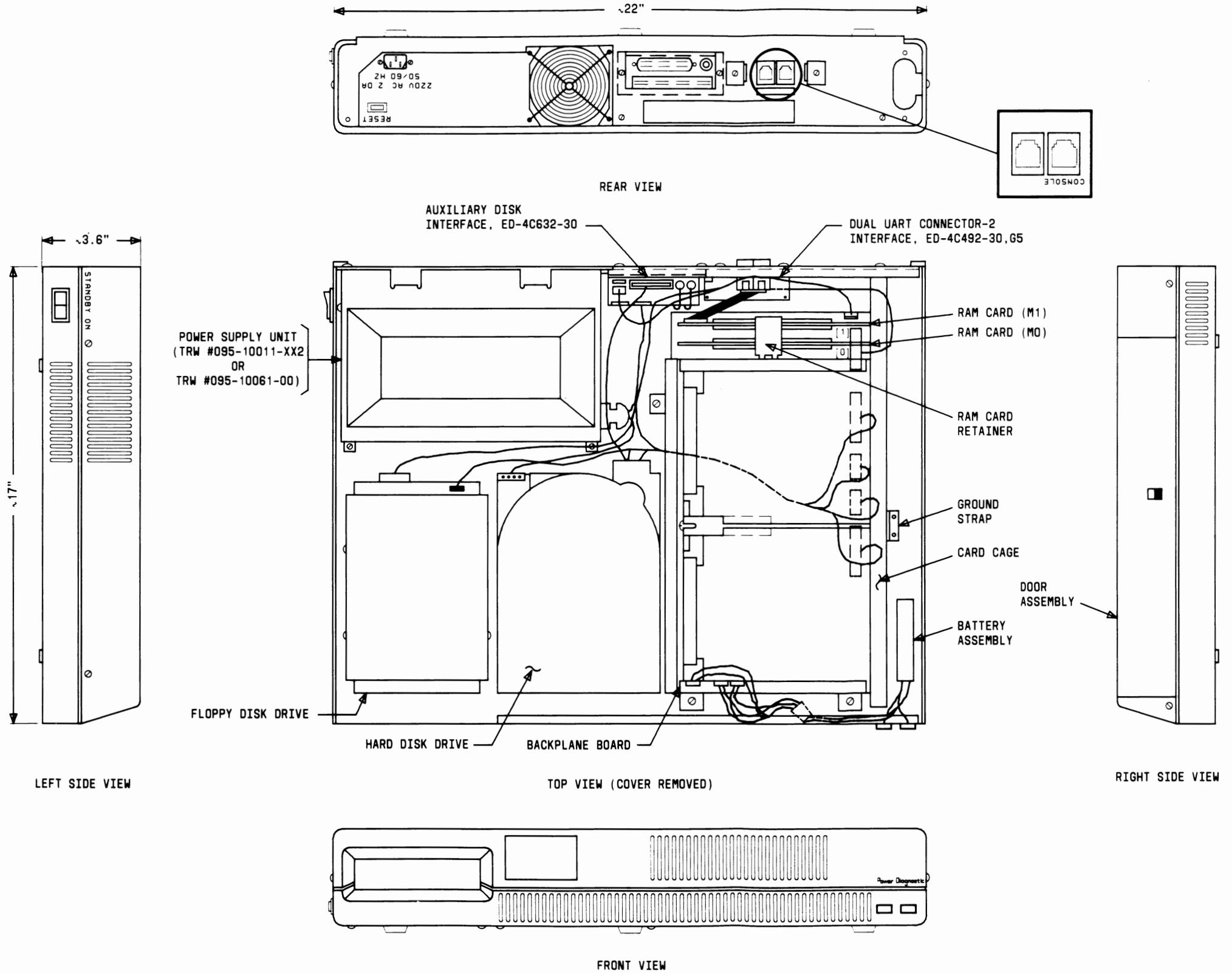
Figure 2-4: International 3B2/310 Computer Cabinet Assembly Drawing (ED-4C646-30)
