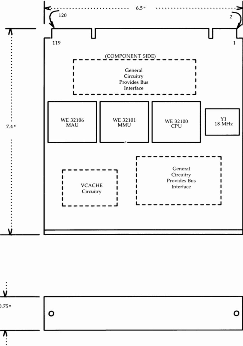
Figure 2-62: CM527A MPE Card Layout
