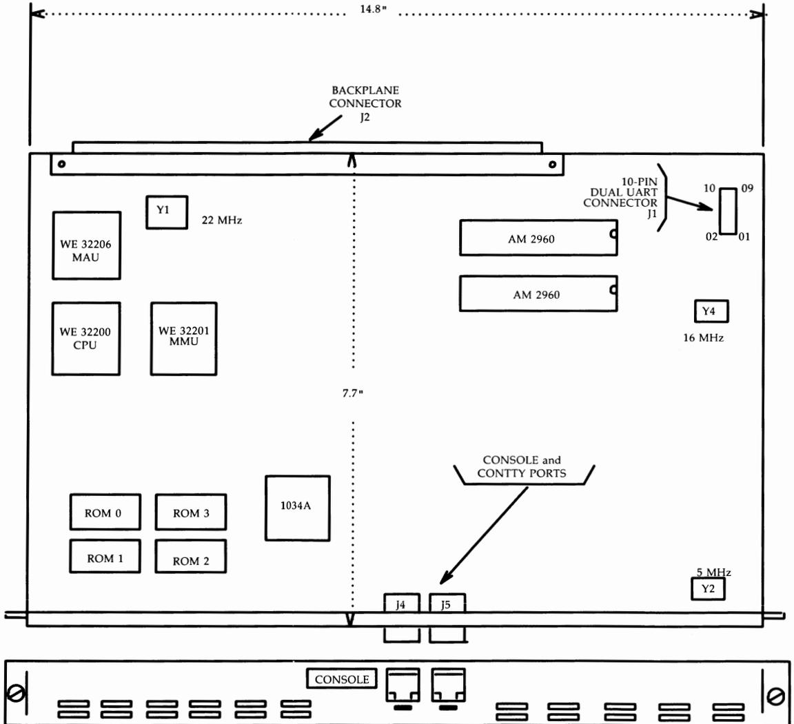
Figure B-4: CM518B System Board Layout
