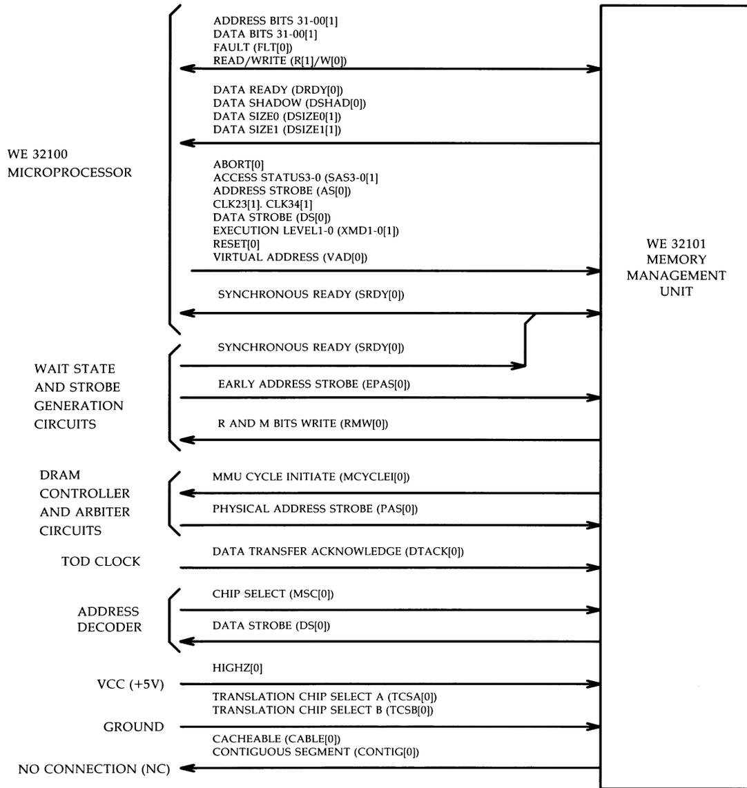
Figure 3-15: WE 32101 MMU Interconnection Diagram
