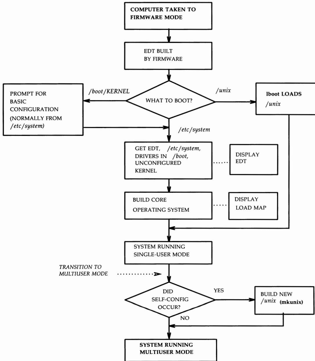
Figure 3-11: Self-Configuration — Manual Boot Sequence
