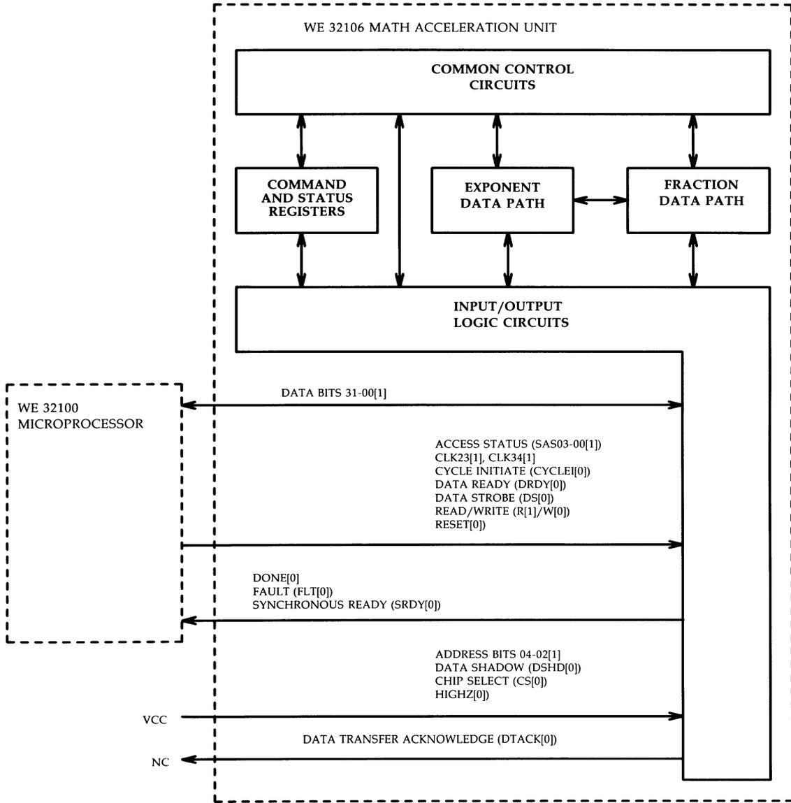
Figure 3-20: WE 32106 Math Acceleration Unit — Functional Block Diagram
