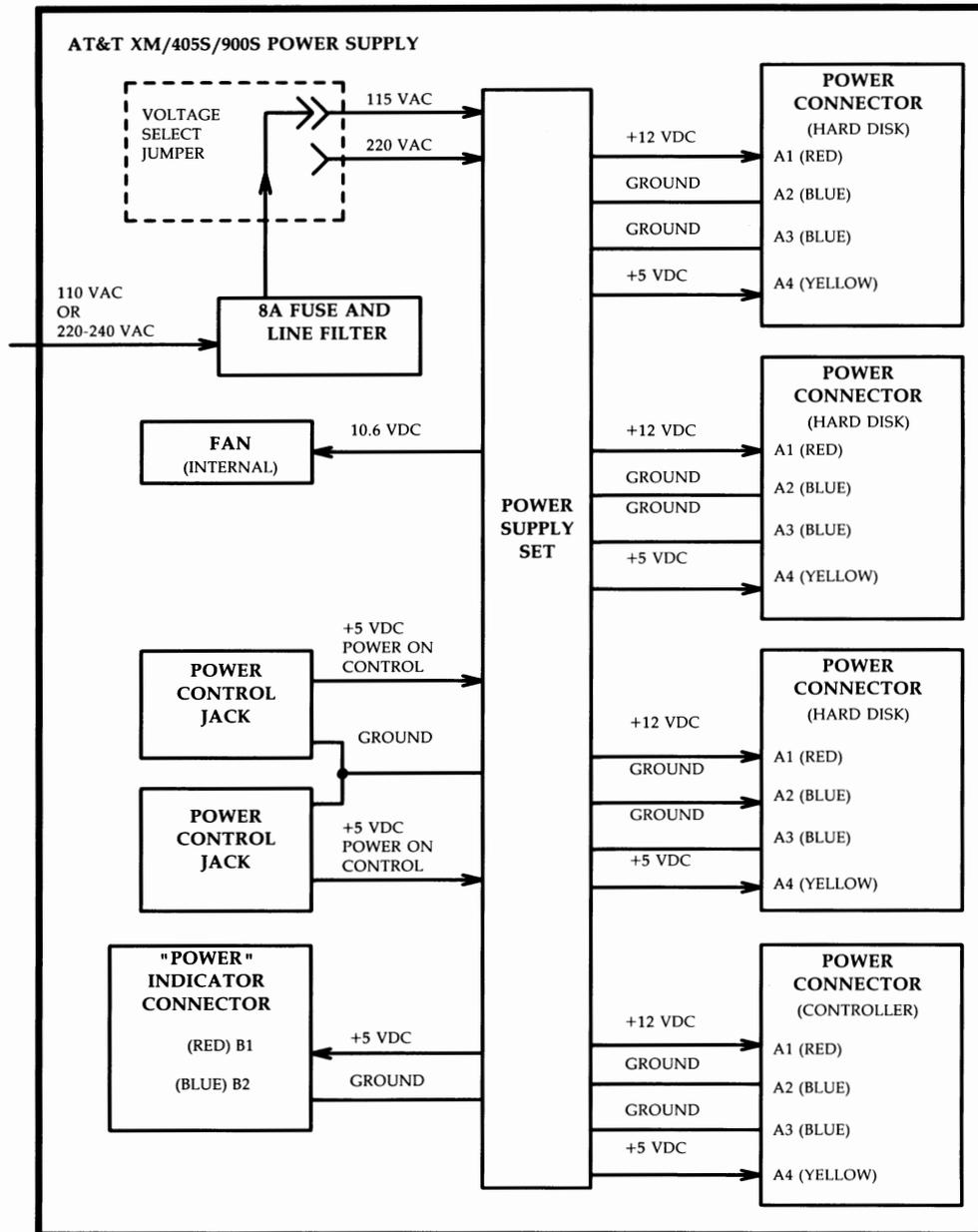
Figure 3-105: AT&T XM/405S/900S Power Supply — Functional Block Diagram
