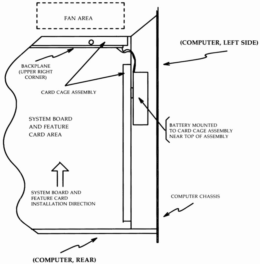
Figure 2-65: 3B2/600, 700, and 1000 Computer Backup Battery Supply Position
