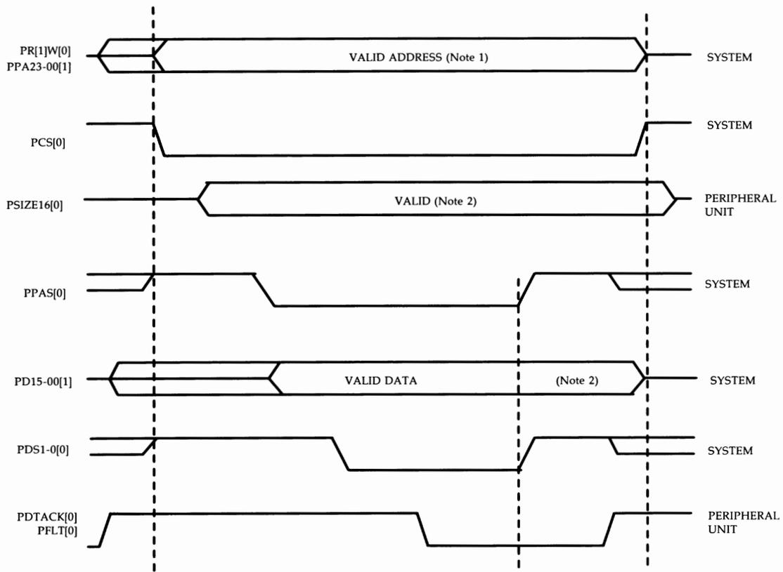
Note 1: PSIZE16[0] must be valid at system board for at least 20 nanoseconds before PDS1-0[0].
