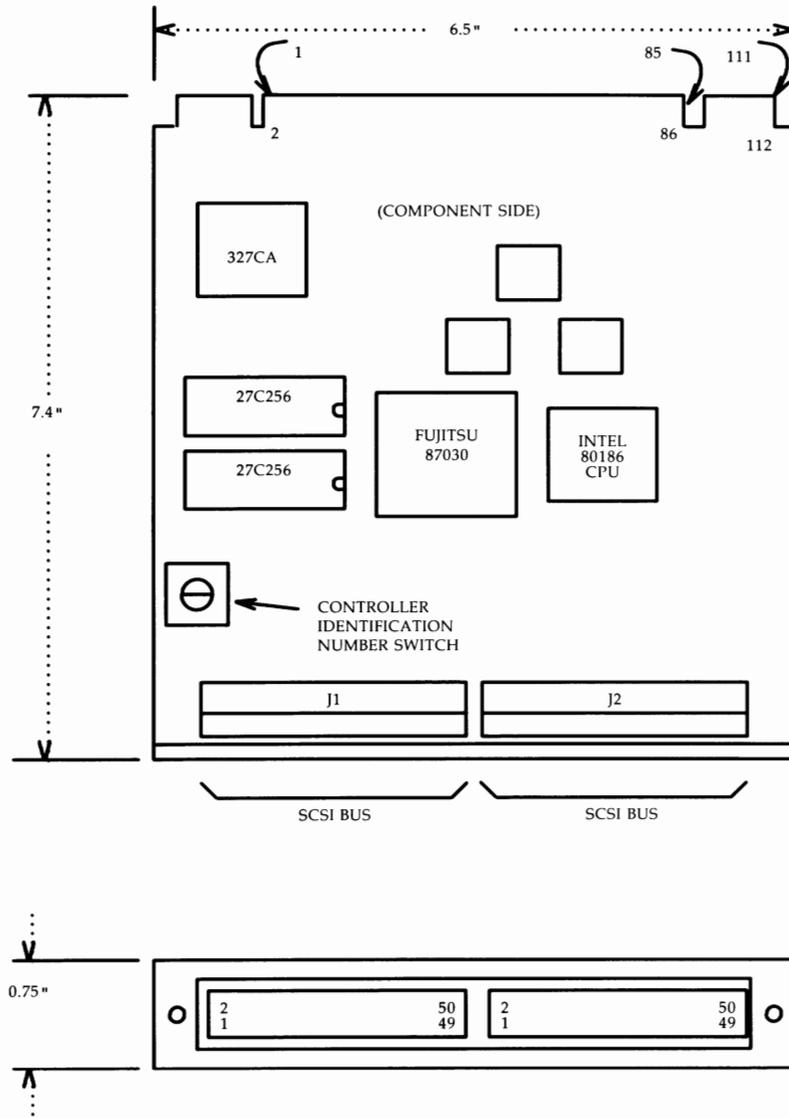
Figure 2-58: CM521A Differential SCSI Host Adapter Card Layout
