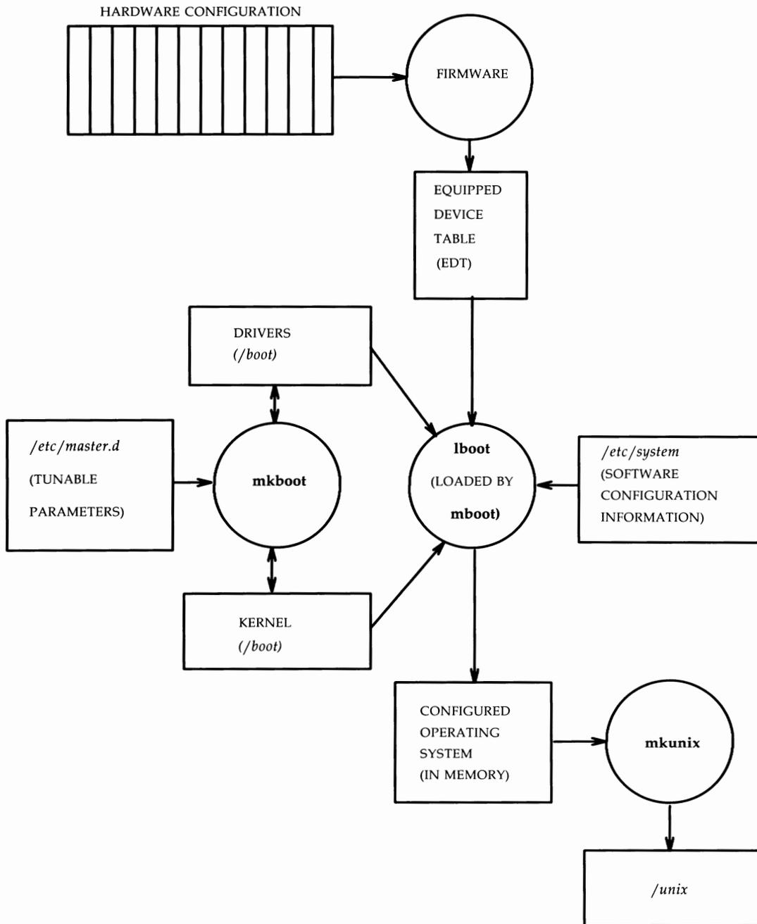
Figure 3-12: Self-Configuration Process
