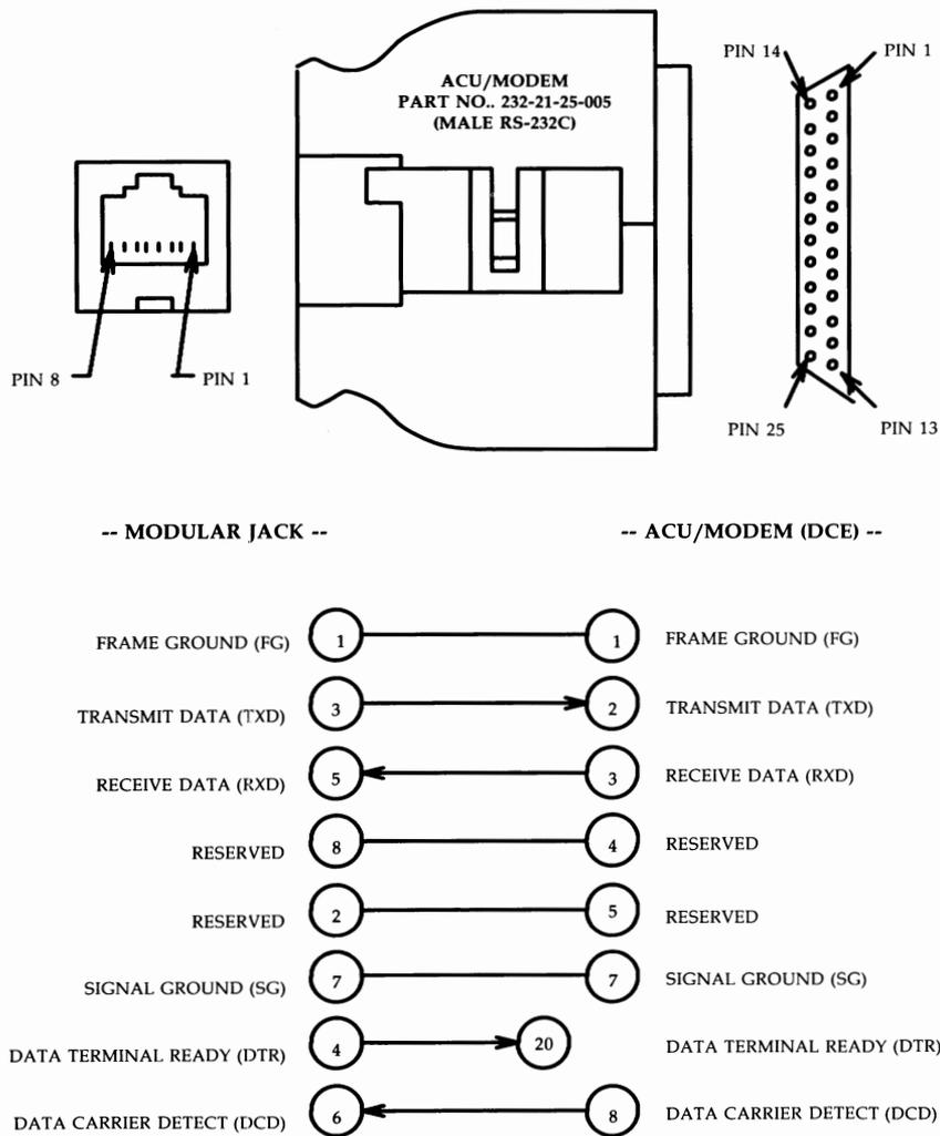
Figure B-37: ACU/MODEM Connector (232-21-25-005) Pin Identification
