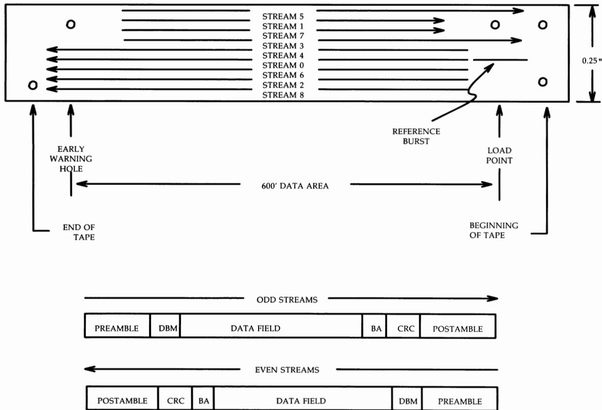
Figure 3-91: 60-Megabyte Cartridge Tape Physical Layout
