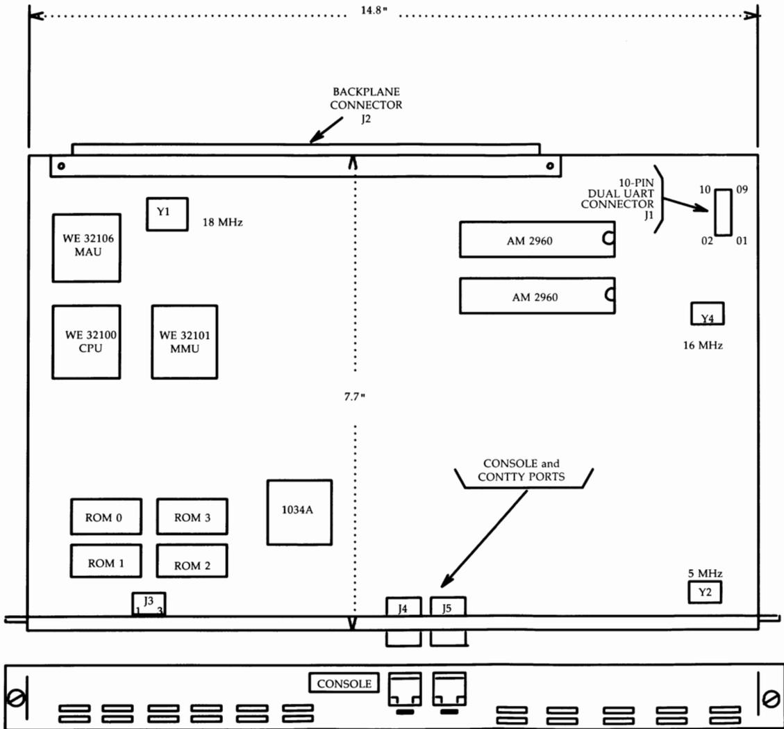
Figure 2-25: CM518A System Board Layout
