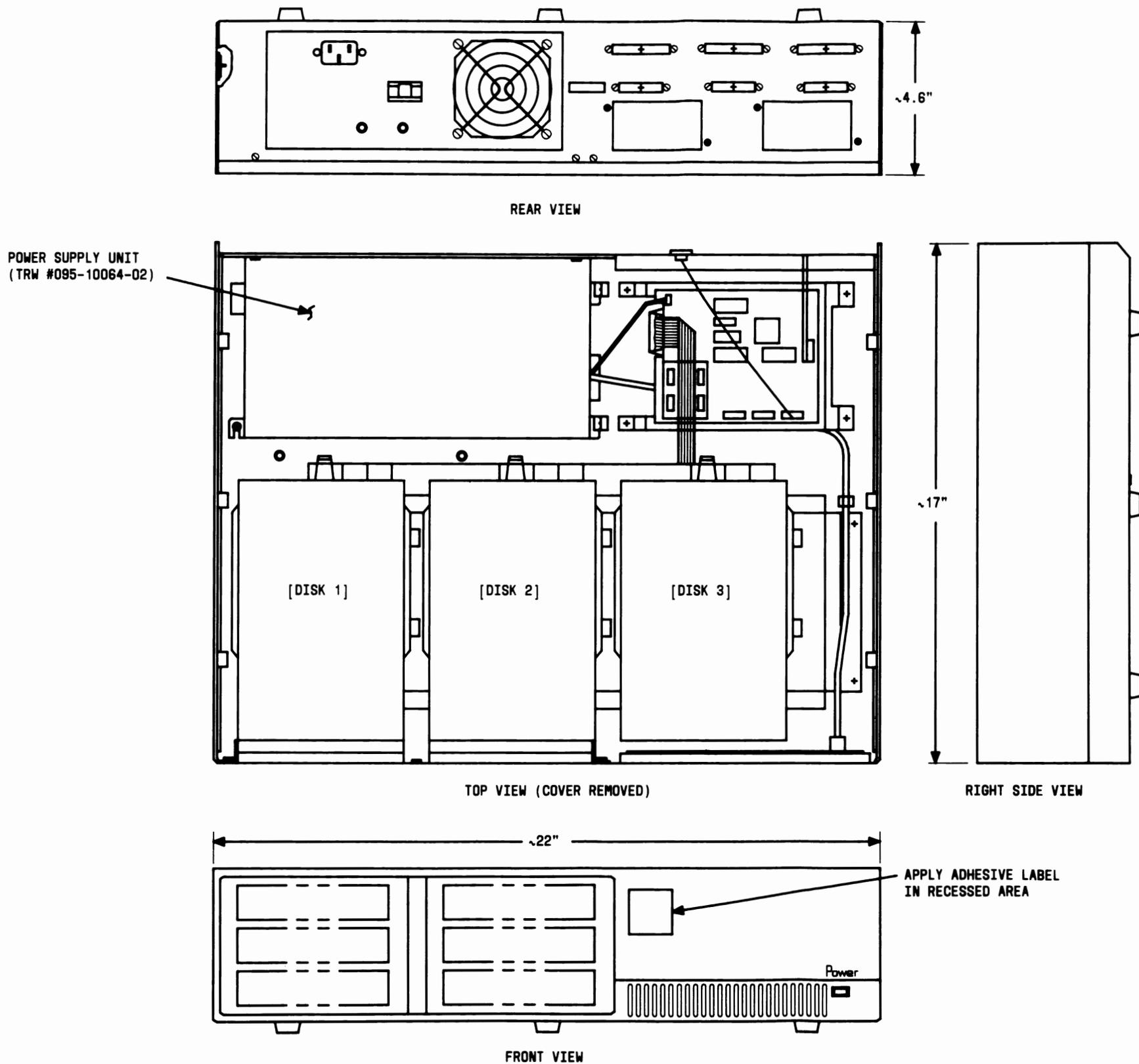
Figure 2-13: Domestic AT&T XM/405S/900S Cabinet Assembly Drawing (ED-3T010-30)
