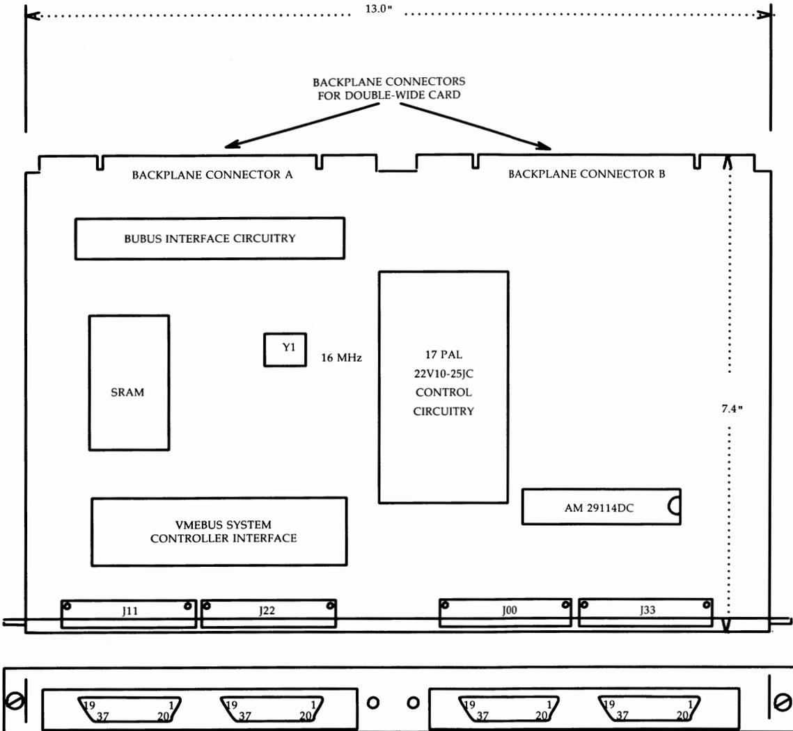
Figure B-34: CM525B VMEbus Card Layout
