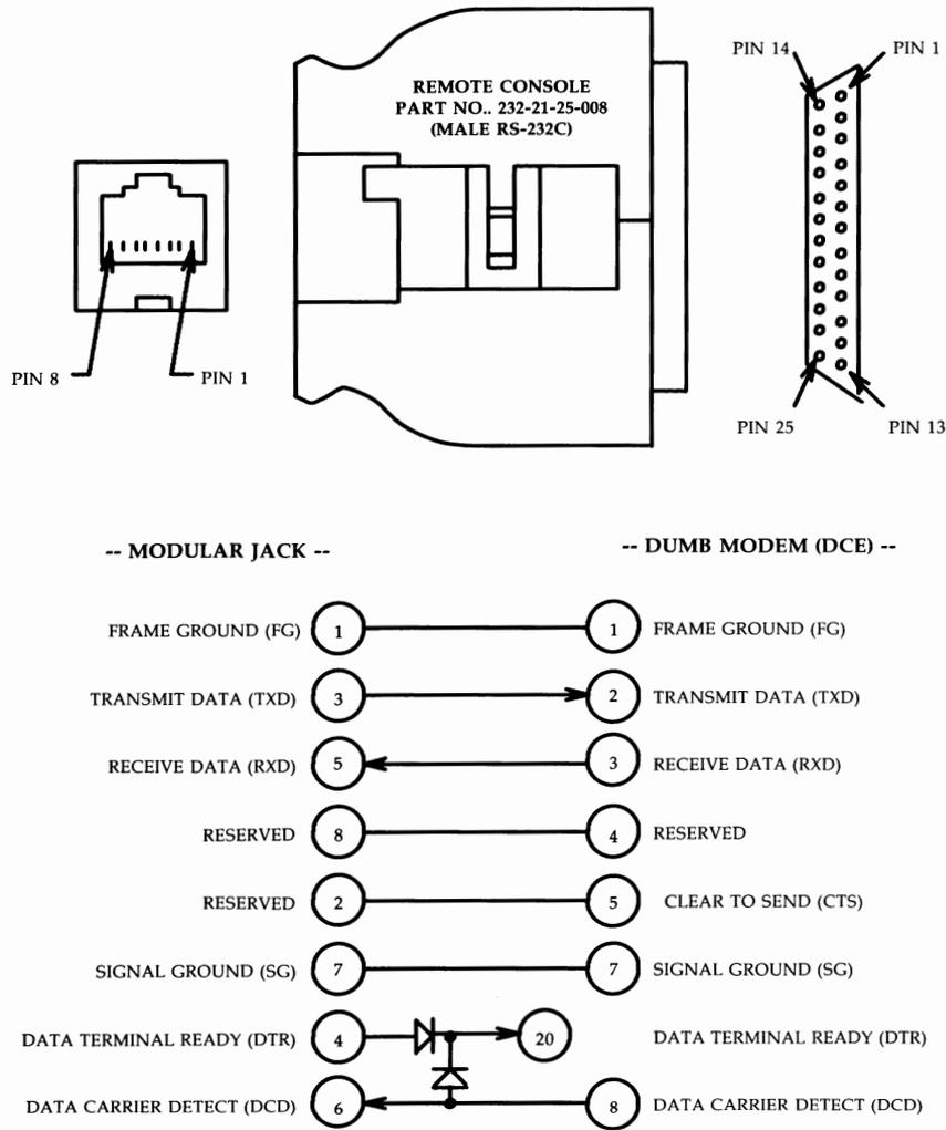
Figure B-40: Remote Console Male Connector (232-21-25-008) Pin Identification
