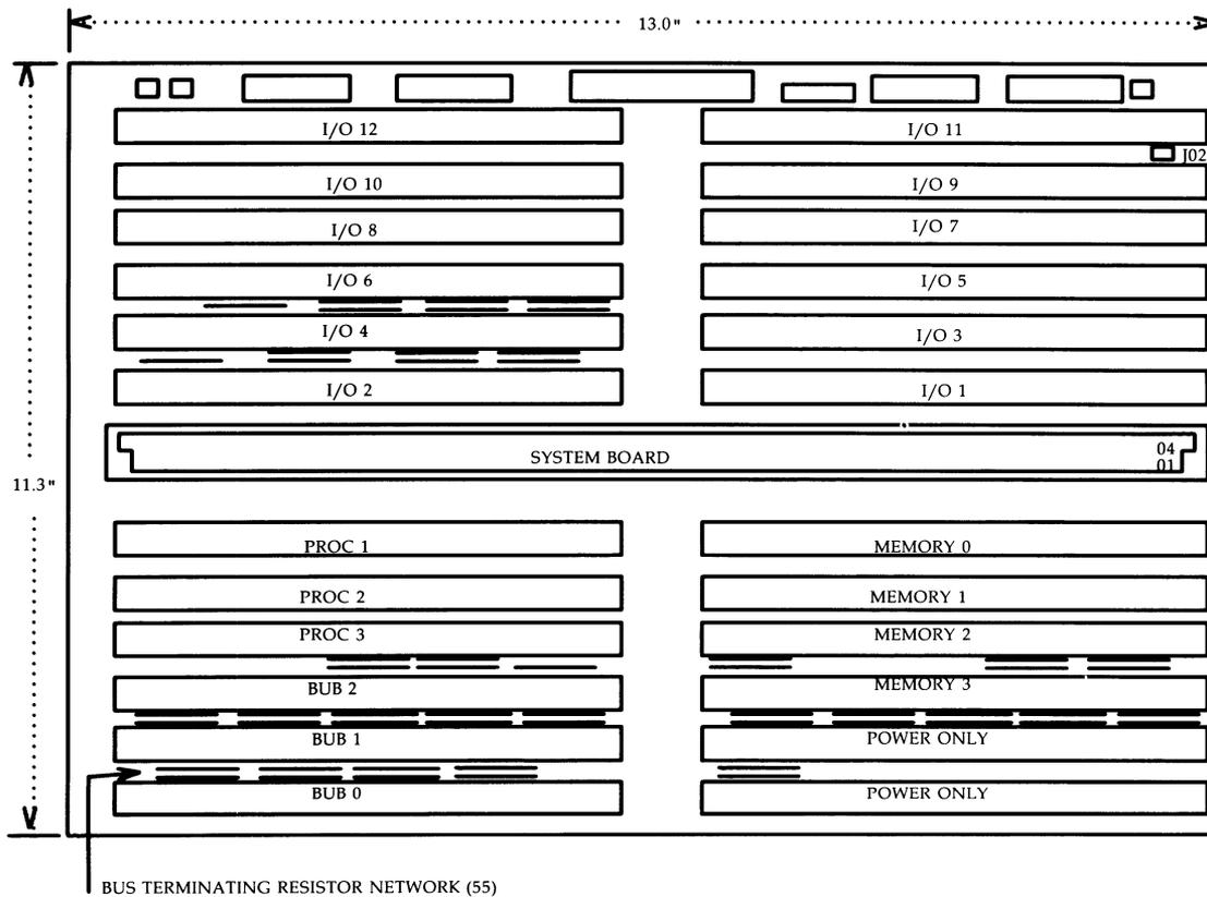
Figure 2-40: CM519B Backplane Board Layout
