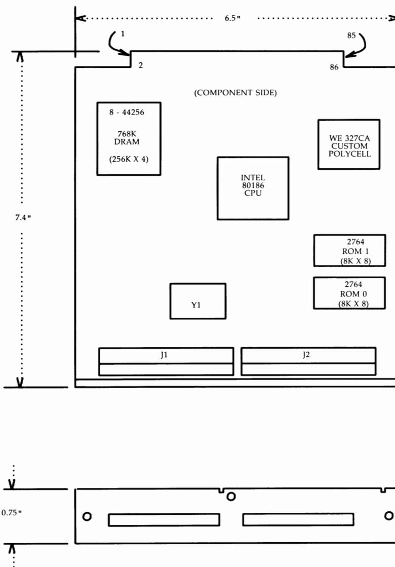
Figure 2-47: CM195AE GPSC Card Layout
