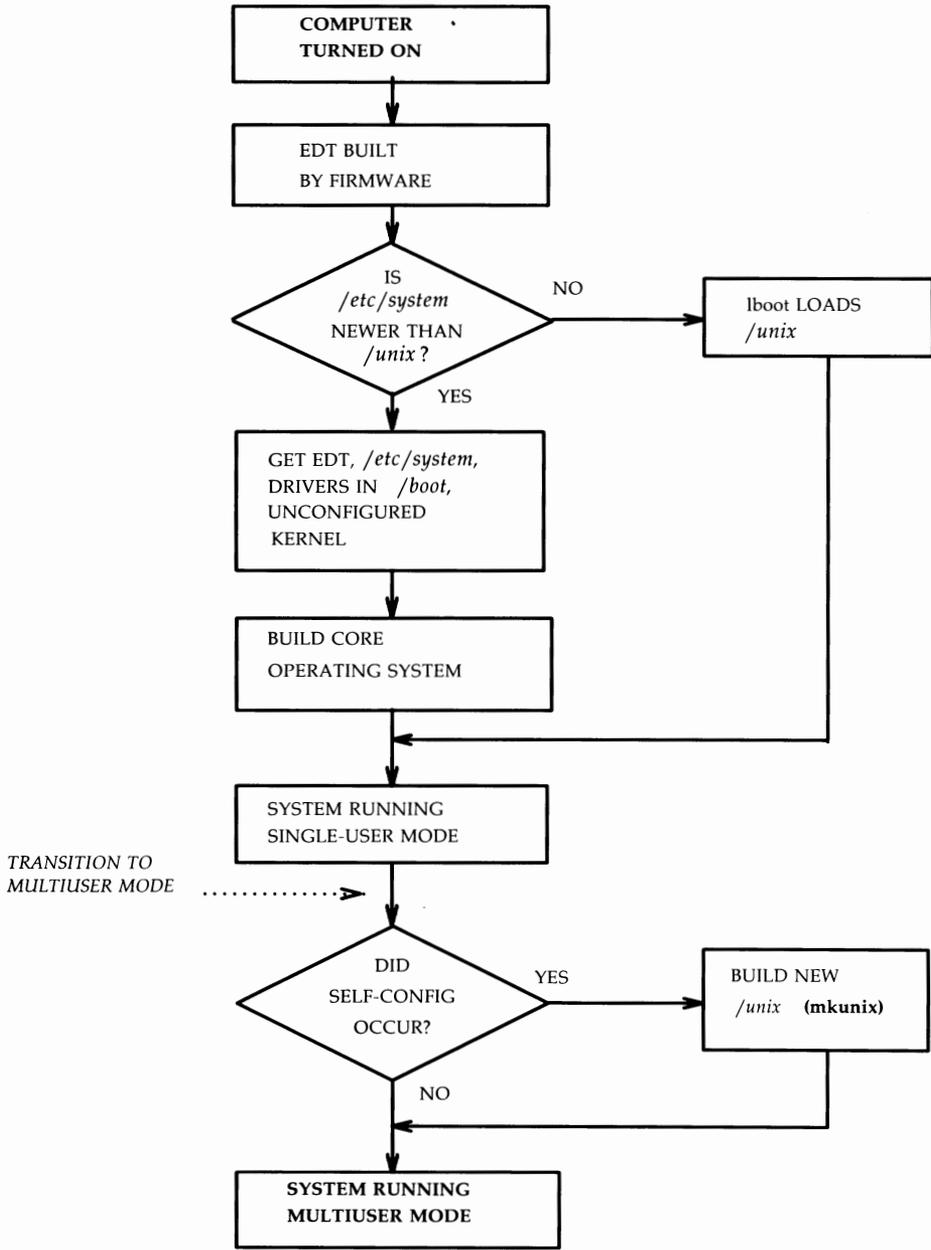
Figure 3-10: Self-Configuration — Powerup Sequence
