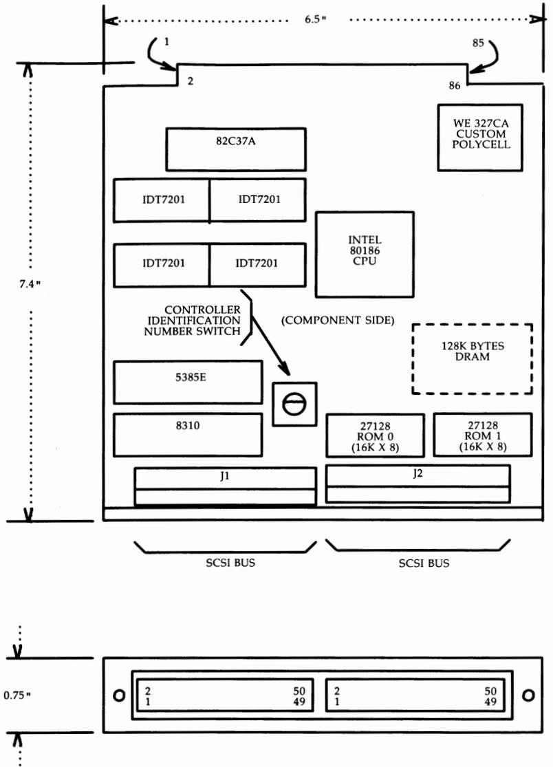
Figure B-30: CM195W SCSI Host Adapter Card Layout
