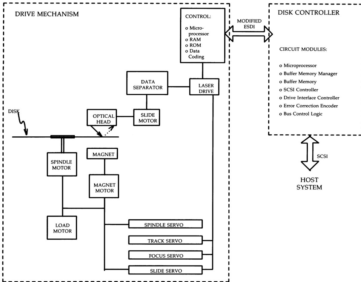
Figure 3-95: SCSI Rewritable Optical Disk Drive — Functional Block Diagram
