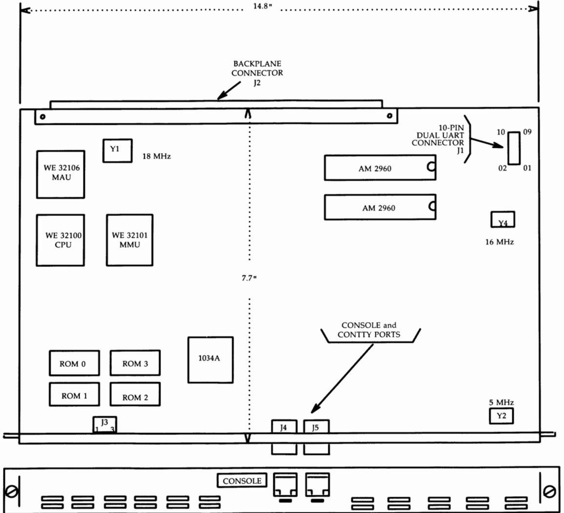
Figure 2-25: CM518A System Board Layout
