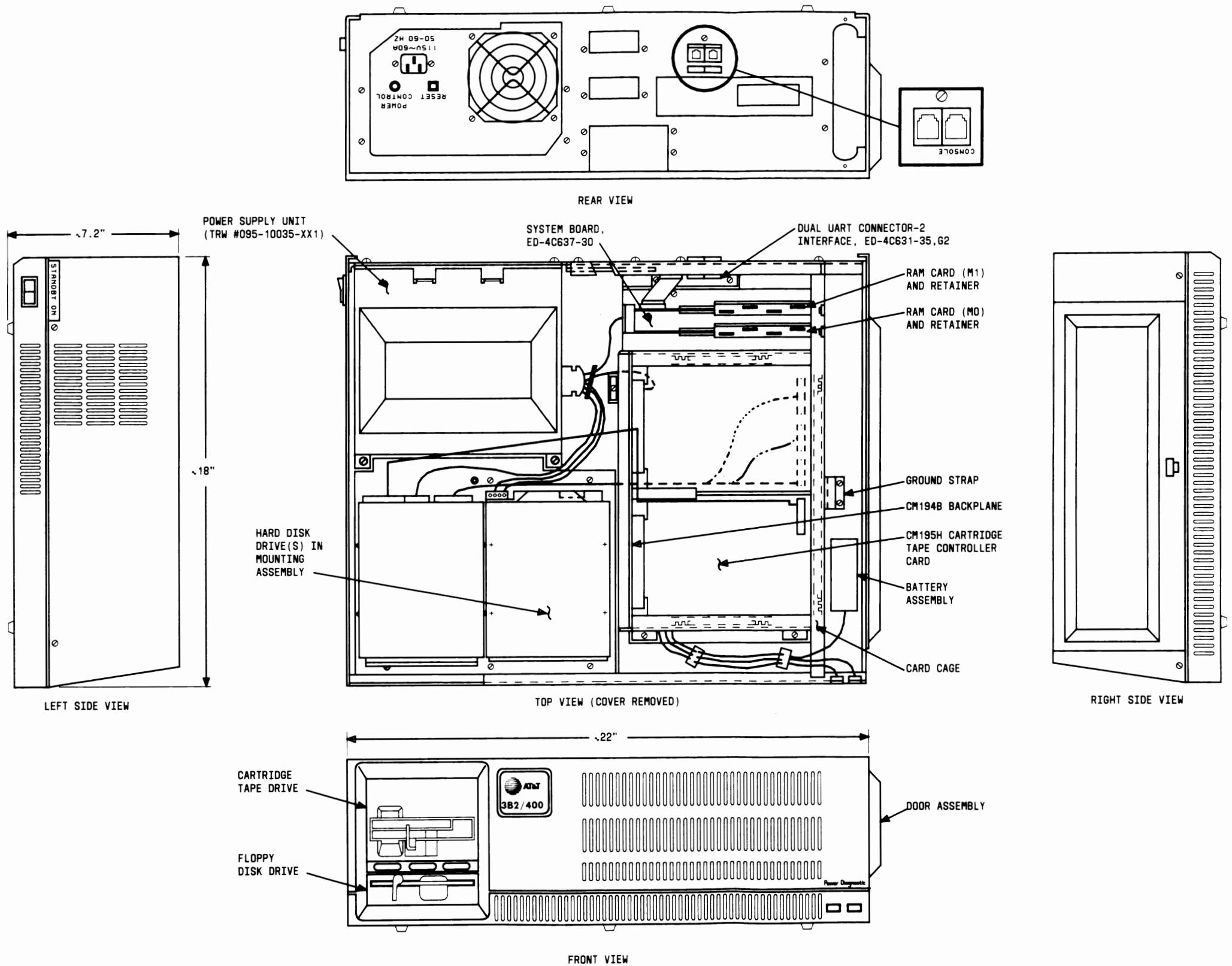
Figure 2-5: Domestic 3B2/400 Computer Cabinet Assembly Drawing (ED-4C631-30)
