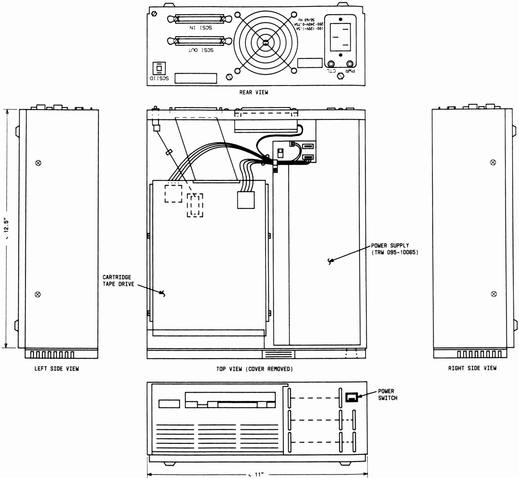
Figure 2-21: AT&T SCSI TM Cabinet Assembly
