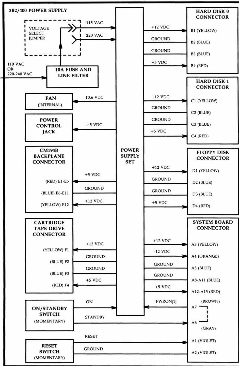
Figure 3-99: 3B2/400 Computer Power Supply — Functional Block Diagram
