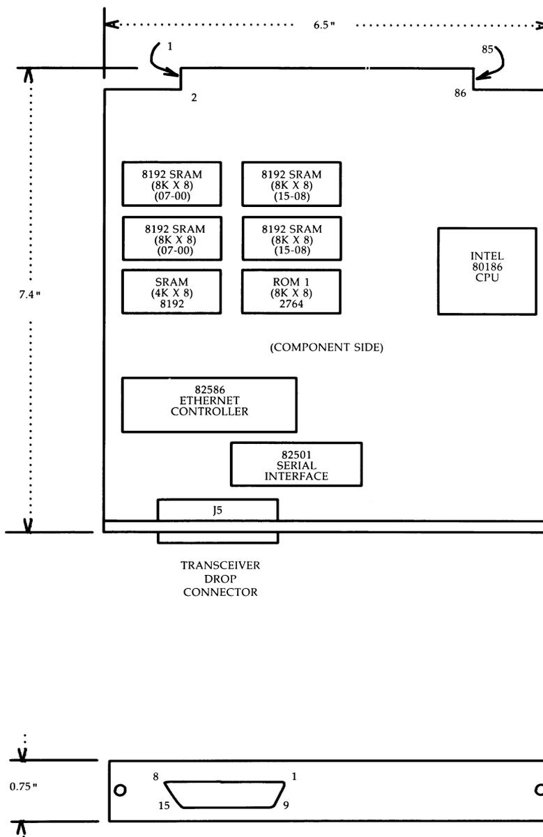
Figure 2-44: CM195A NI Card Layout
