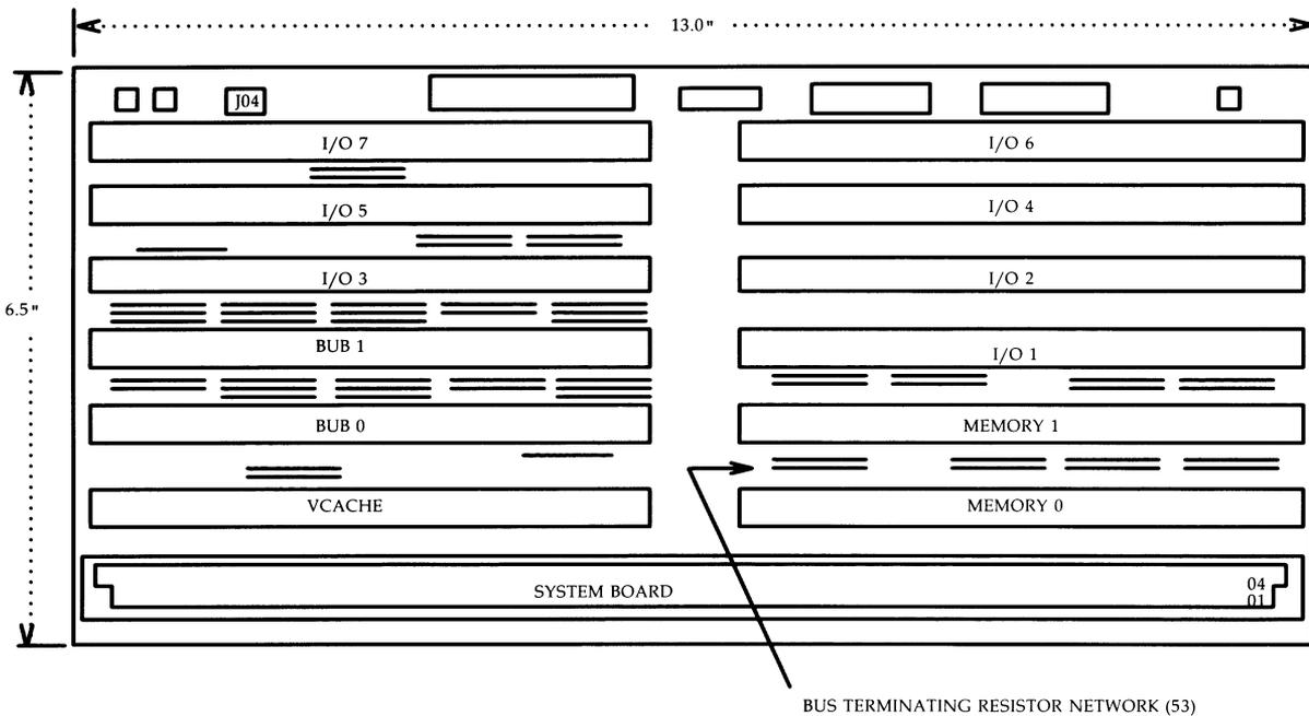
Figure 2-41: CM520A Backplane Board Layout
