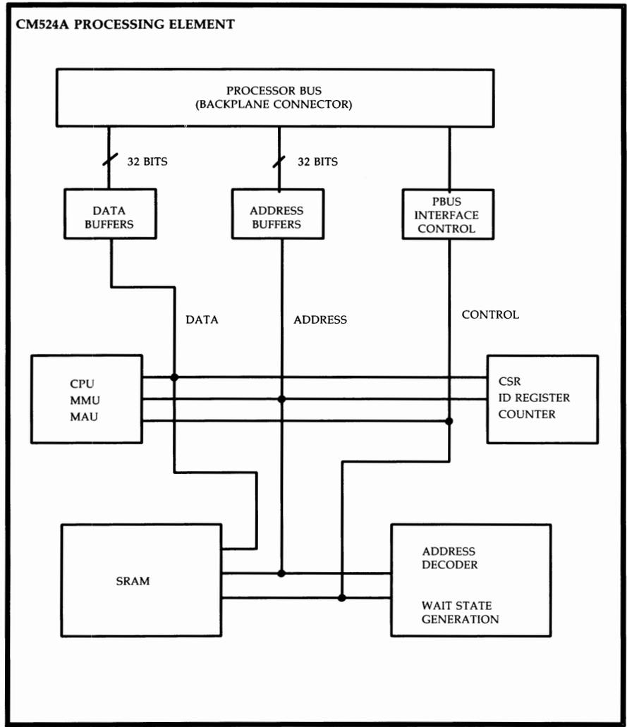
Figure 3-81: CM524A PE Card — Functional Block Diagram
