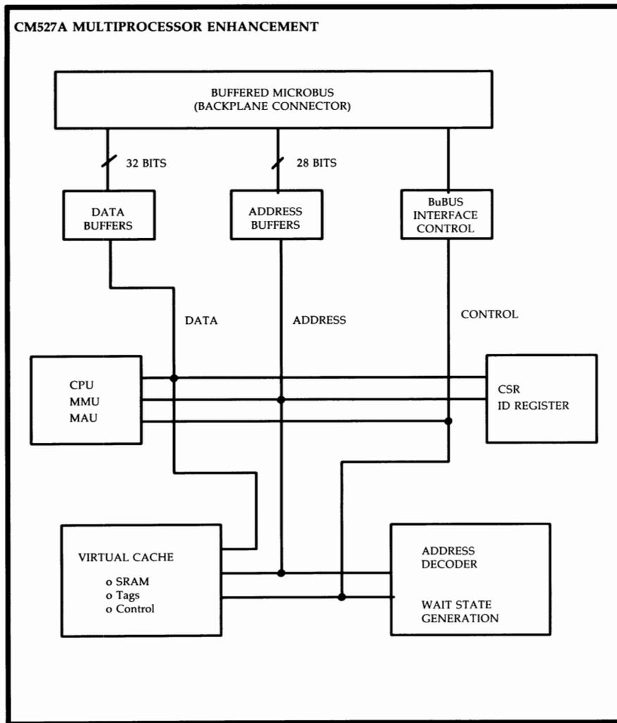
Figure 3-85: CM527A MPE Card — Functional Block Diagram
