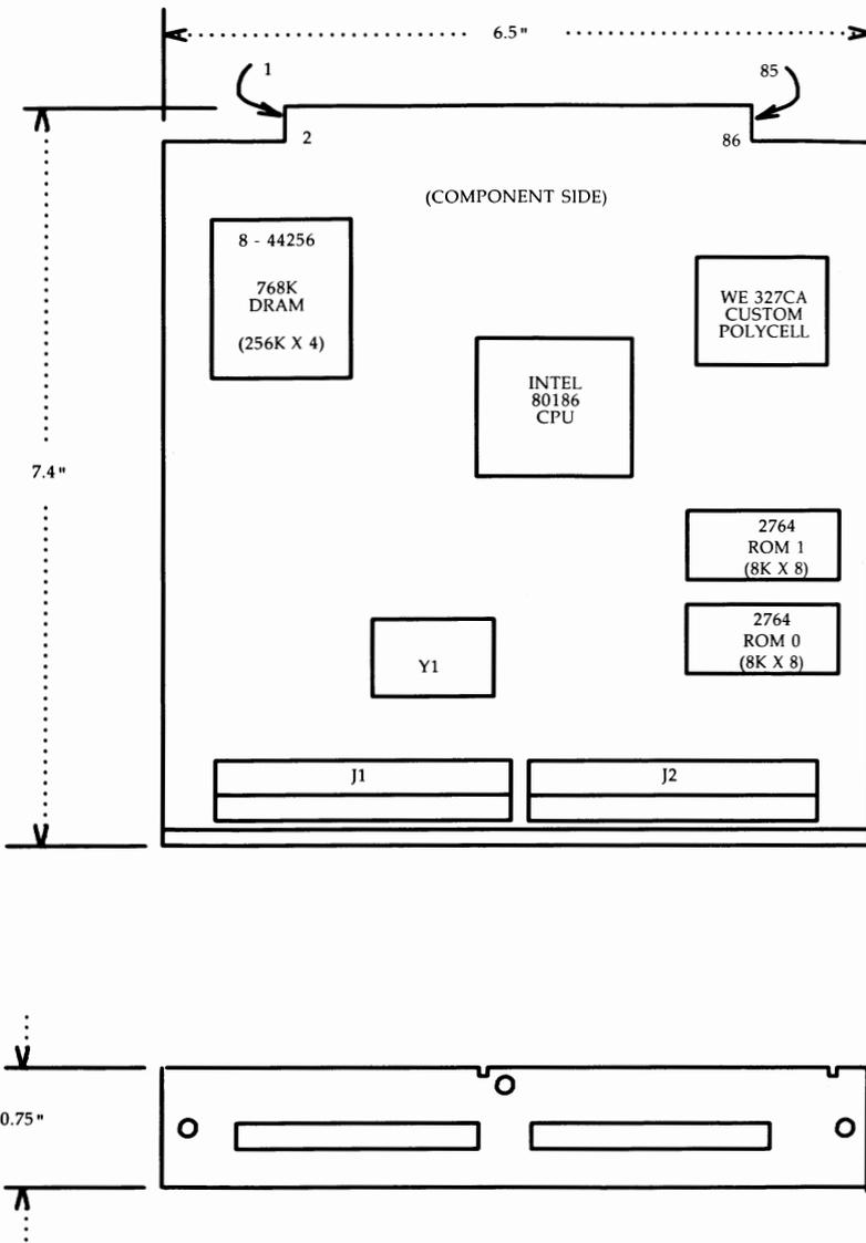
Figure B-23: CM195AE GPSC Card Layout
