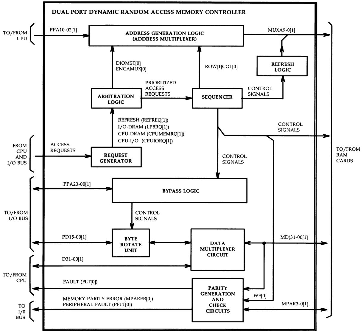
Figure 3-24: Dual Port Dynamic Random Access Memory Controller — Functional Block Diagram
