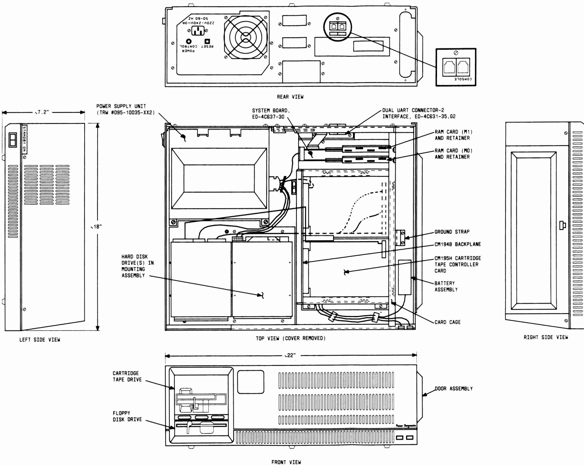
Figure 2-6: International 3B2/400 Computer Cabinet Assembly Drawing (ED-4C638-30)
