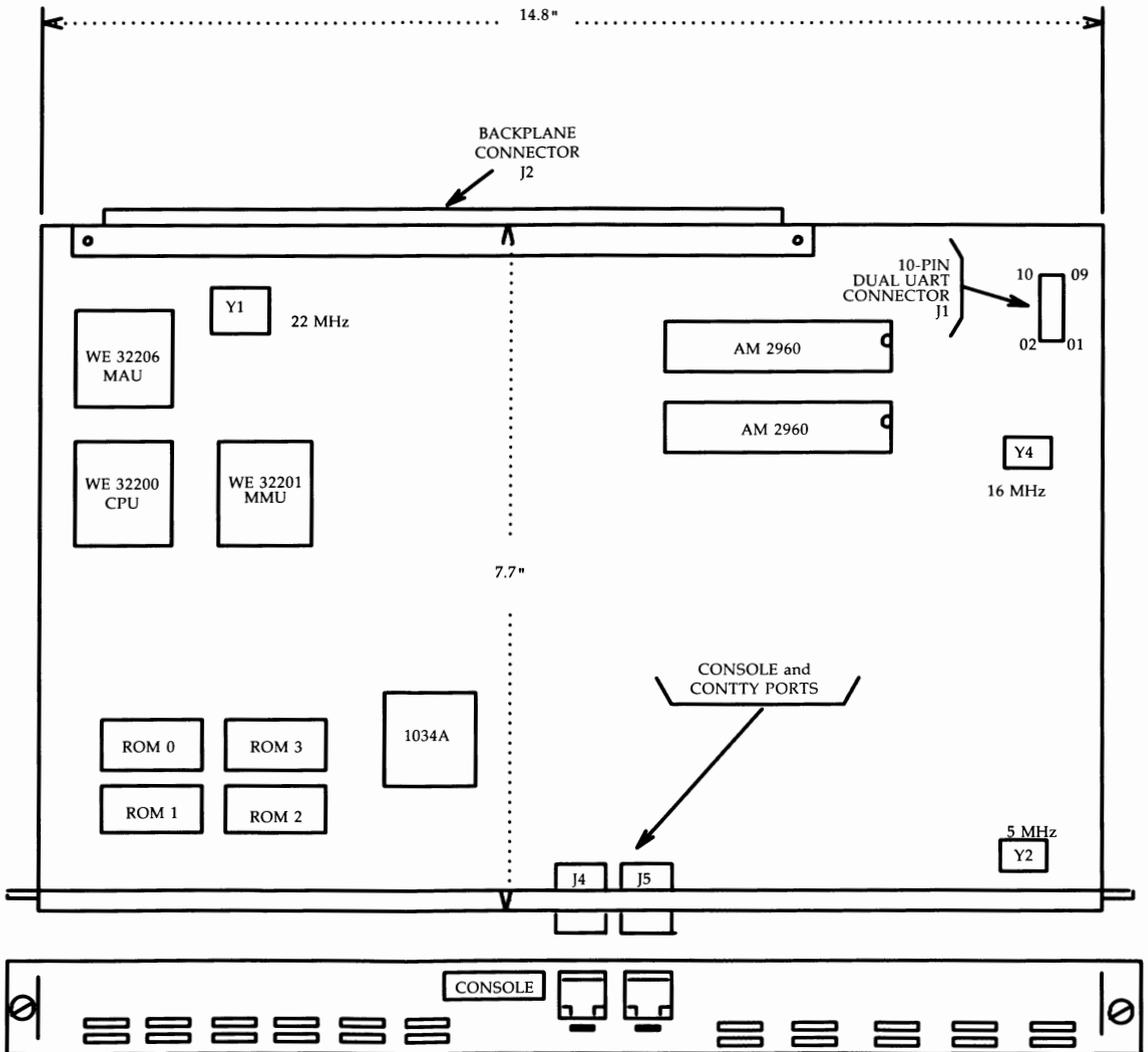
Figure 2-26: CM518B System Board Layout
