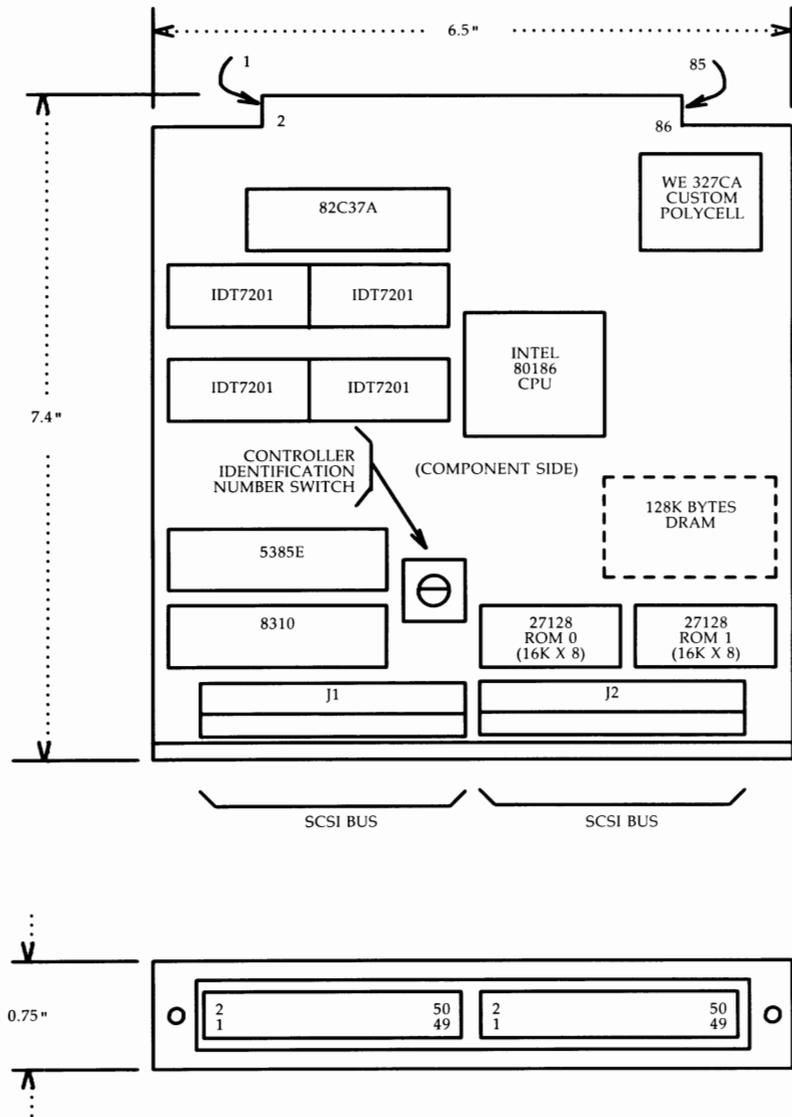
Figure 2-56: CM195W SCSI Host Adapter Card Layout
