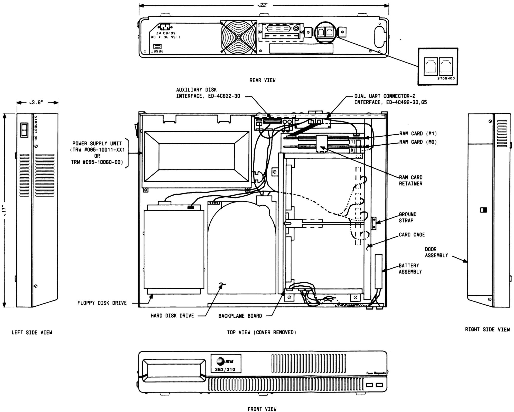
Figure 2-3: Domestic 3B2/310 Computer Cabinet Assembly Drawing (ED-4C645-30)
