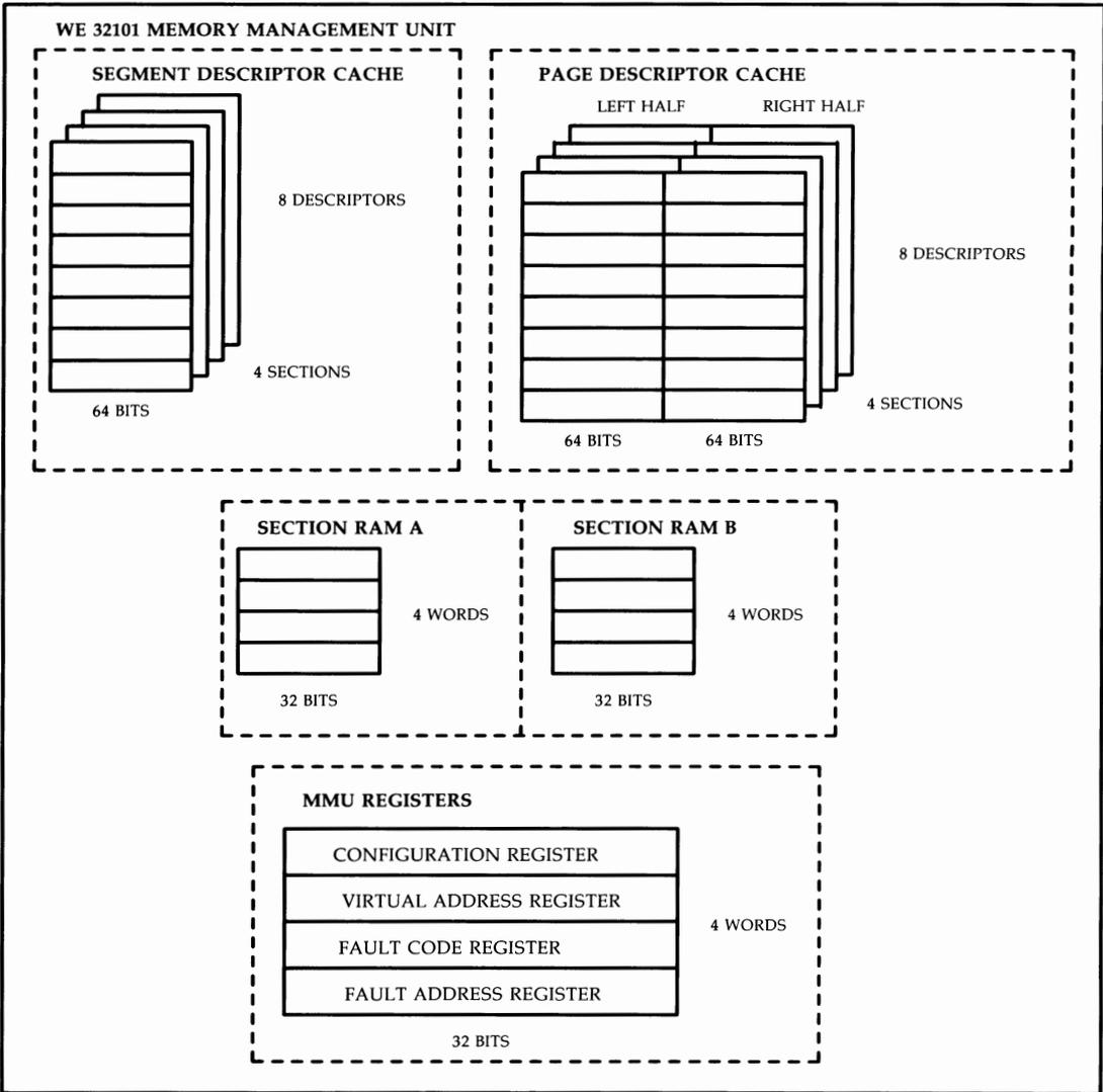
Figure 3-16: WE 32101 MMU Block Diagram
