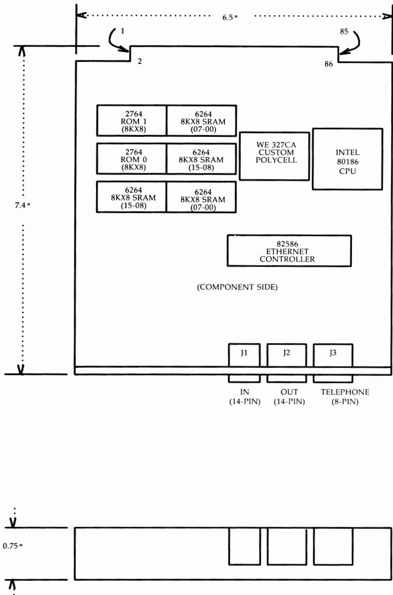
Figure 2-55: CM195U STARLAN Interface Card Layout
