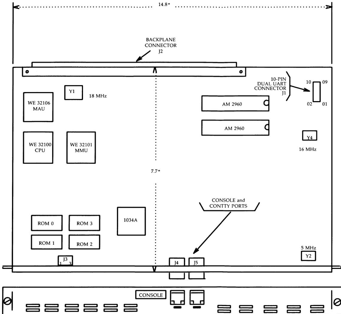
Figure B-3: CM518A System Board Layout
