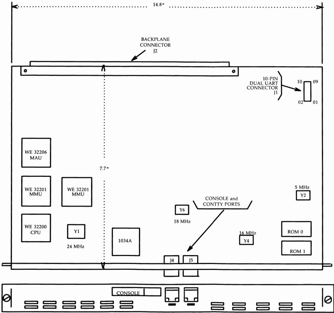
Figure 2-27: CM518C System Board Layout
