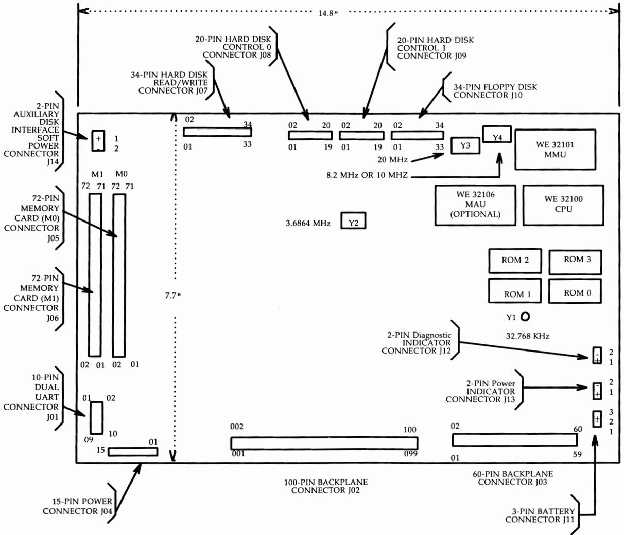
Figure 2-24: System Board, ED-4C637-30 Layout
