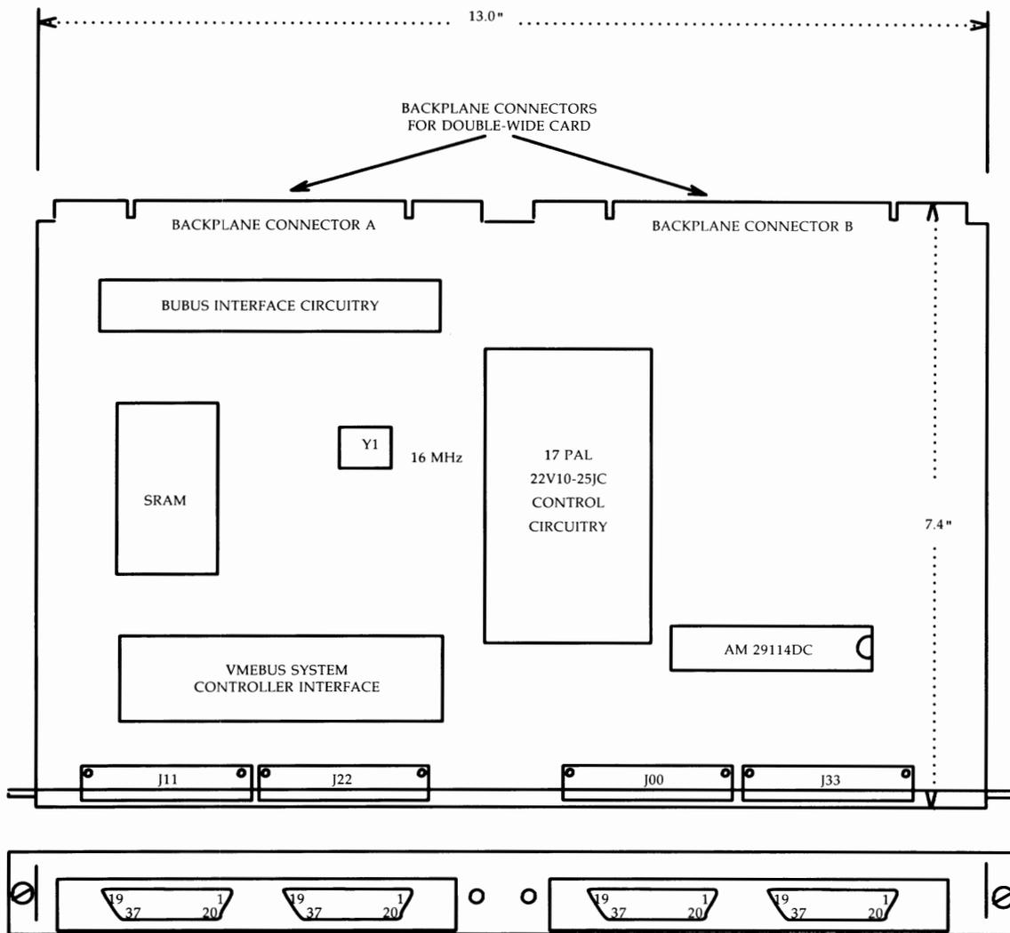
Figure 2-61: CM525B VMEbus Card Layout
