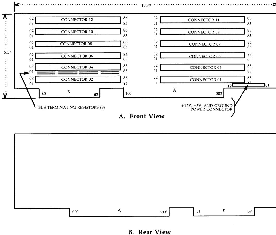
Figure 2-38: CM194B Backplane Board Layout
