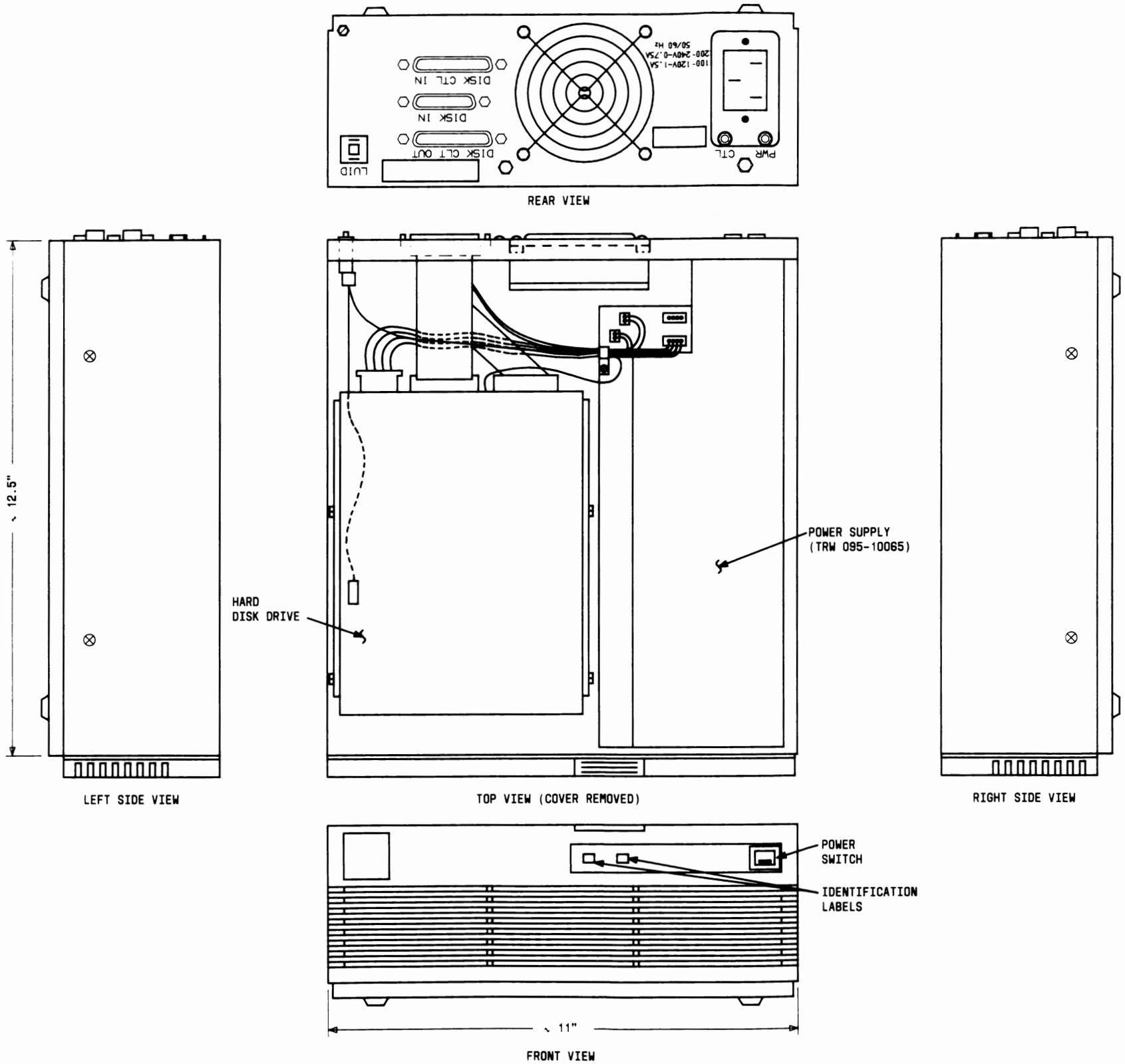
Figure 2-16: AT&T DM Cabinet Assembly Drawing (ED-3T011-30,G2,G3,G5,G6)
