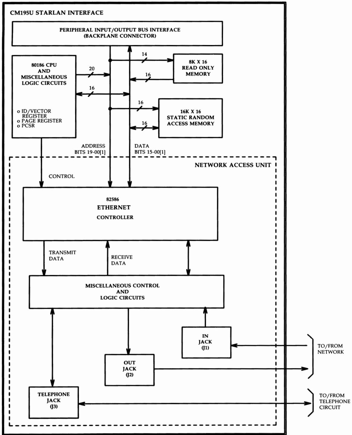
Figure 3-71: CM195U STARLAN Interface Card — Functional Block Diagram
