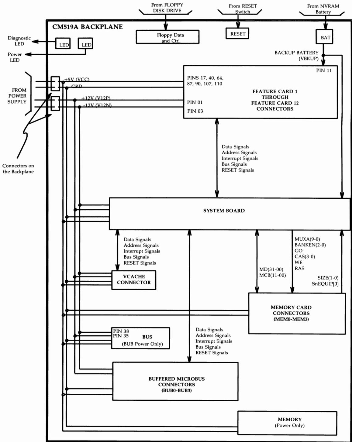
Figure 3-50: CM519A (3B2/600 and 700) Backplane — Functional Block Diagram
