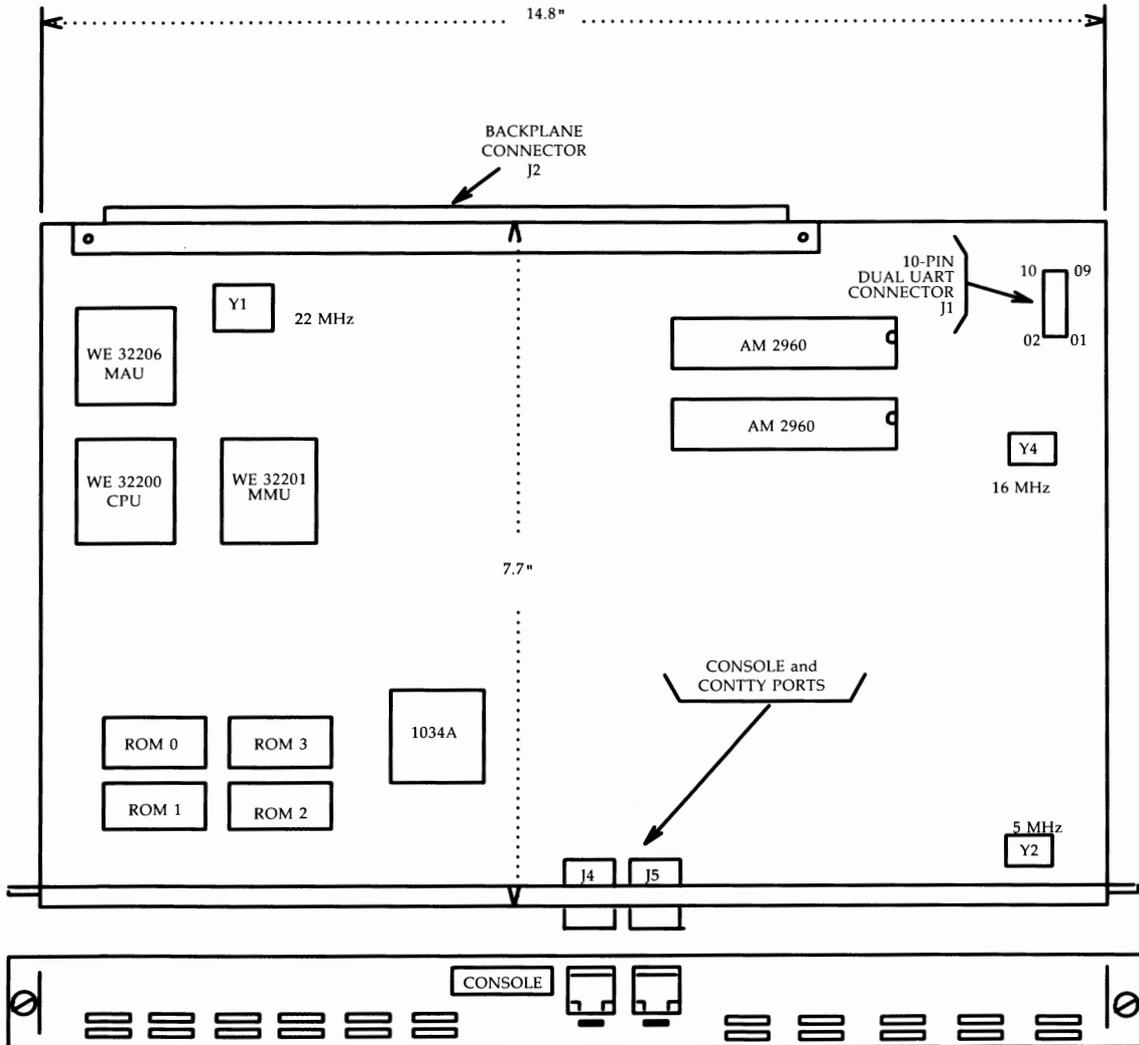
Figure B-4: CM518B System Board Layout
