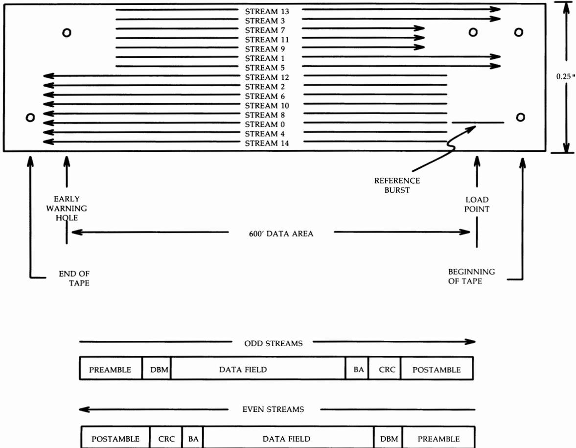
Figure 3-93: 120-Megabyte Cartridge Tape Physical Layout
