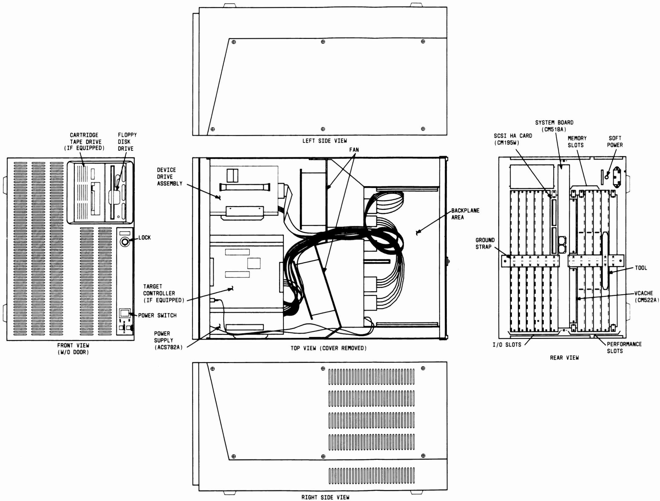
Figure 2-8: 3B2/600 Computer Cabinet Assembly Drawing (ED-3T023-30)
