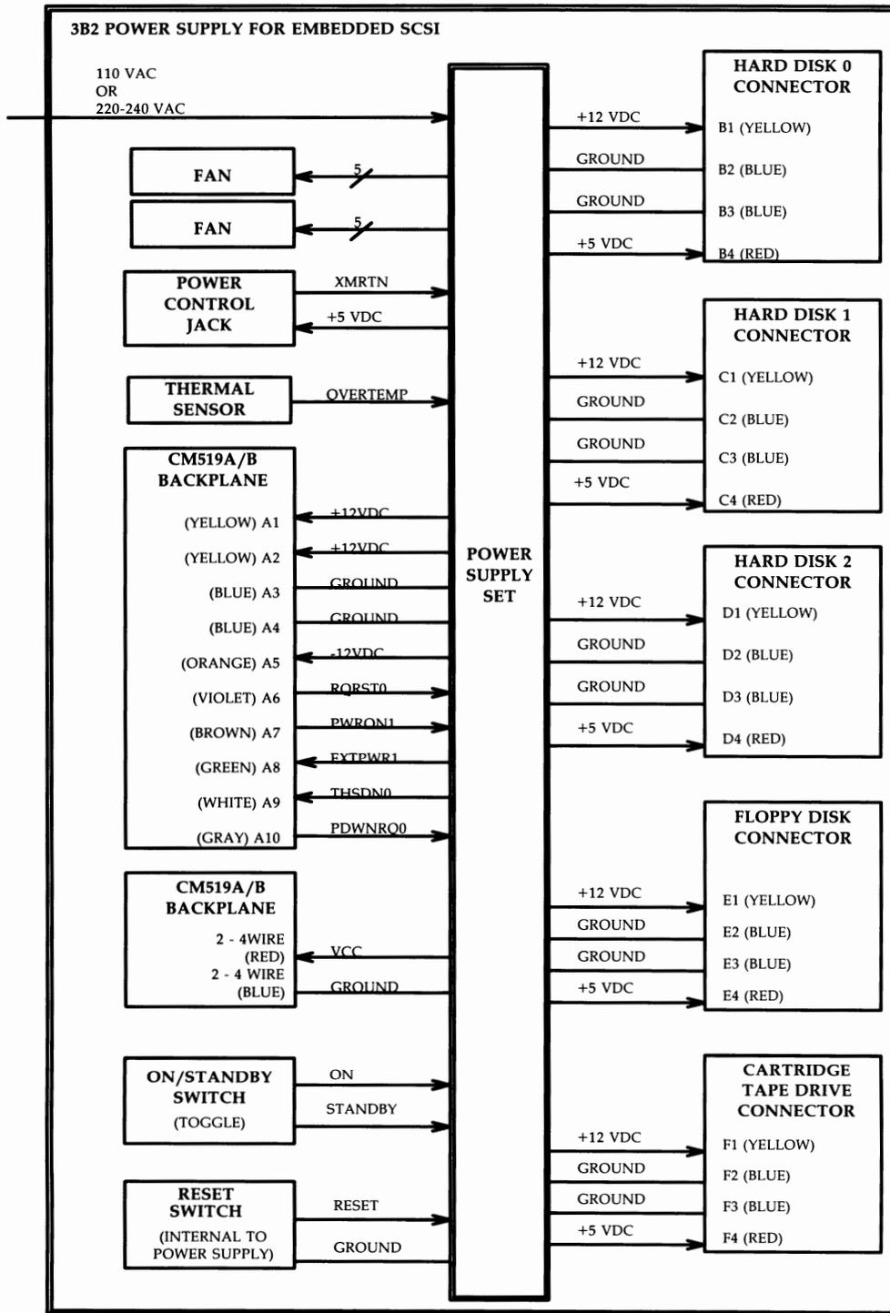
Figure 3-102: 3B2 Power Supply for Embedded SCSI— Functional Block Diagram
