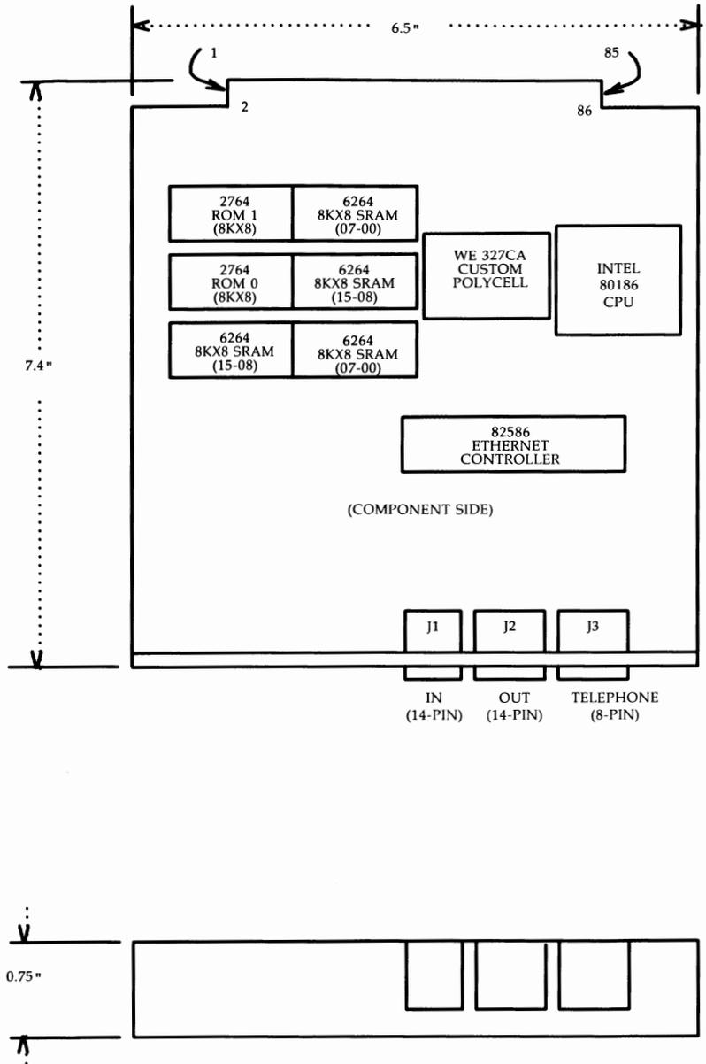
Figure B-29: CM195U STARLAN Interface Card Layout
