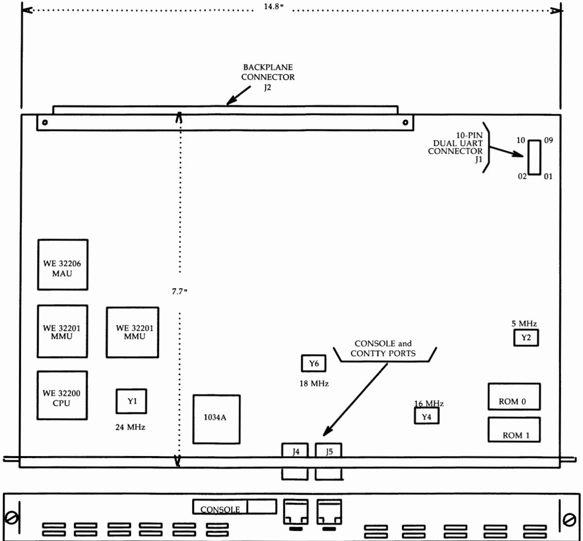
Figure 2-27: CM518C System Board Layout
