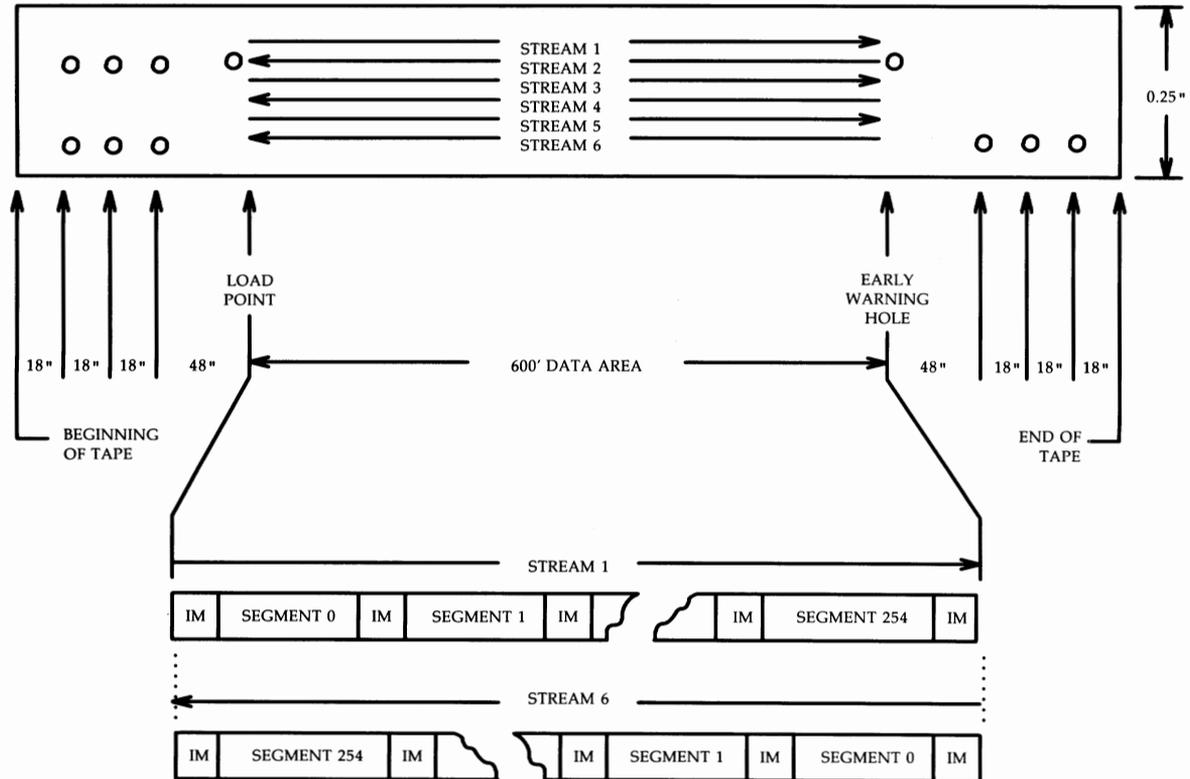
Figure 3-89: Cartridge Tape Physical Layout
