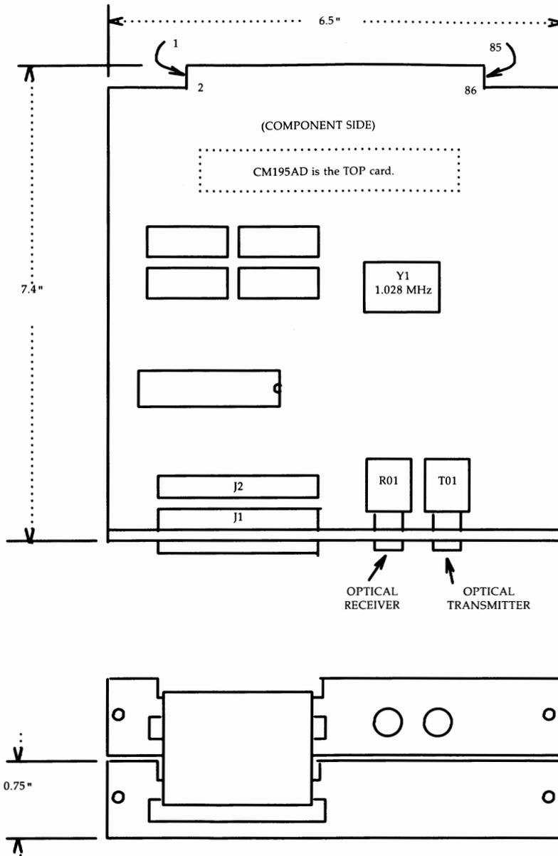
Figure B-22: CM195A/CM195AD Datakit VCS Interface Card Layout
