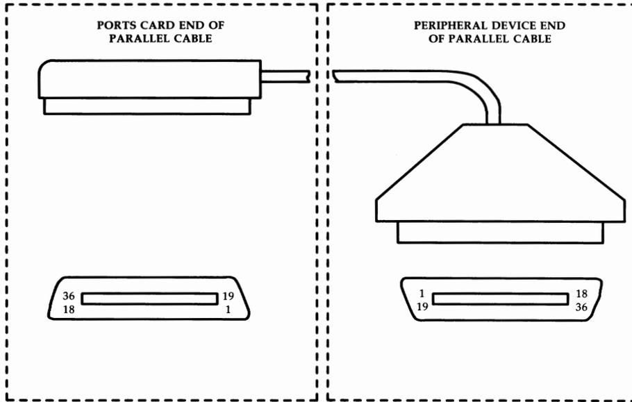
Figure B-43: CENTRONICS Connectorized Cable Pin Identification
