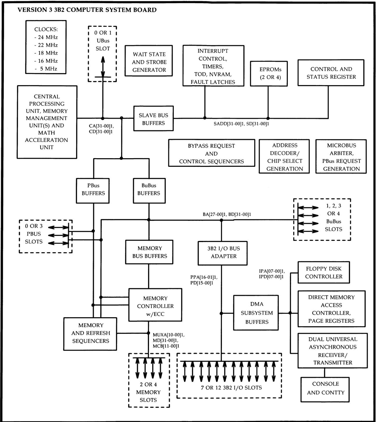
Figure 3-27: Version 3 3B2 Computer System Board — Functional Block Diagram
