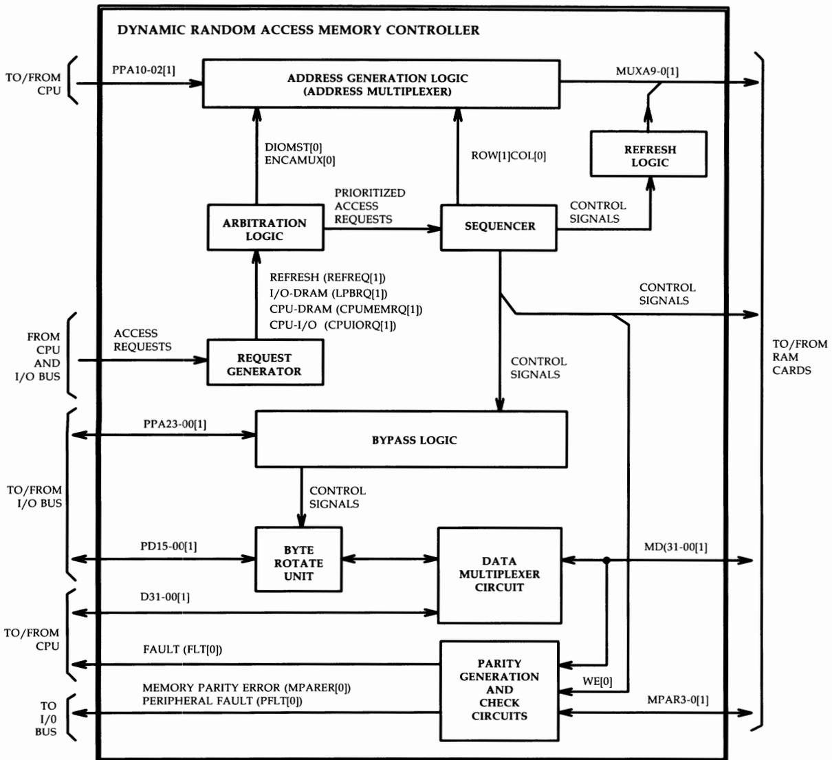
Figure 3-36: Dynamic Random Access Memory Controller — Functional Block Diagram
