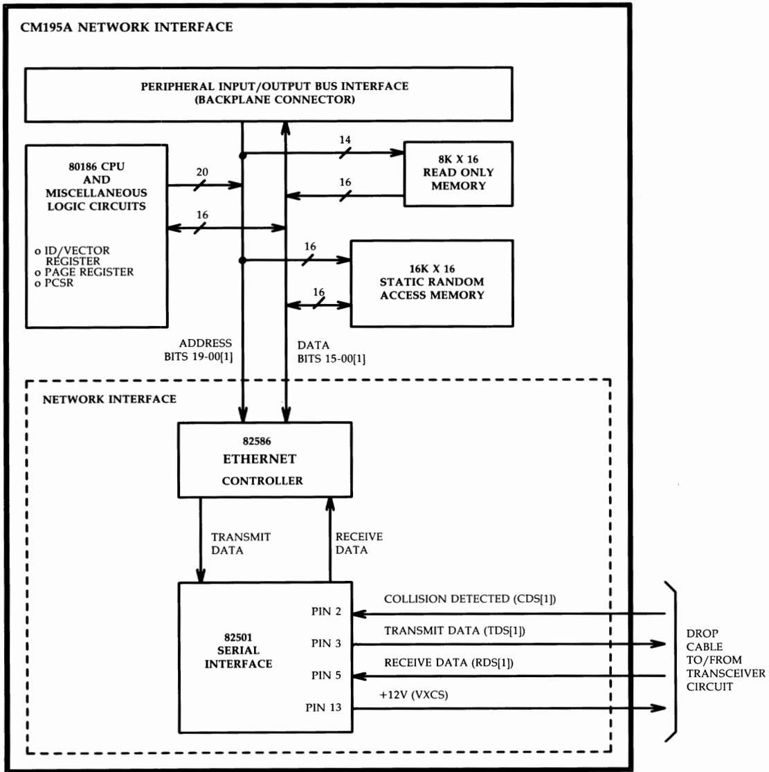
Figure 3-53: CM195A NI Card — Functional Block Diagram
