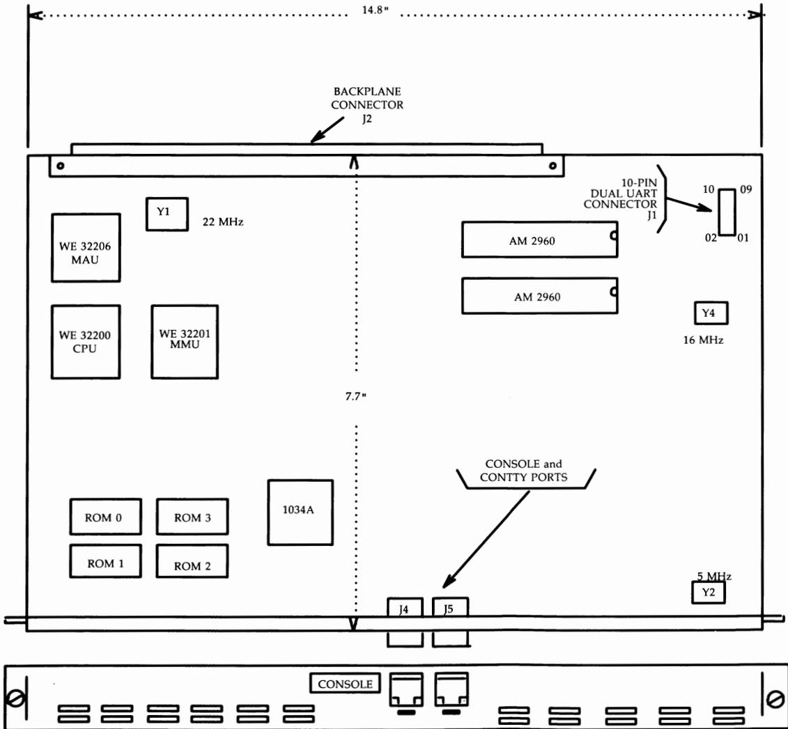
Figure 2-26: CM518B System Board Layout
