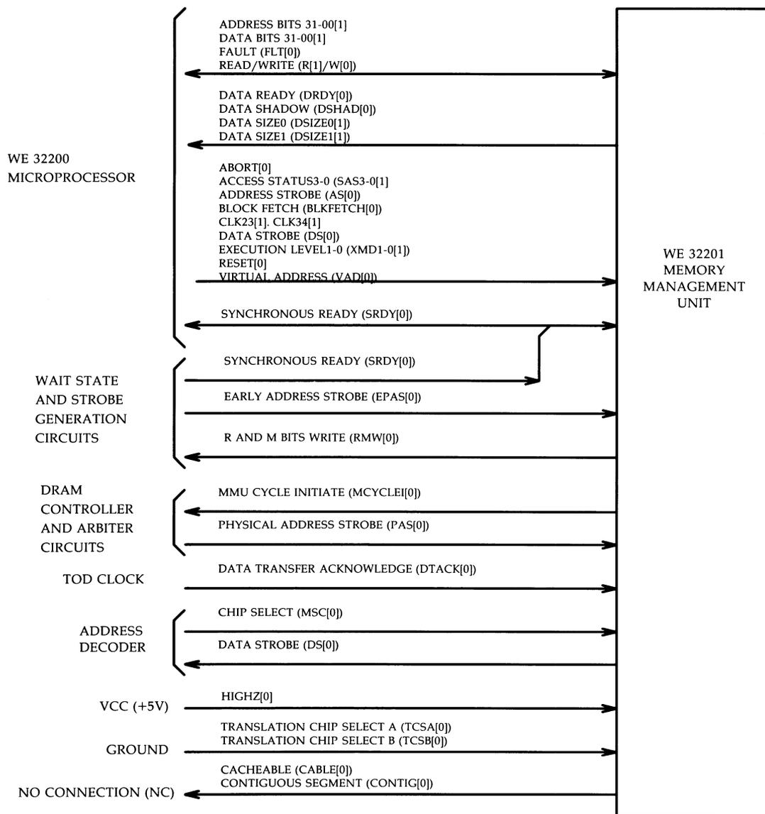
Figure 3-29: WE 32201 MMU Interconnection Diagram
