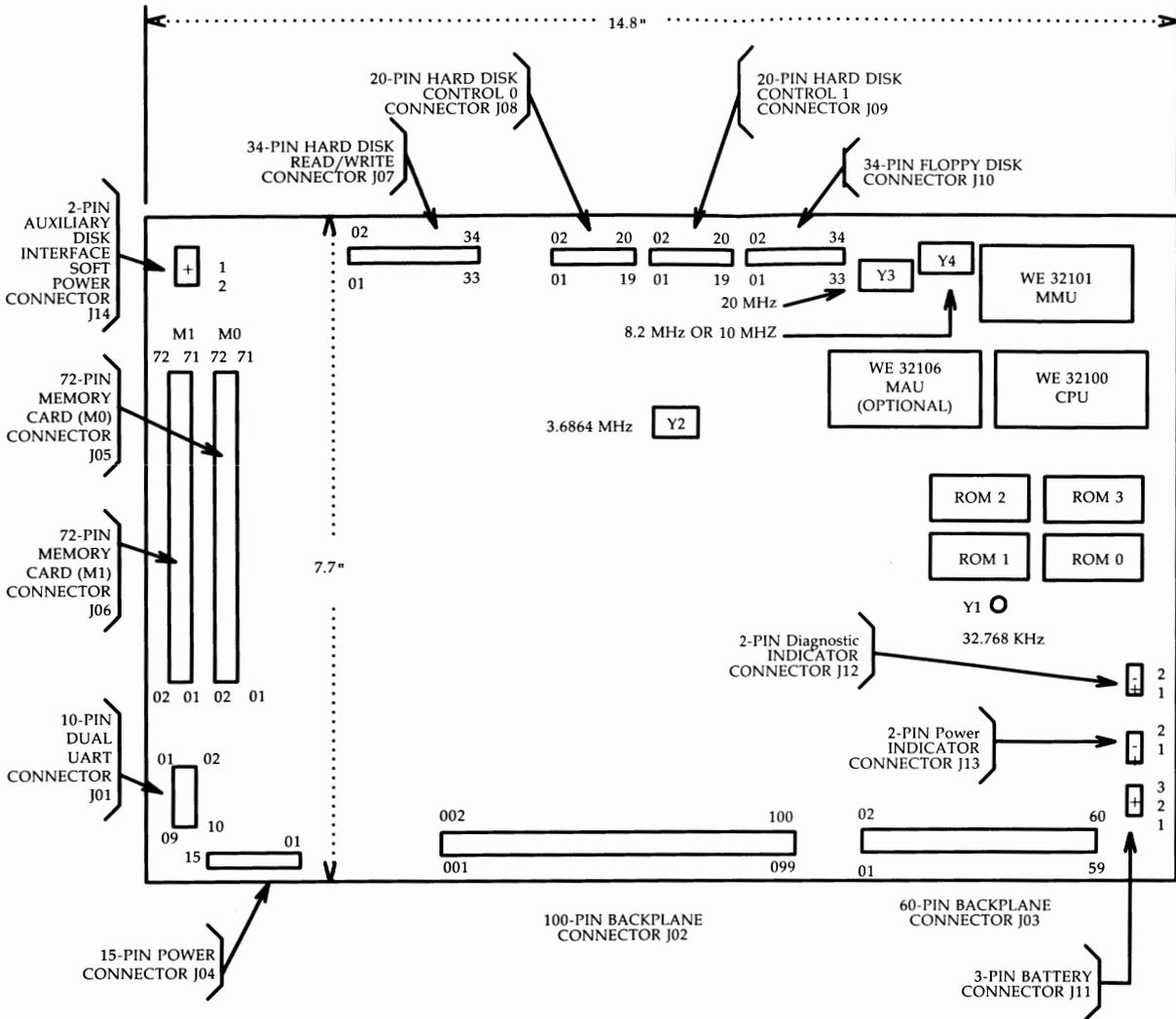
Figure B-2: System Board, ED-4C637-30 Layout
