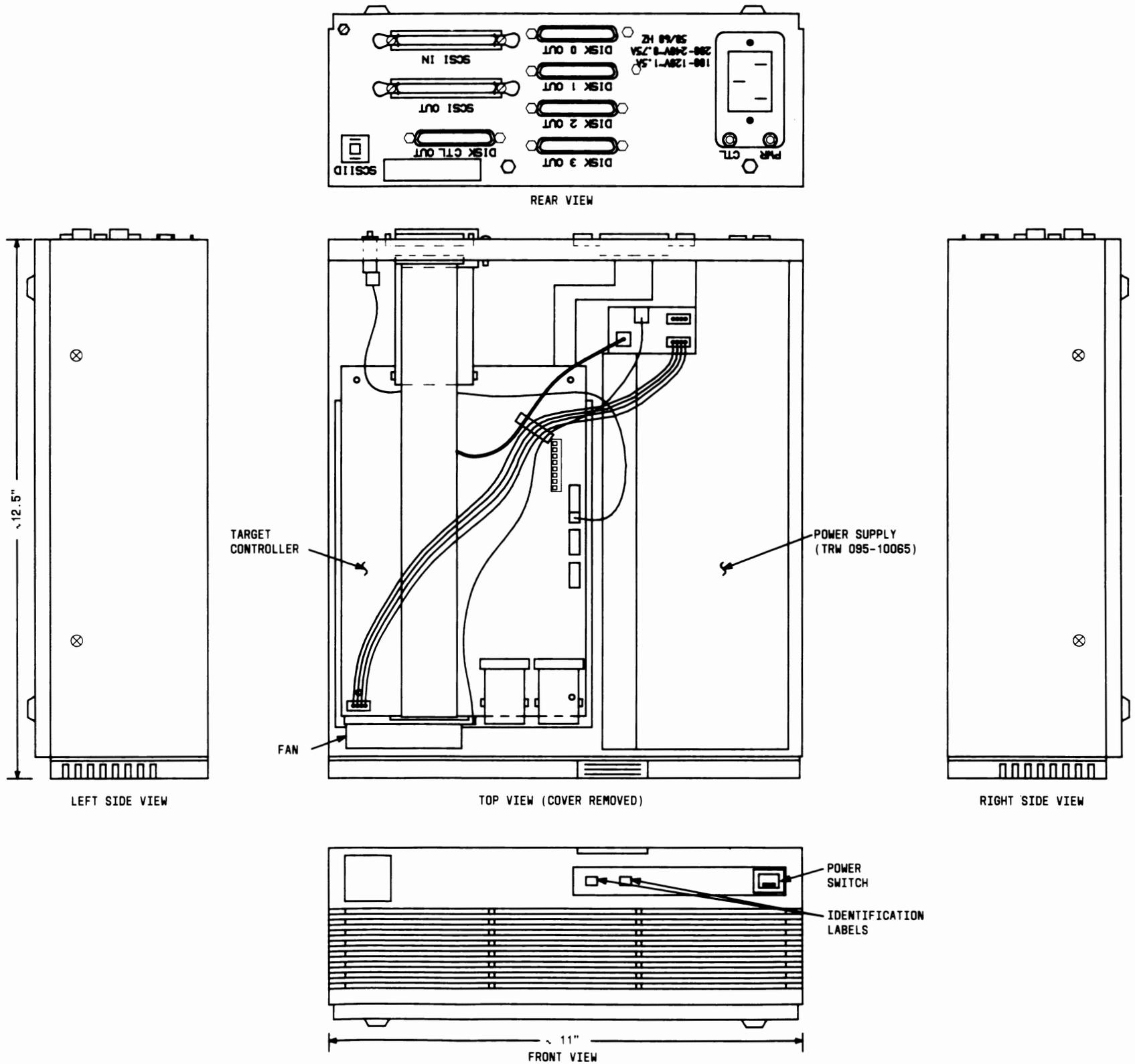
Figure 2-15: AT&T DCM/4E Cabinet Assembly Drawing (ED-3T011-30,G1)
