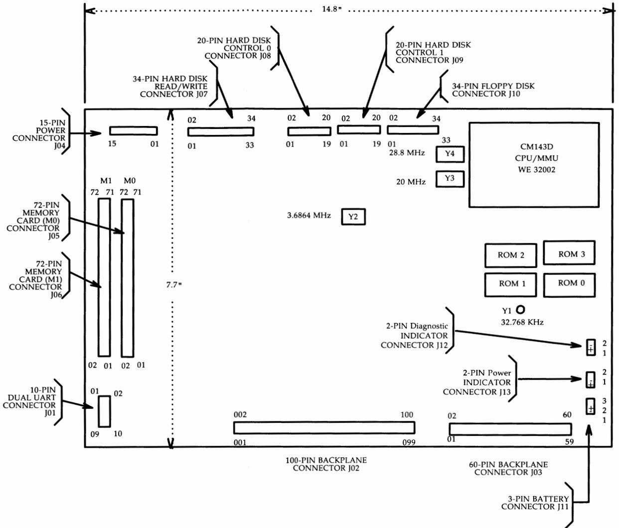
Figure B-1: CM190A System Board Layout
