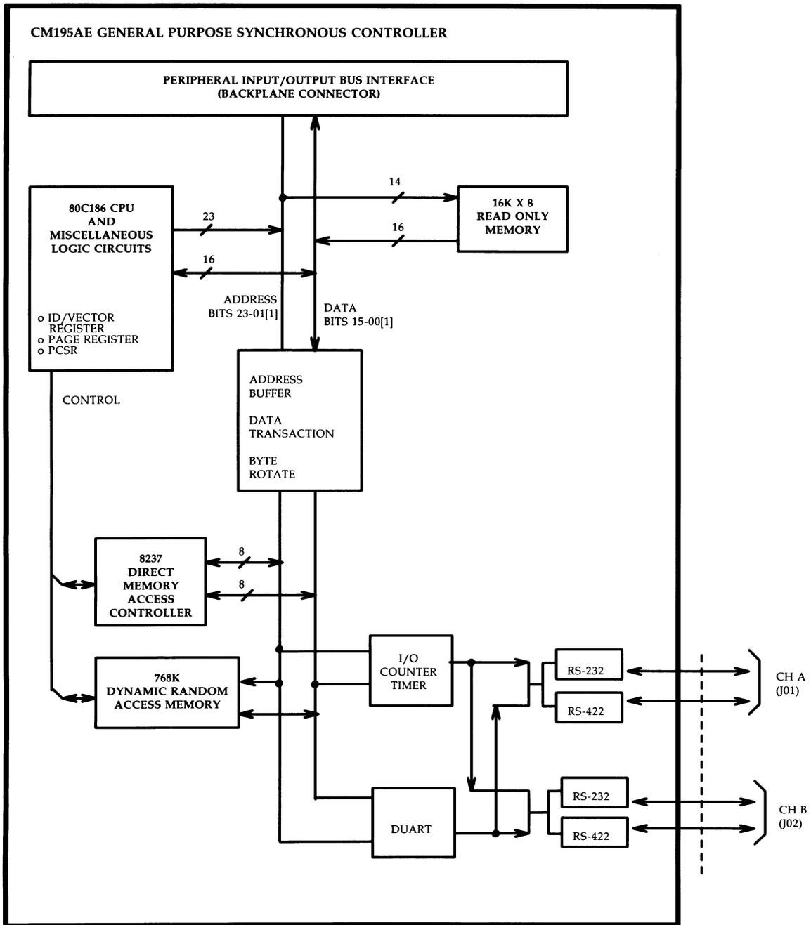
Figure 3-59: CM195AE GPSC Card—Functional Block Diagram
