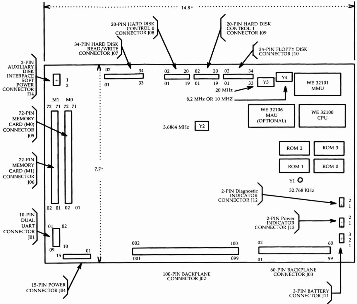
Figure B-2: System Board, ED-4C637-30 Layout
