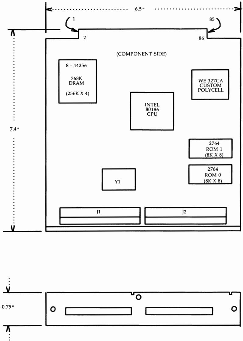
Figure B-23: CM195AE GPSC Card Layout
