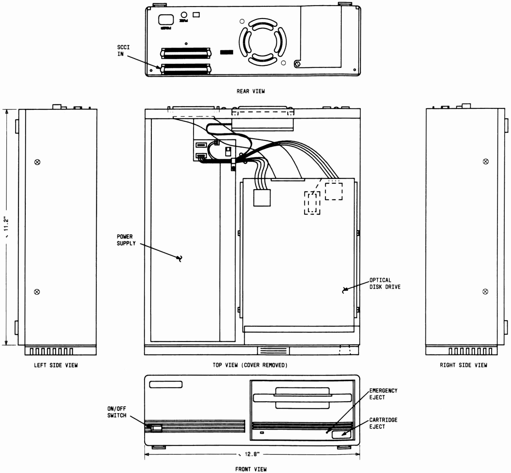
Figure 2-18: AT&T SCSI Rewritable Optical Disk Cabinet Assembly Drawing
