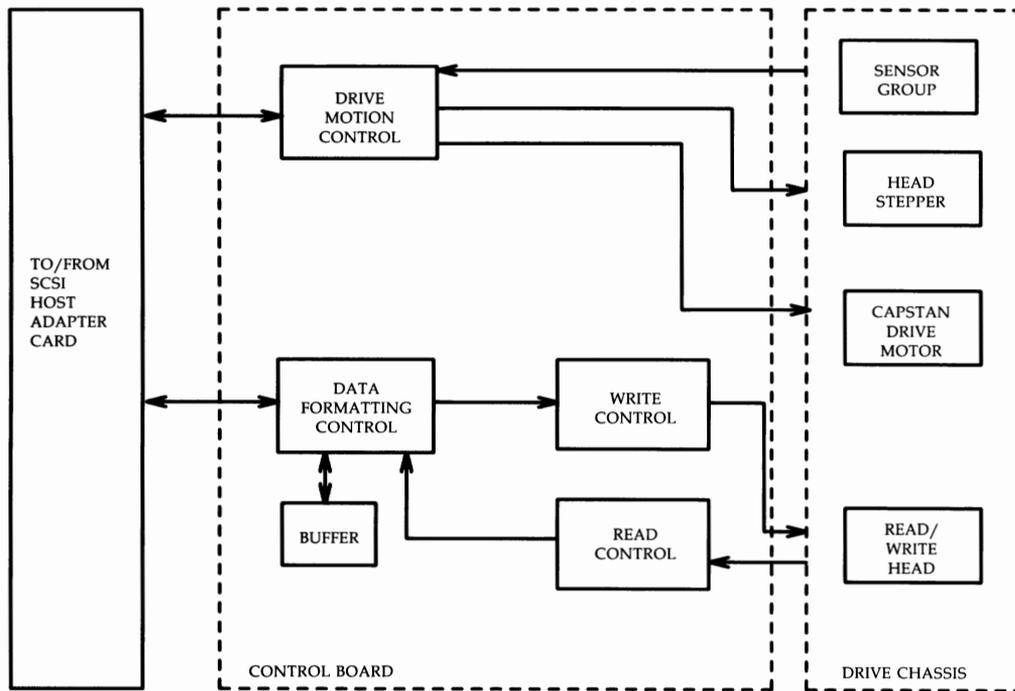
Figure 3-94: 120-Megabyte Cartridge Tape Drive — Functional Block Diagram
