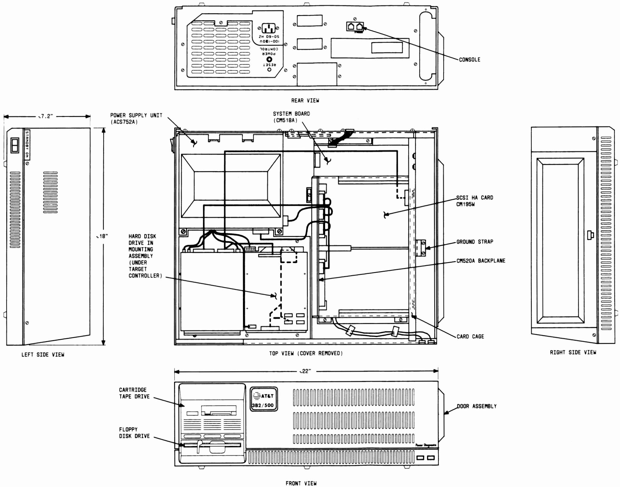
Figure 2-7: 3B2/500 Computer Cabinet Assembly Drawing (ED-3T043-30)
