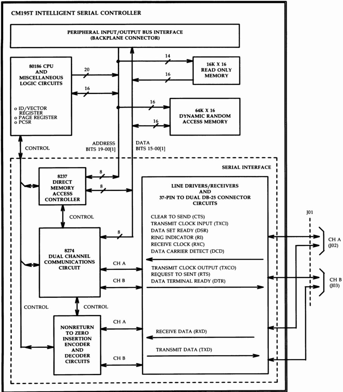
Figure 3-69: CM195T ISC Card — Functional Block Diagram
