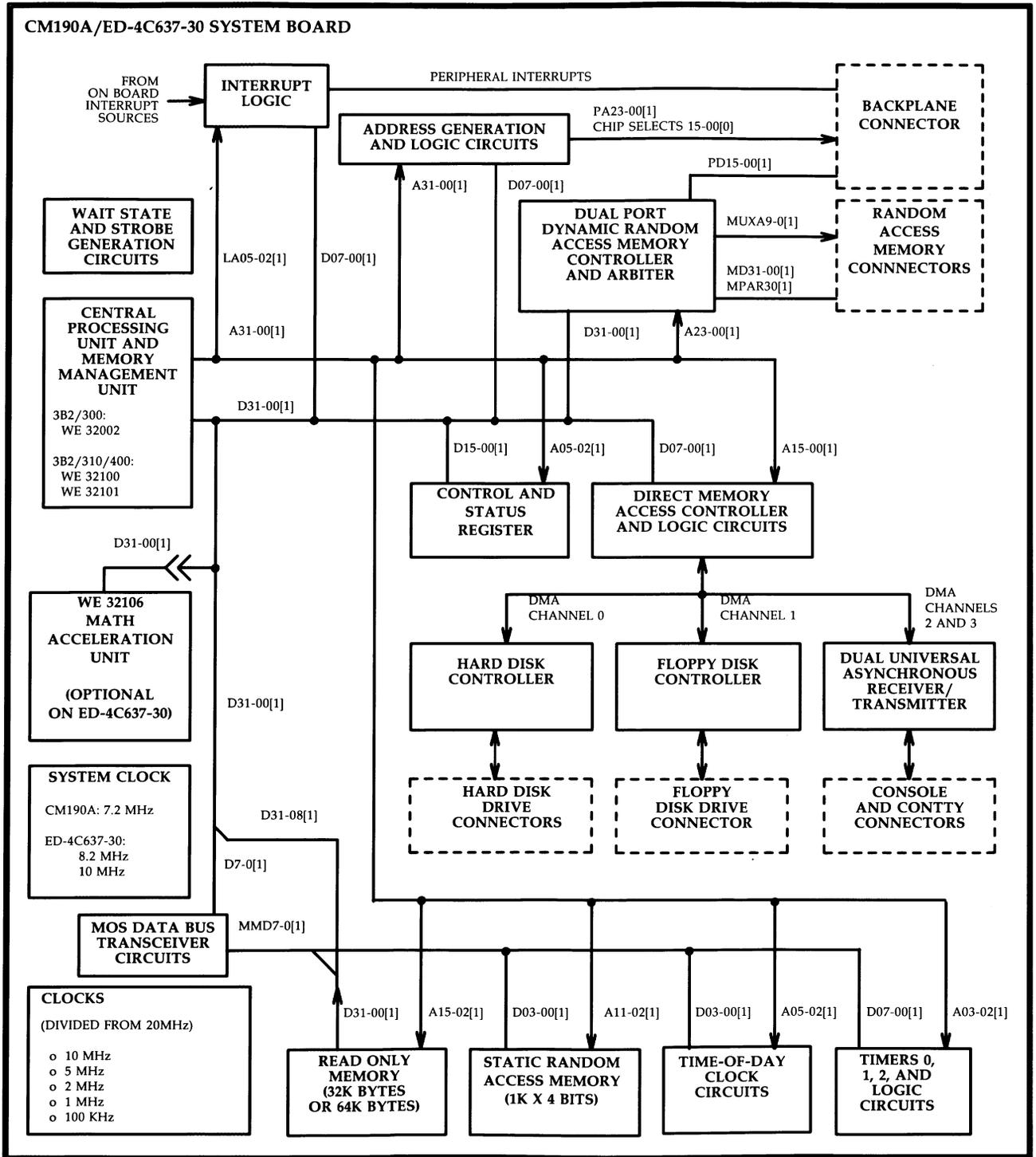
Figure 3-13: Version 2 3B2 Computer System Board — Functional Block Diagram
