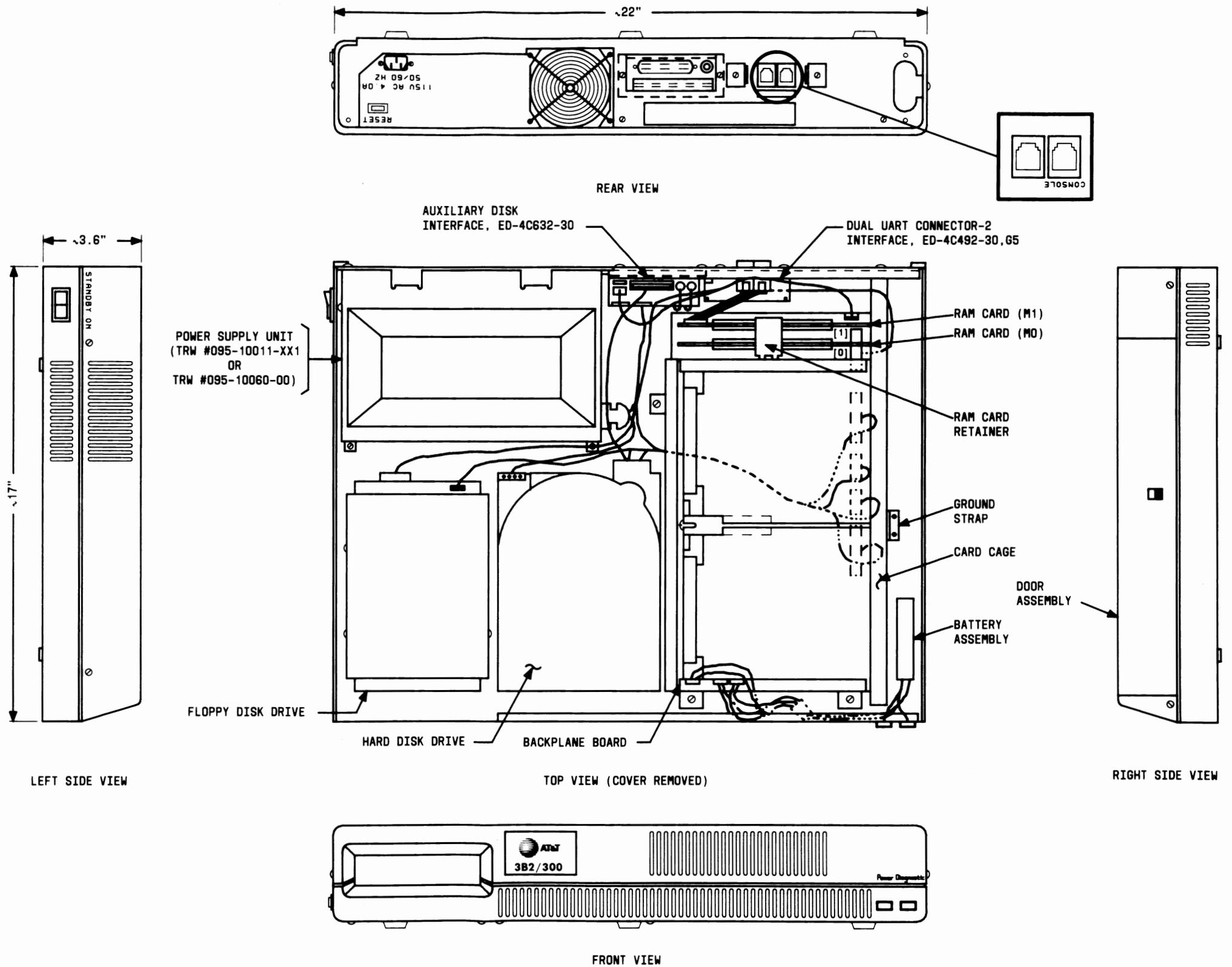
Figure 2-1: Domestic 3B2/300 Computer Cabinet Assembly Drawing (ED-4C492-30)
