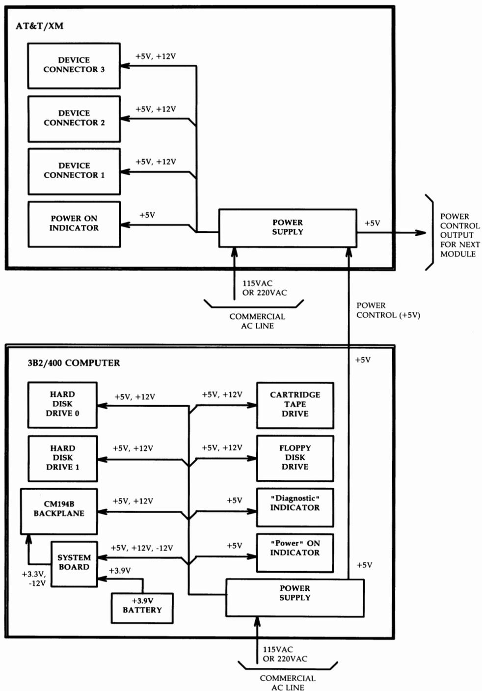
Figure 3-97: 3B2/400 Computer and AT&T/XM Power — Functional Block Diagram
