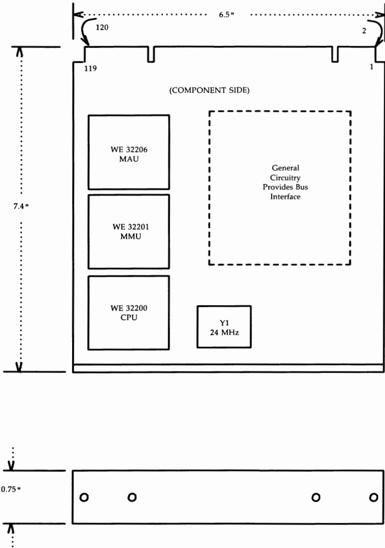
Figure B-33: CM524A PE Card Layout
