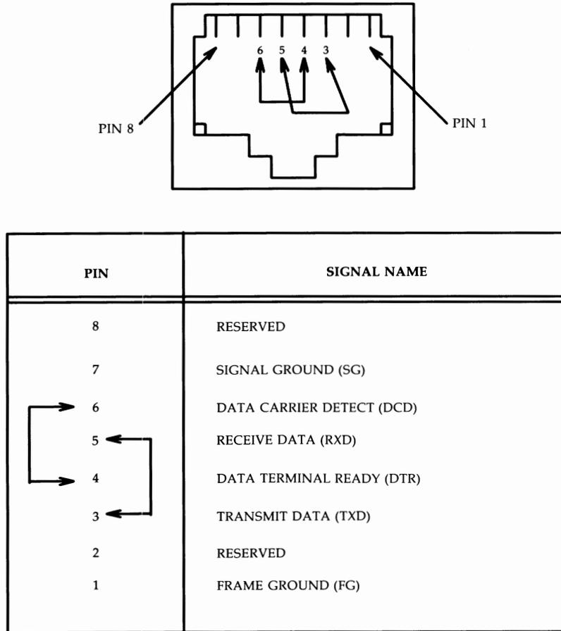
Figure B-41: PORTS Loop Around Connections
