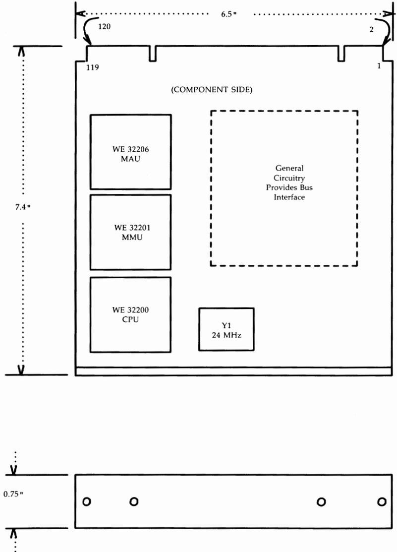
Figure B-33: CM524A PE Card Layout
