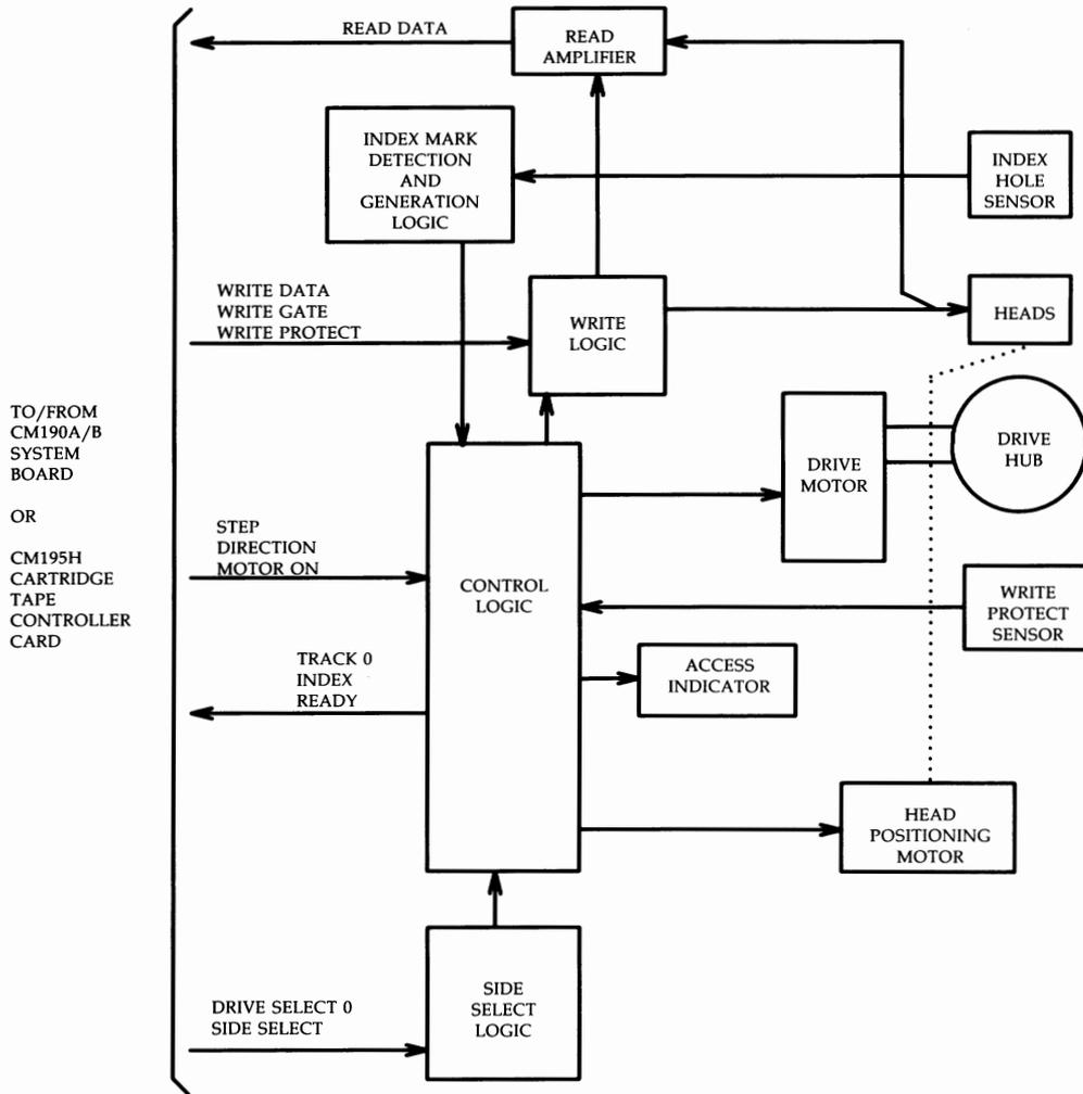
Figure 3-88: Floppy Disk Drive — Functional Block Diagram
