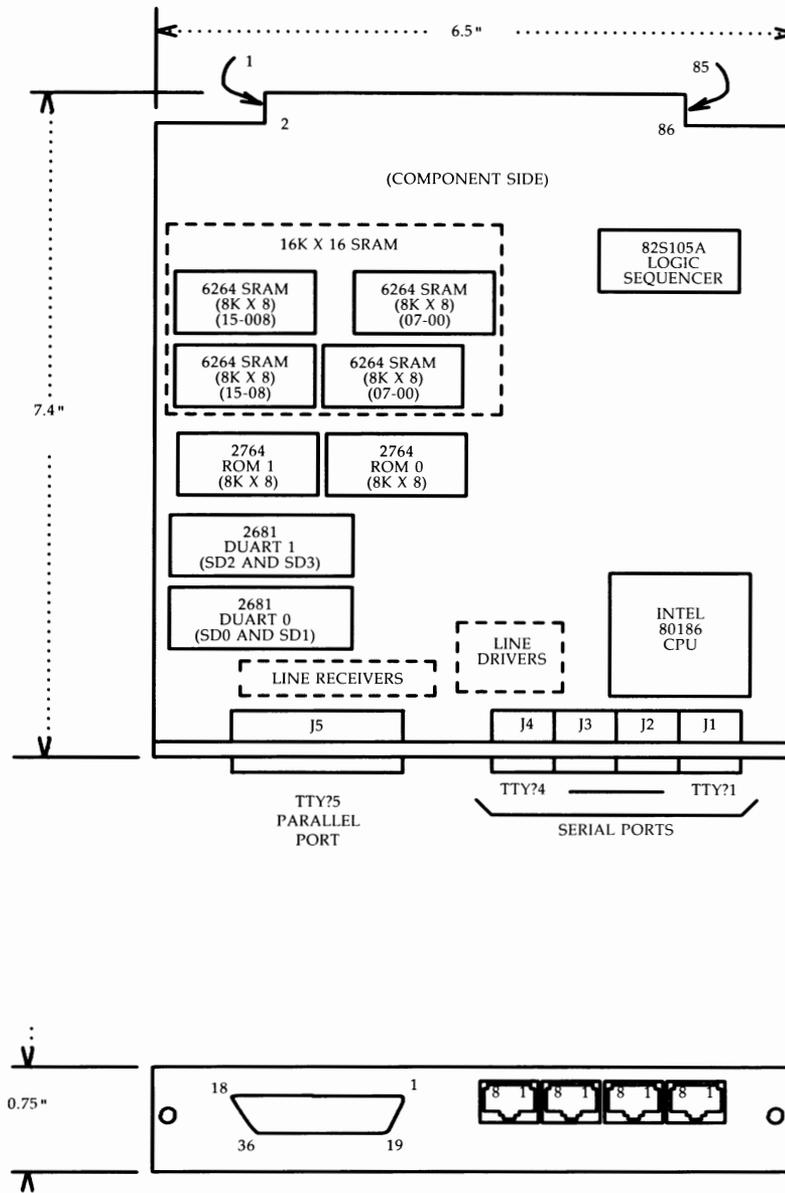
Figure 2-49: CM195B PORTS Card Layout (Early Production)
