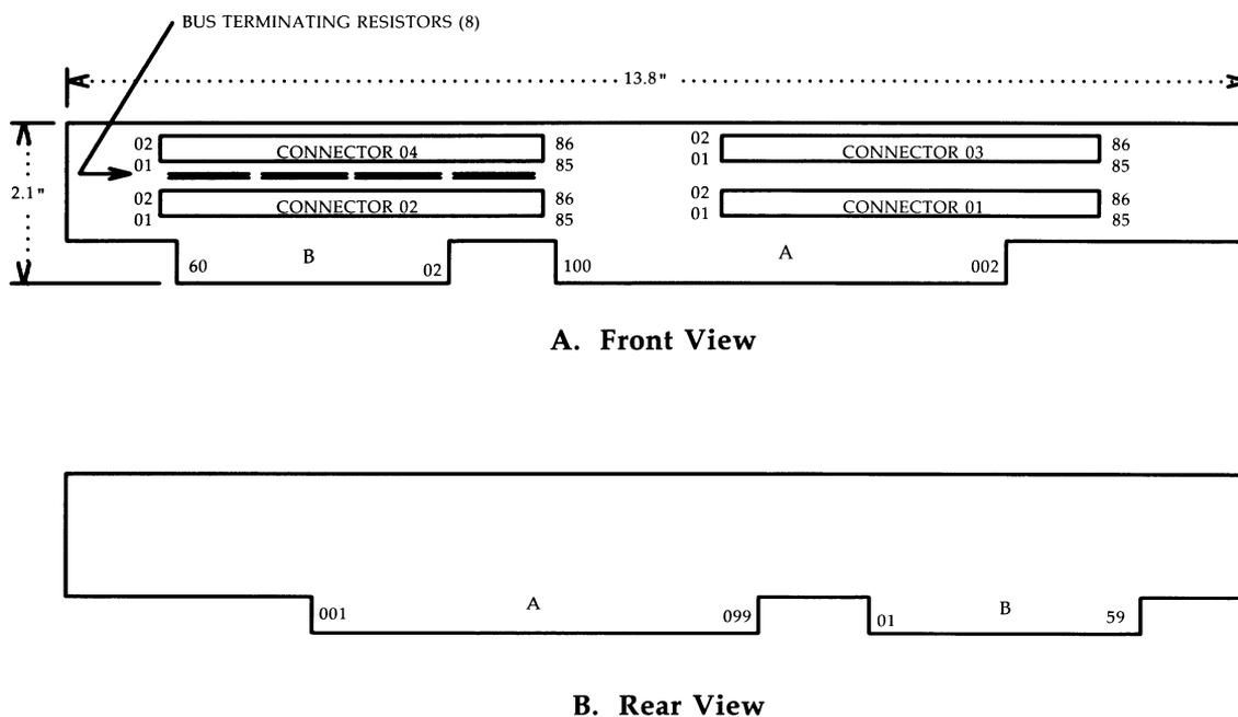
Figure 2-37: CM193A/B Backplane Board Layout
