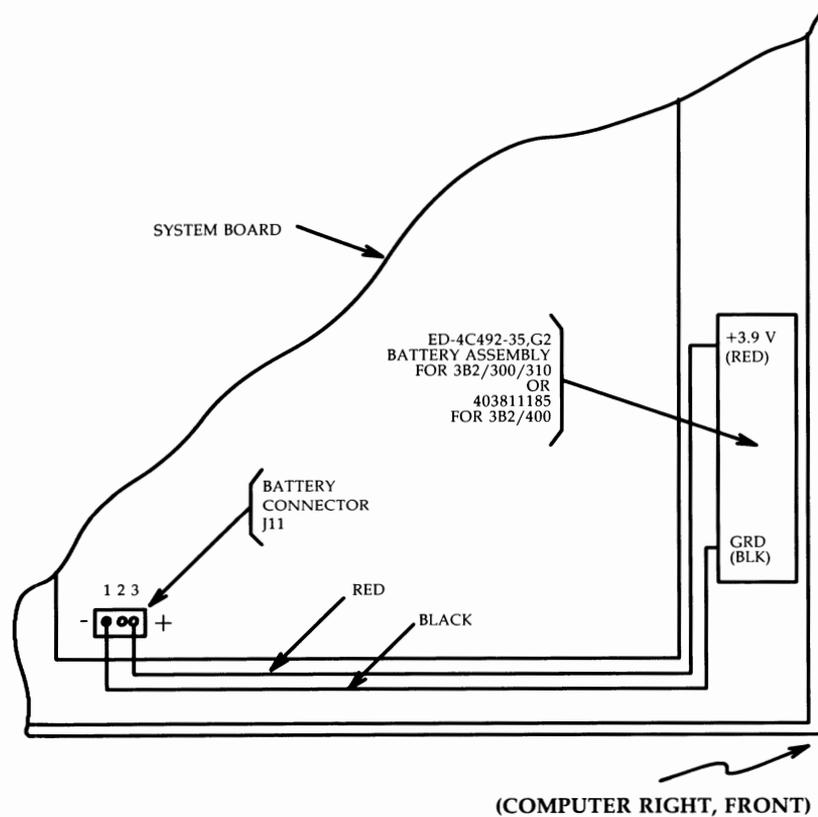
Figure 2-63: Version 2 Computer Backup Battery Supply Layout
