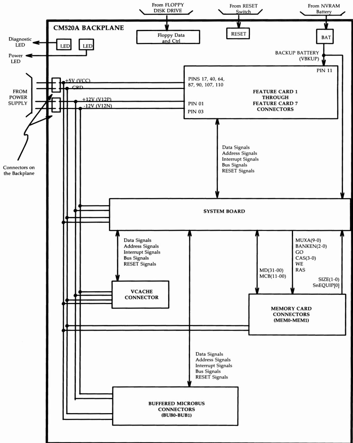
Figure 3-52: CM520A (3B2/500) Backplane — Functional Block Diagram
