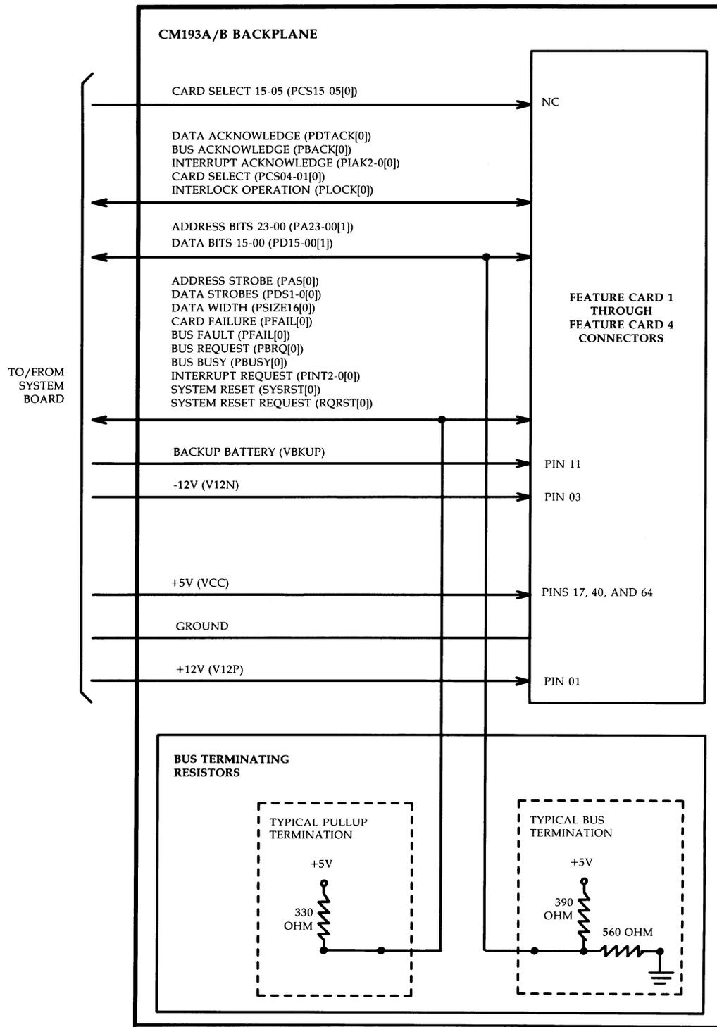
Figure 3-48: CM193A/B (3B2/300 and 310) Backplane — Functional Block Diagram
