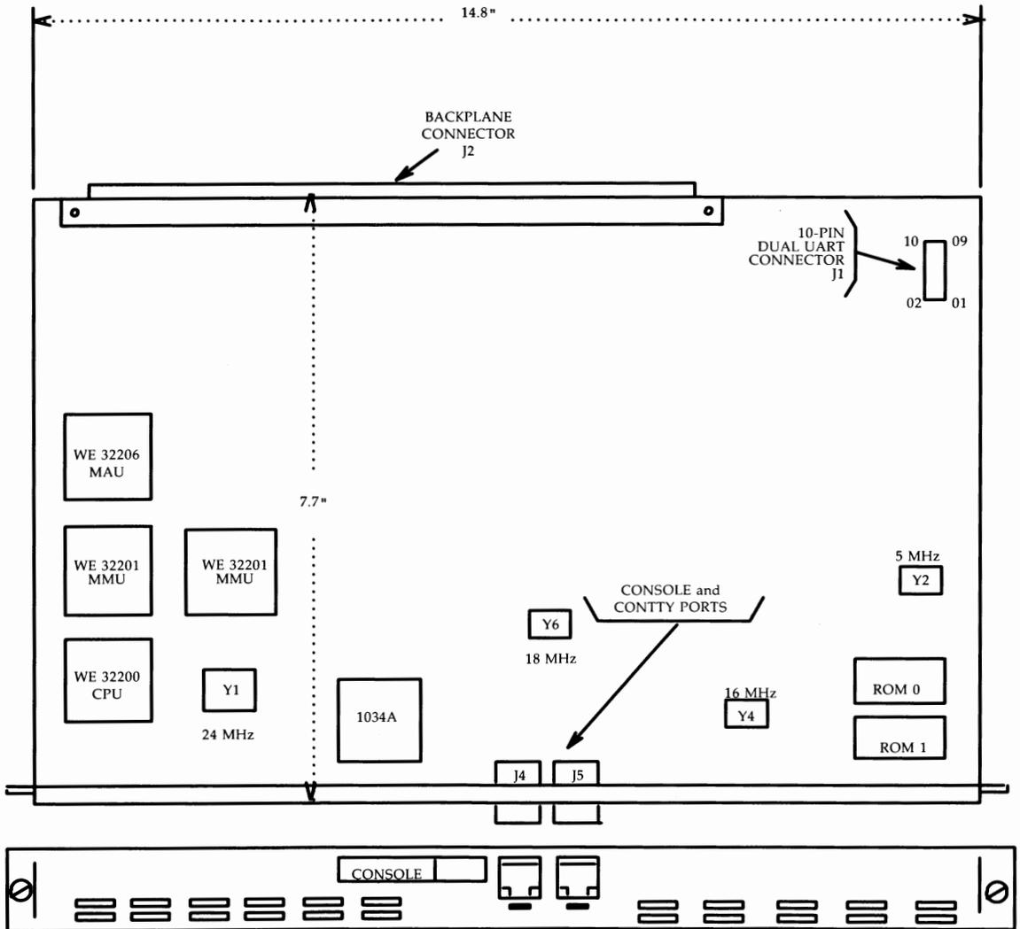
Figure B-5: CM518C System Board Layout
