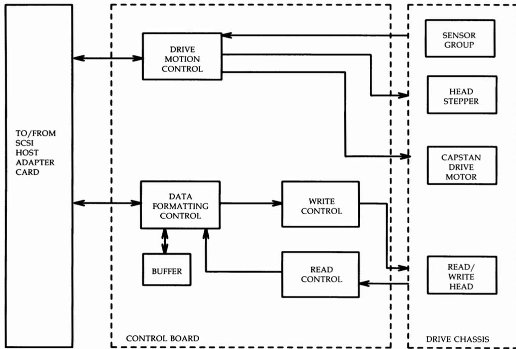
Figure 3-92: 60-Megabyte Cartridge Tape Drive — Functional Block Diagram
