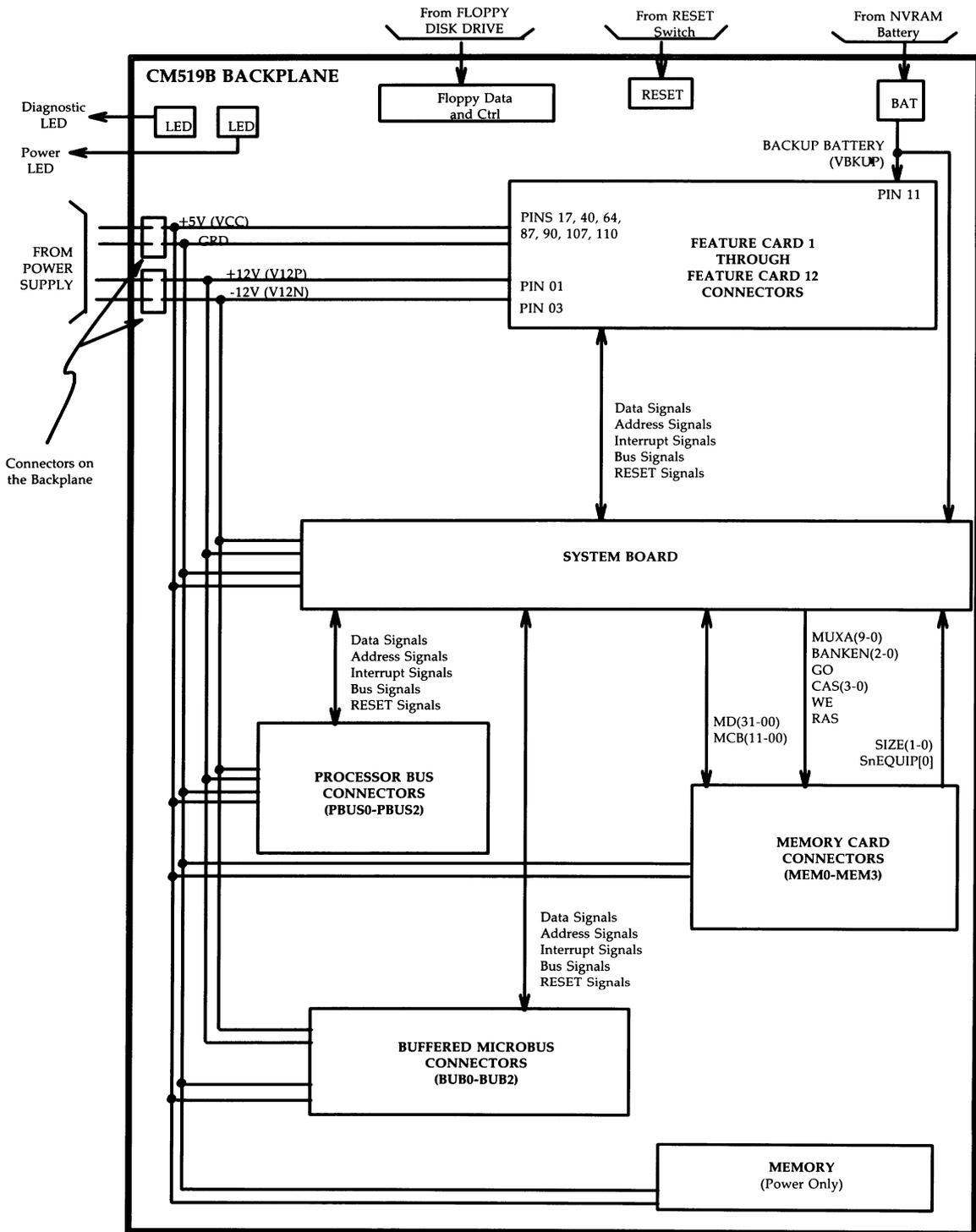
Figure 3-51: CM519B (3B2/1000) Backplane — Functional Block Diagram
