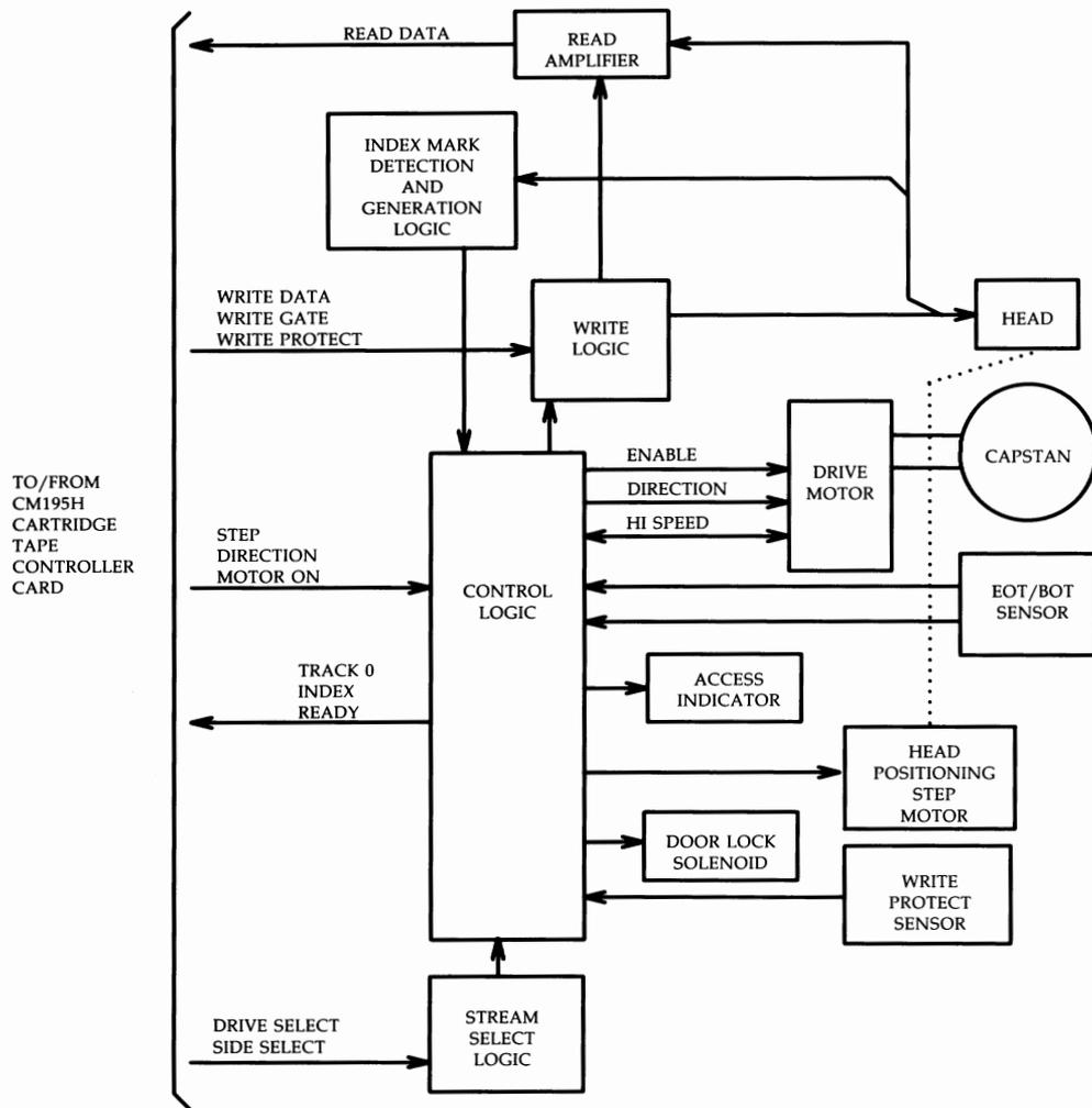
Figure 3-90: 23-Megabyte Cartridge Tape Drive — Functional Block Diagram
