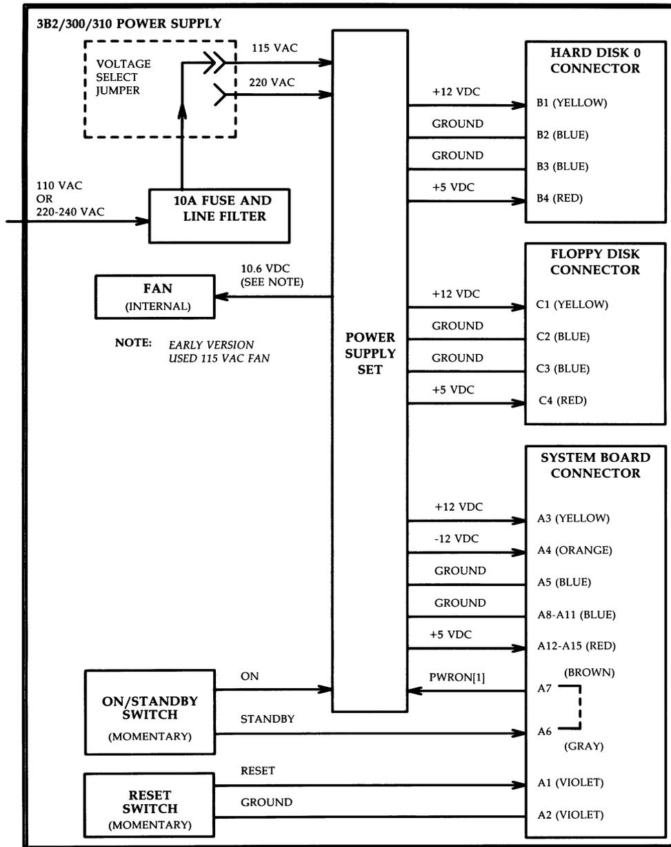
Figure 3-98: 3B2/300 and 310 Computer Power Supply — Functional Block Diagram
