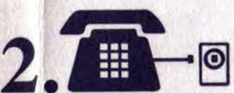
2. Unplug all telephone equipment from wall jacks. Wait 5 minutes. Replug a telephone into the wall jack. (Don't forget answering machines, speed dialers, etc.)
