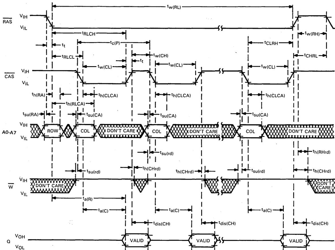
NOTE: A write cycle or a read-modify-write cycle can be intermixed with read cycles as long as the write and read-modify-write timing specifications are not violated.
