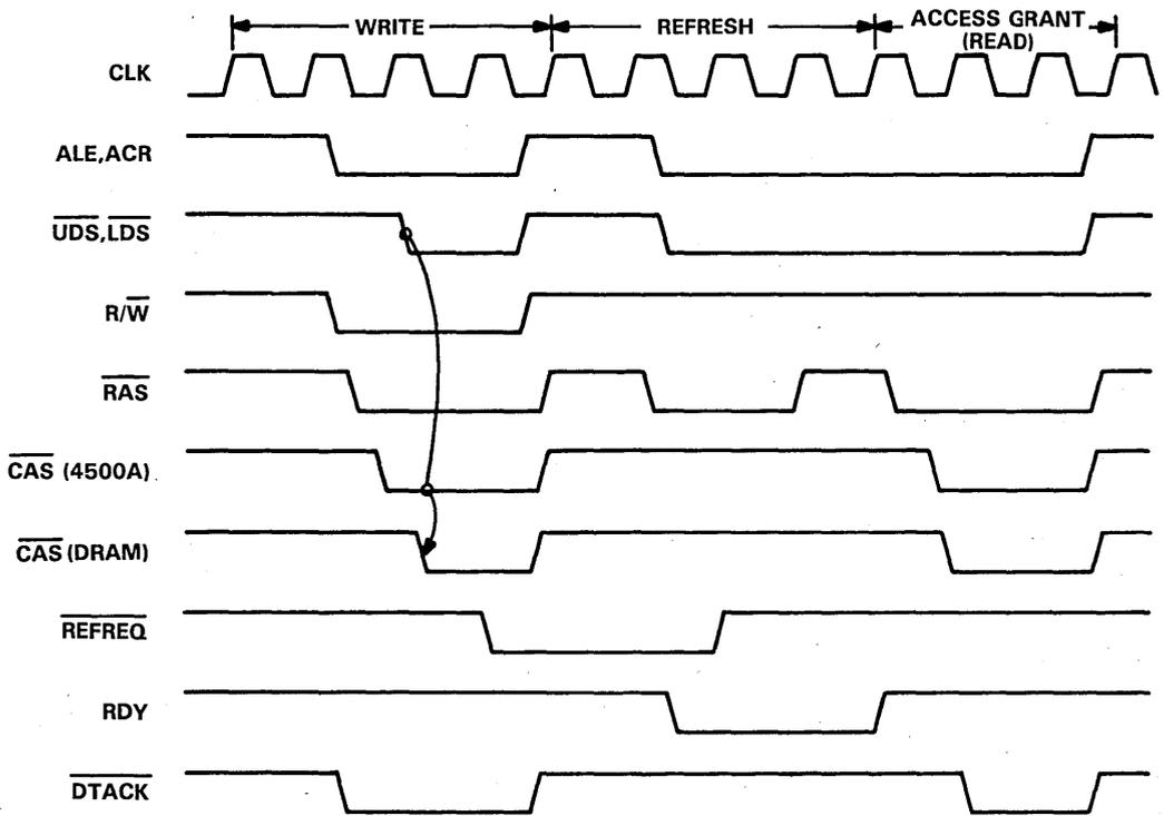
FIGURE 1B - TIMING DIAGRAM (GATED  $\overline{\text{CAS}}$ )
