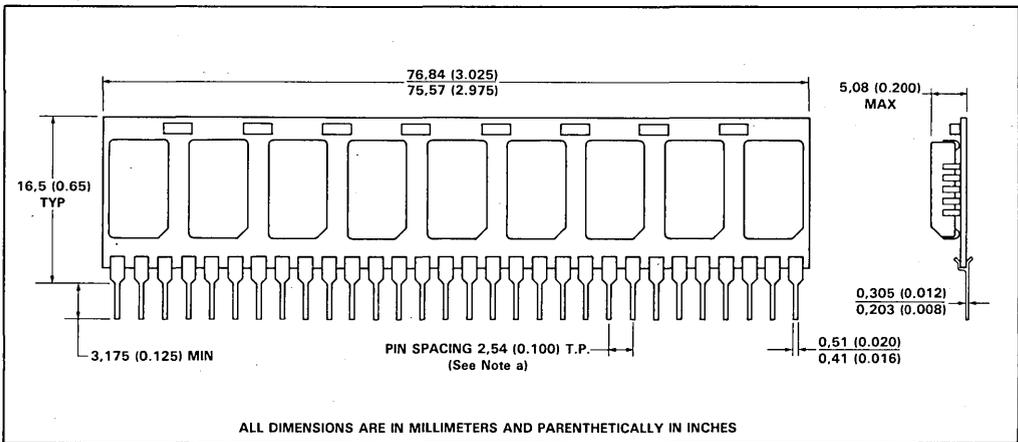
NOTE a. Each pin centerline is located within 0,25 (0.010) of its true longitudinal position.
