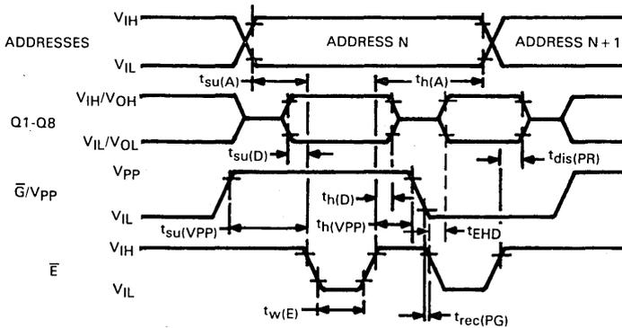
Timing measurement reference levels: Inputs 0.8 V and 2 V
