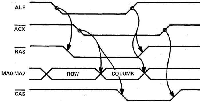
FIGURE 1 — ALE LEADING  $\overline{\text{ACX}}$
