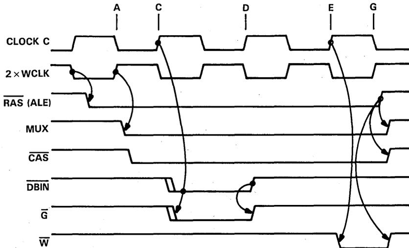
Figure 3. RMW Cycle Timing
