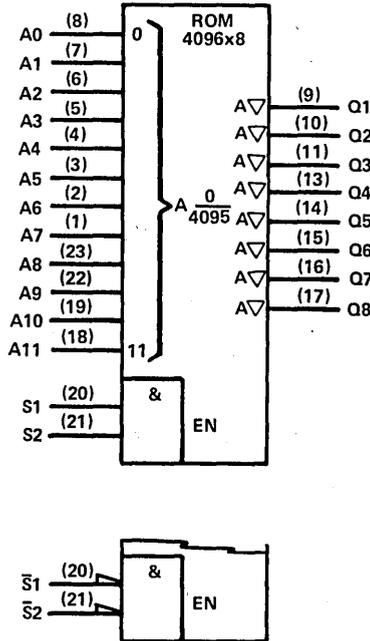
Pins 20 and 21 can be active-high as shown in the upper symbol or active-low as shown in the lower (partial) symbol.
