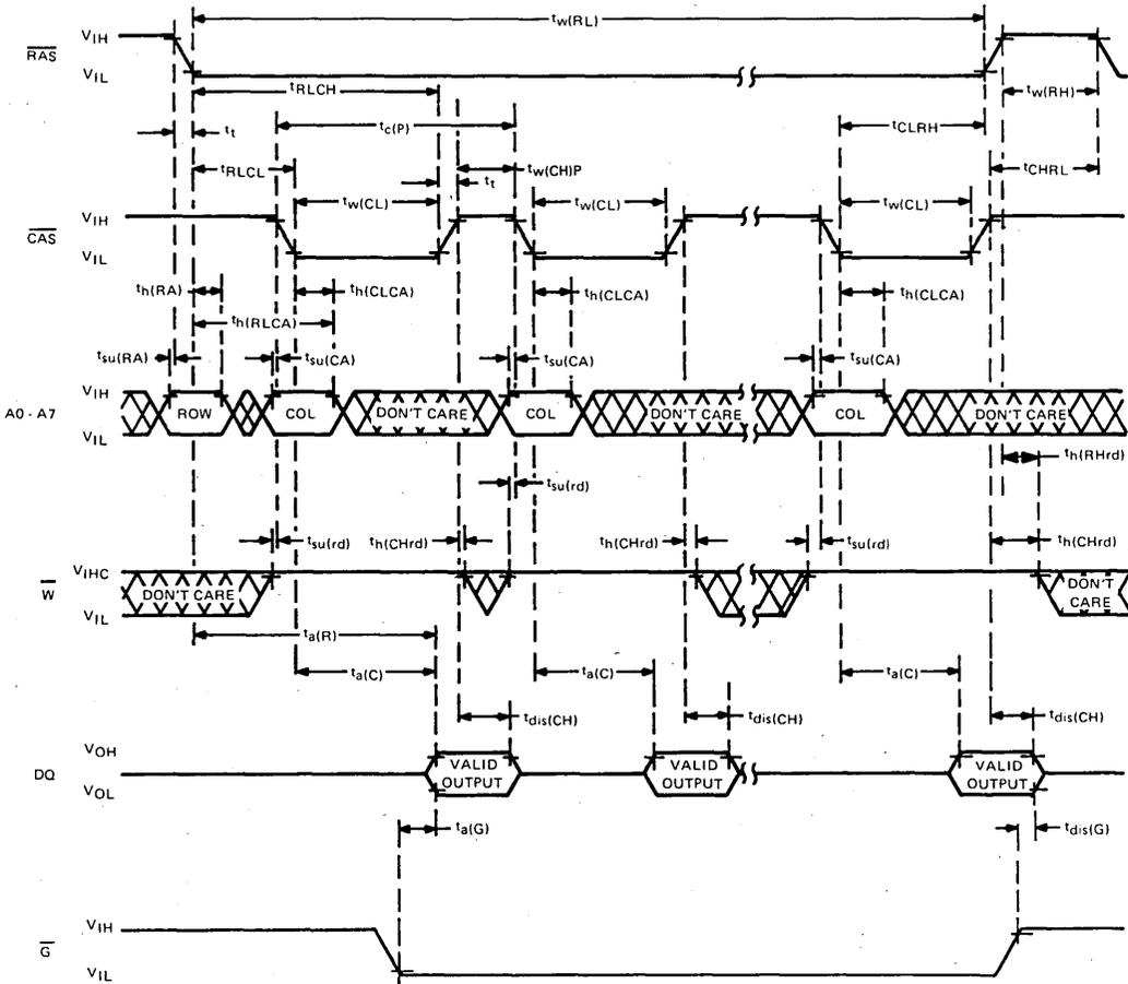
NOTE: A write cycle or read-modify-write cycle can be intermixed with read cycles as long as the write and read modify-write timing specifications are not violated.
