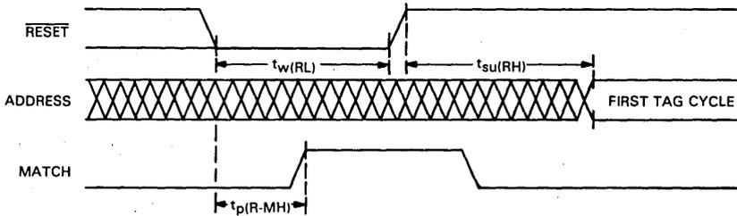
NOTE: Input pulse levels are 0 V and 3 V, with rise and fall times of 5 ns. The timing reference levels on the input pulses are 0.8 V and 2.0 V. The timing reference level for output pulses is 1.5 V. See Figures 1A and 1B for output loading.
