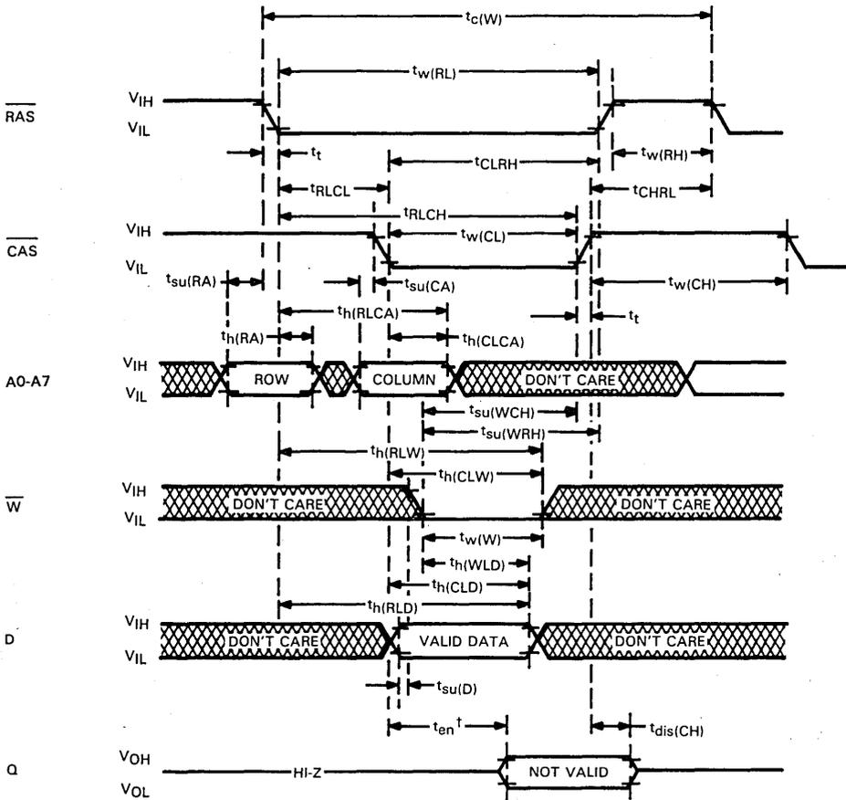
† The enable time ( $t_{en}$ ) for a write cycle is equal in duration to the access time from  $\overline{\text{CAS}}$  ( $t_{a(C)}$ ) in a read cycle; but the active levels at the output are invalid.
