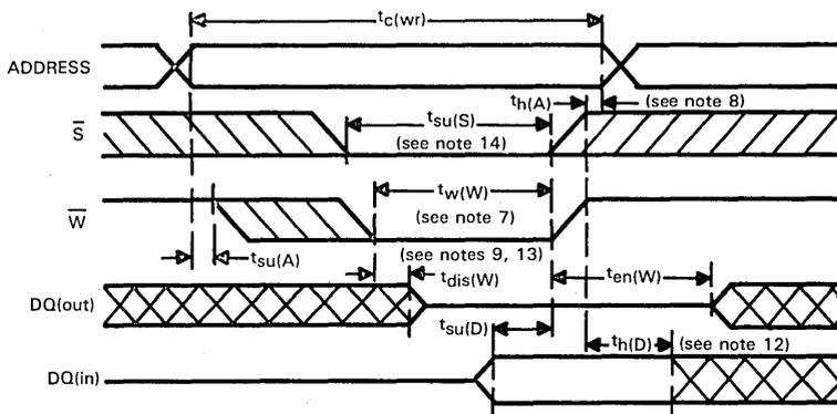
All timing reference points are 0.8 V and 2.0 V on inputs and 0.6 V and 2.2 V on outputs (90% points). Input rise and fall times equal 10 nanoseconds.
