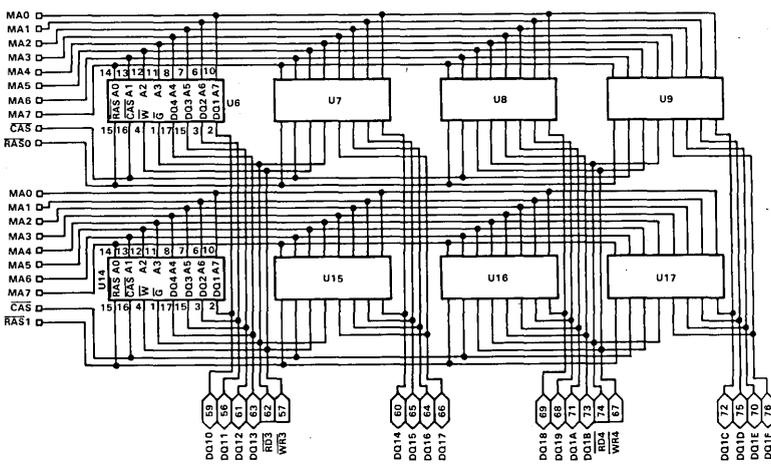
FIGURE 6 - TMS4416/TMS4500A BOARD SCHEMATIC
