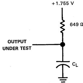
FIGURE 1 - OUTPUT LOAD
