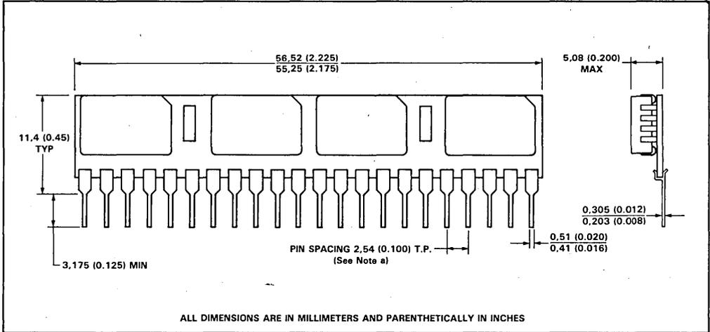
NOTE a. Each pin centerline is located within 0.25 (0.010) of its true longitudinal position.
