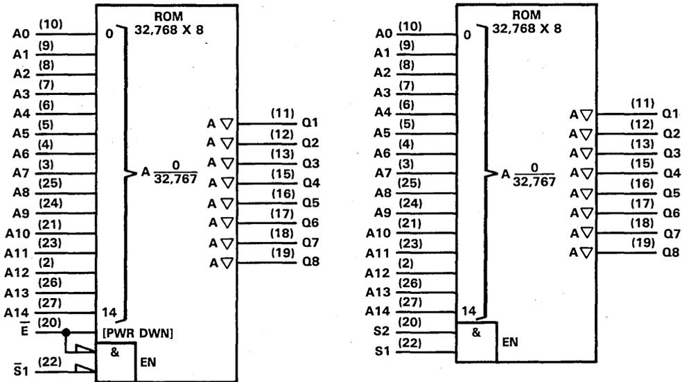
Pins 20 and 22 can be active-low as shown in the symbol on the left or active-high as shown in the symbol on the right. In addition, pin 20 can be either a secondary chip select (S2 or S2) or a chip enable/power down (E or  $\bar{E}$ ).
