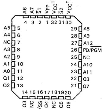
†Connected internally. VCC need be supplied to only one of these two pins.
