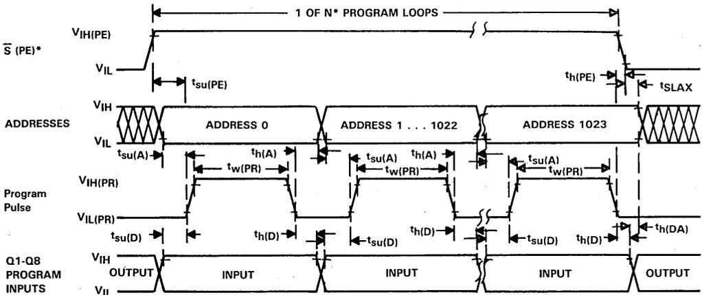
\* $\bar{S}(\text{PE})$  is at +12 V through N program loops where  $N < 100 \text{ ms}/t_{w(\text{PR})}$ .
