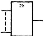
Even-parity element. The output stands at its 1-state if an even number of inputs stand at their 1-states.
