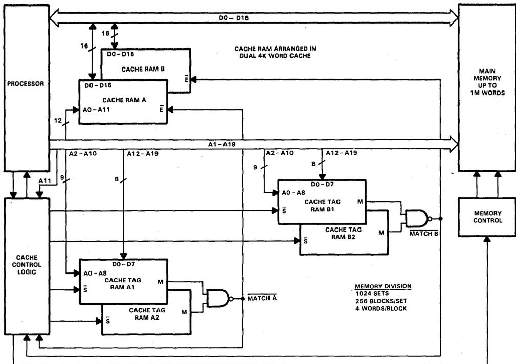
FIGURE 6 – CACHE MEMORY CONFIGURATION: DUAL CACHE ( $K=2$ )
