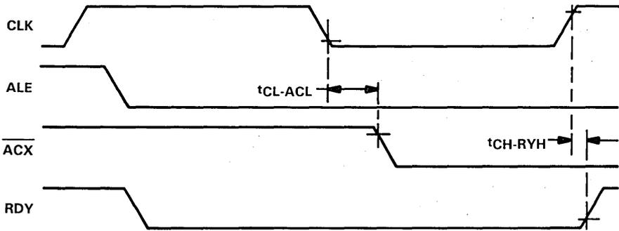
RDY starting high is timed from CLK high ( $t_{CH-RYH}$ ) for the condition  $\overline{ACX}$  going low while CLK low.
