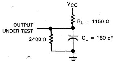
FIGURE 1 - LOAD CIRCUIT
