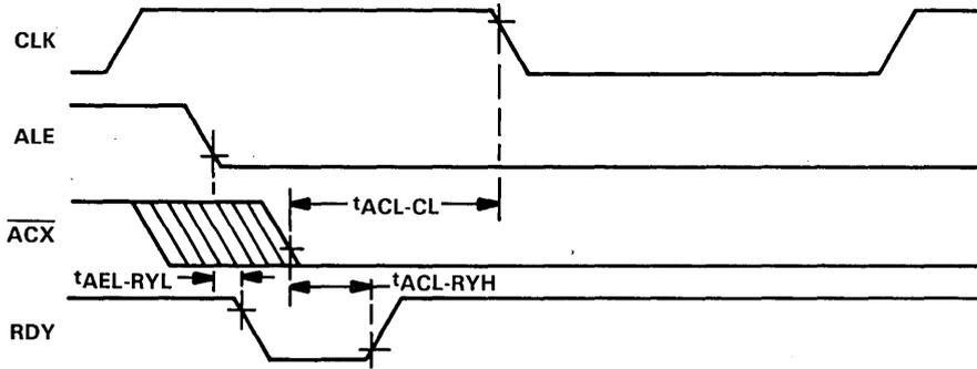
RDY starting high is timed from  $\overline{ACX}$  low ( $t_{ACL-RYH}$ ) for the condition  $\overline{ACX}$  going low while CLK high.
