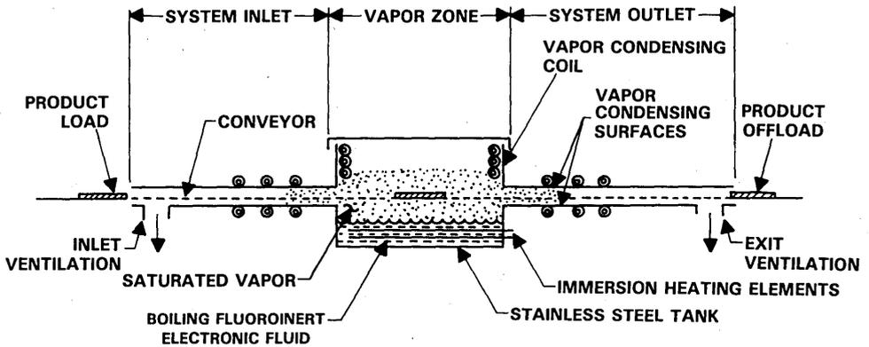
Figure 7. In-Line Single Vapor Heating System Schematic
