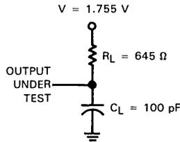
FIGURE 1 – LOAD CIRCUIT
