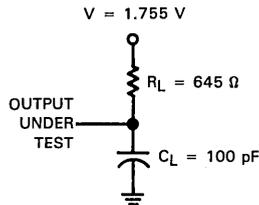
FIGURE 1 - LOAD CIRCUIT
