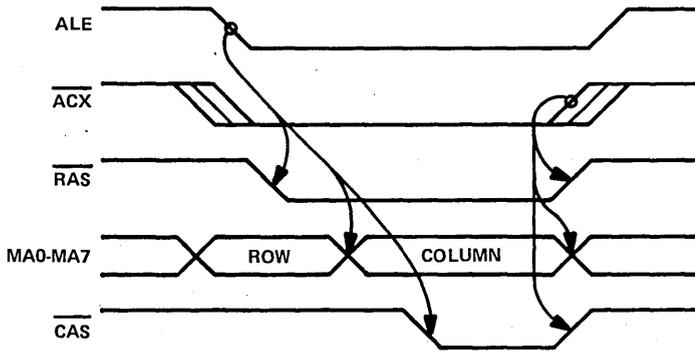
FIGURE 3 —  $\overline{\text{ACX}}$  PRIOR TO OR COINCIDENT WITH ALE
