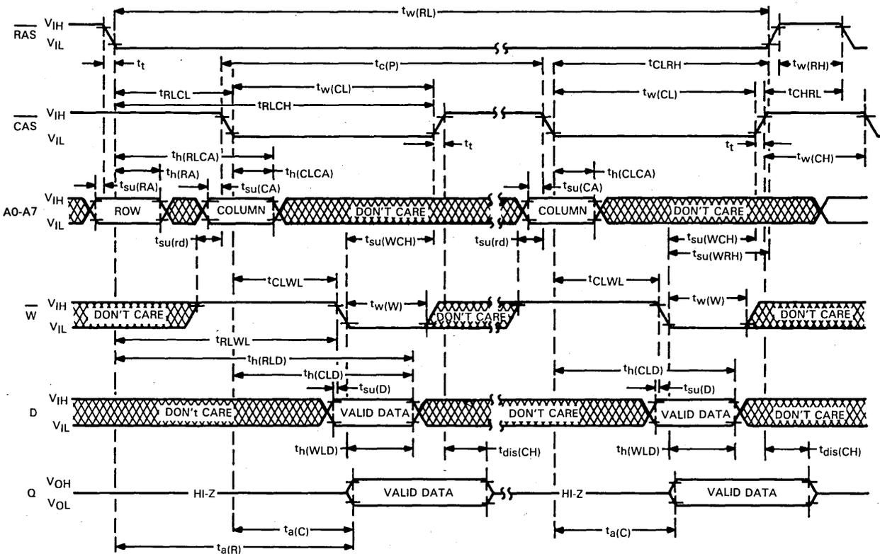
NOTE: A read or a write cycle can be intermixed with read-modify-write cycles as long as the read and write timing specifications are not violated.
