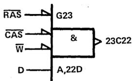
By virtue of the AND relationship between  $\overline{CAS}$  and  $\overline{W}$  (explicitly shown), when either one of these inputs goes low with the other one and  $\overline{RAS}$  already low ( $\overline{RAS}$  is AND'ed by G23), the D input is momentarily enabled (through C22). In an "early-write" cycle it is  $\overline{W}$  that goes low first; this causes the output to remain off as explained below.
