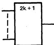
Odd-parity element. The output stands at its 1-state if an odd number of inputs stand at their 1-states.
