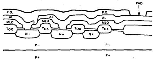
FIGURE 2B - CROSS SECTION OF CLAMPING CIRCUIT
