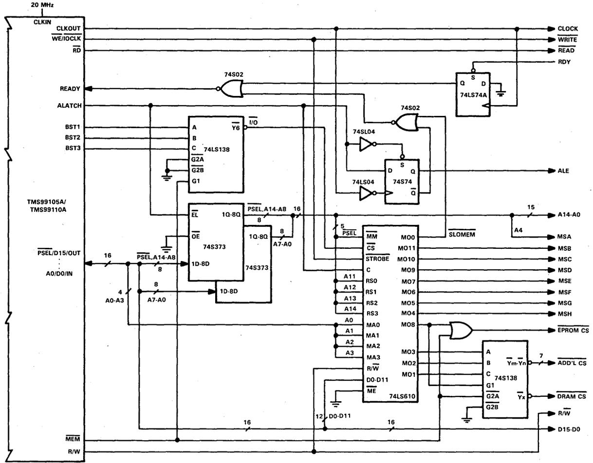
FIGURE 3 — TMS99105A/TMS99110A AND MEMORY MAPPING CIRCUITRY (5 MHz VERSION)
