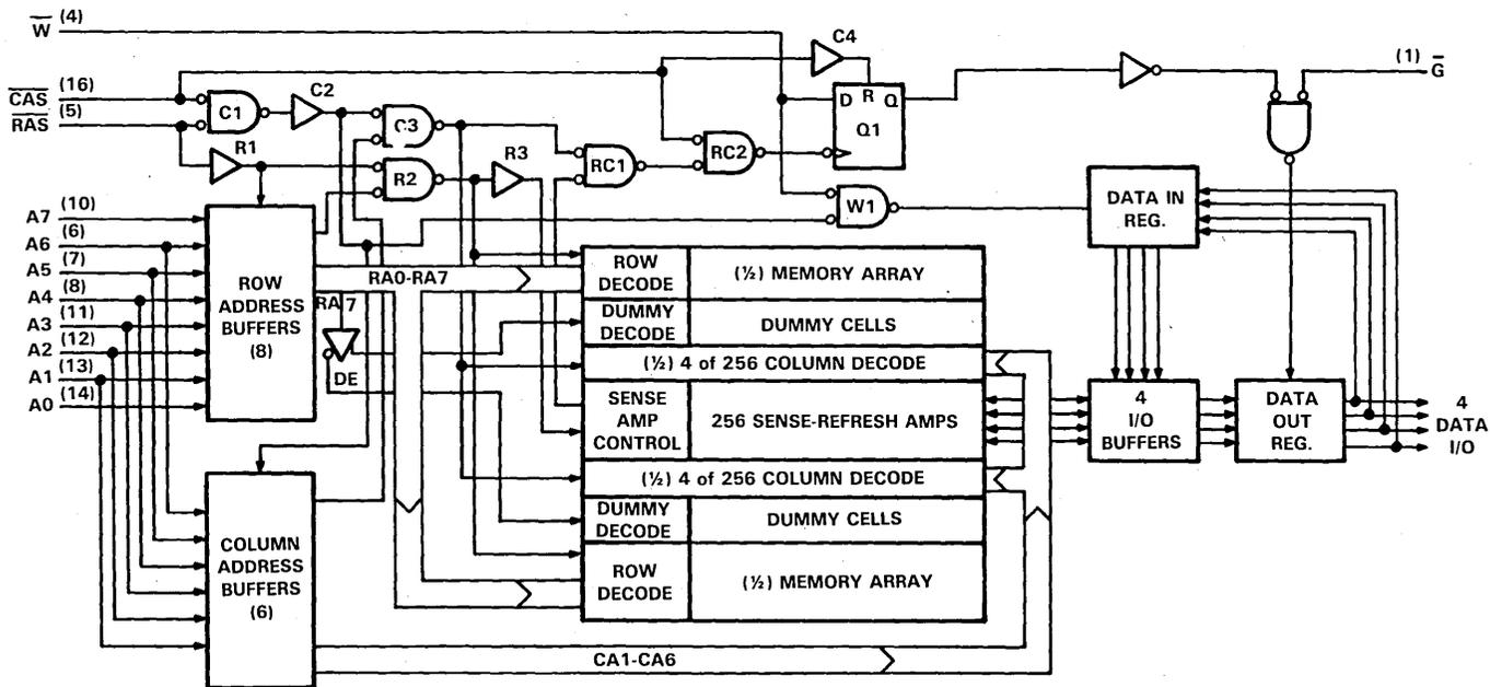
FIGURE 2 - TMS4416 BLOCK DIAGRAM
