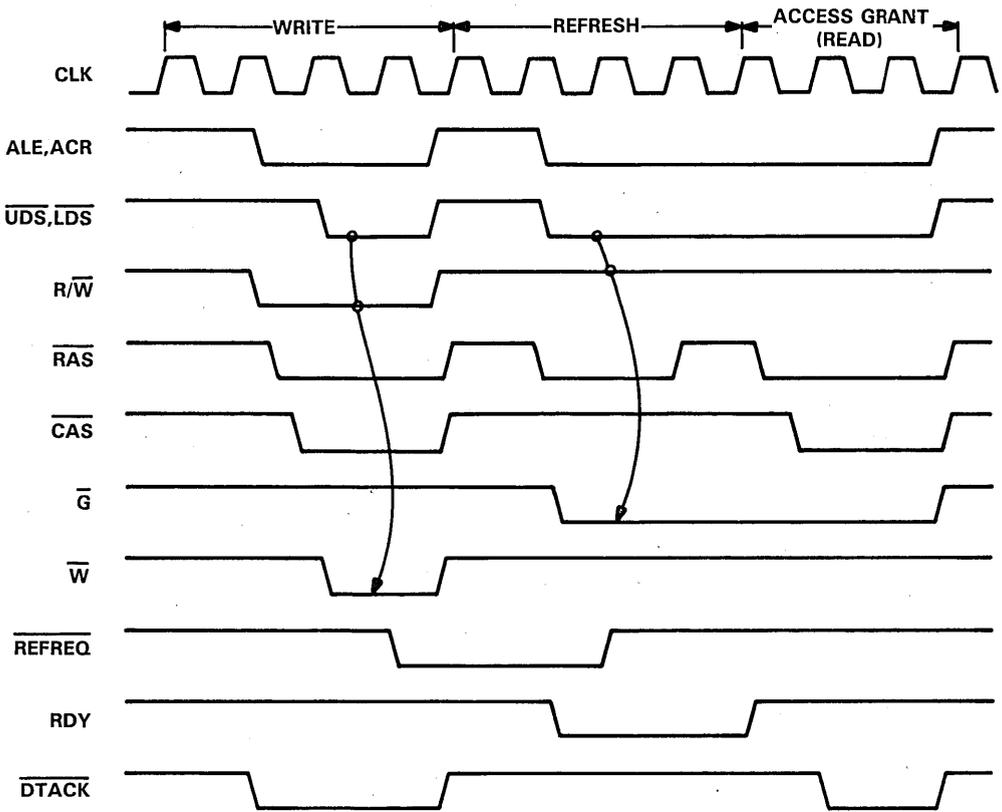
FIGURE 2B - TIMING DIAGRAM (GATED R/W)
