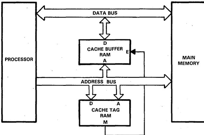
FIGURE 2 - TYPICAL MEMORY SYSTEM WITH CACHE
