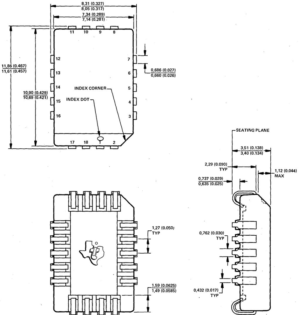
Figure 1. Plastic Chip Carrier Package (FP Suffix)
