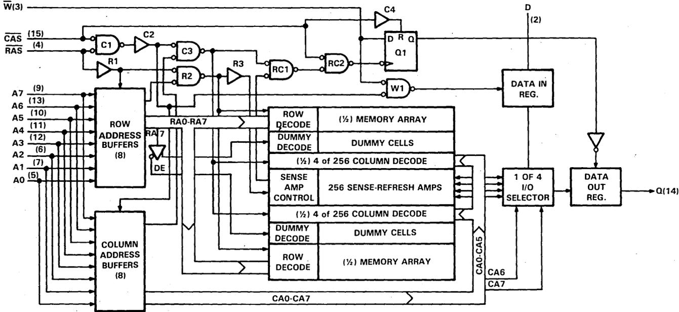
FIGURE 1 - TMS4164 BLOCK DIAGRAM
