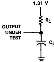
FIGURE 1 — LOAD CIRCUIT
