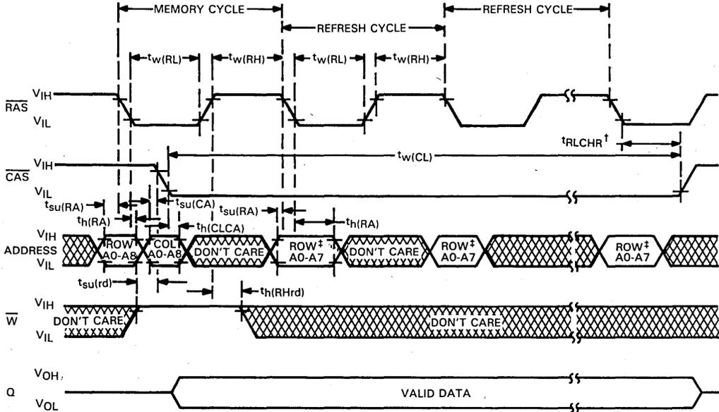
† For devices with  $\overline{\text{CAS}}$  before  $\overline{\text{RAS}}$  refresh option only.
