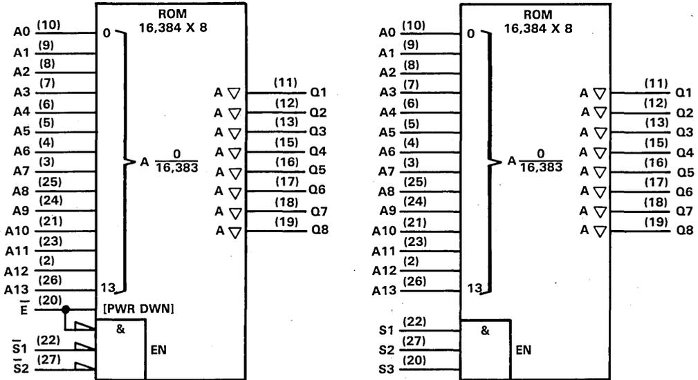
Pins 20, 22 and 27 can be active-low as shown in the symbol on the left or active-high as shown in the symbol on the right. In addition, pin 20 can be either a third chip select (S3 or  $\bar{S}3$ ) or a chip enable/power down (E or  $\bar{E}$ ).
