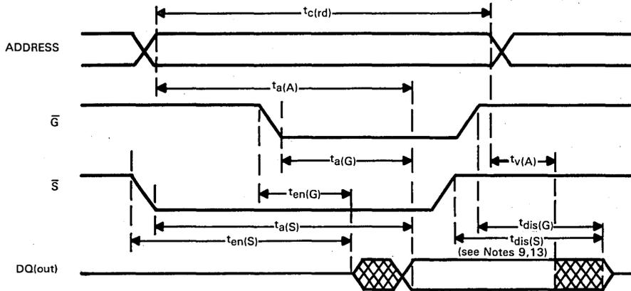
All timing reference points are 0.8 V and 2.0 V on inputs and 0.6 V and 2.2 V on outputs (90% points). Input rise and fall times equal 10 ns.
