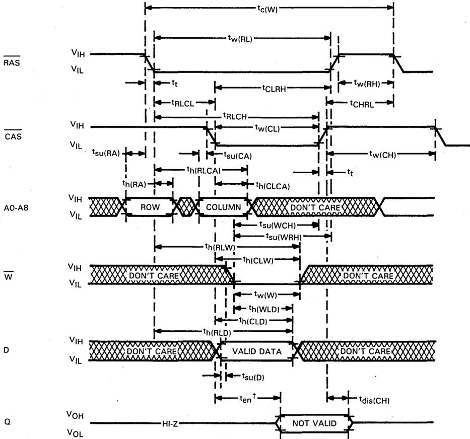
† The enable time ( $t_{en}$ ) for a write cycle is equal in duration to the access time from CAS ( $t_{a(C)}$ ) in a read cycle; but the active levels at the output are invalid.
