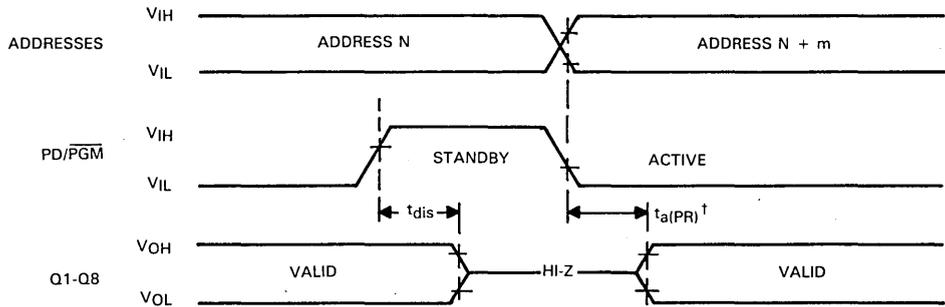
$^\dagger t_{a(PR)}$  referenced to PD/PGM or the address, whichever occurs last.
