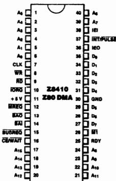
Figure 2. 40-pin Dual-In-Line Package (DIP), Pin Assignments
