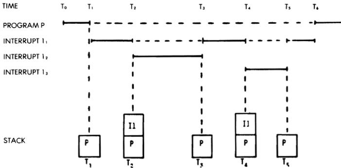
**Fig. 6.33: Stack Contents During Multiple Interrupts**
