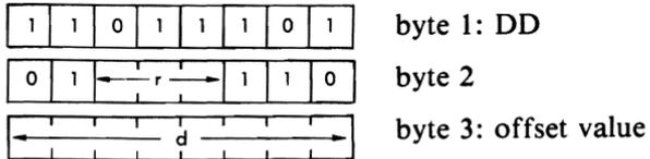
*Description:* The contents of the memory location addressed by the IX index register plus the given offset value, are loaded into the specified register. r may be any one of:
