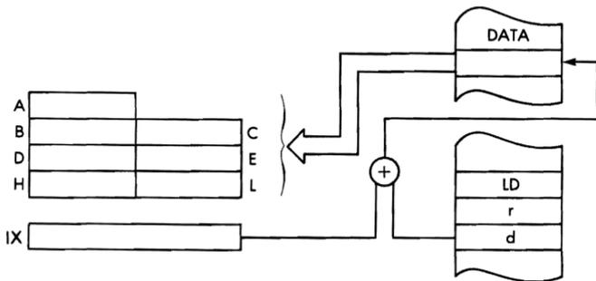
*Timing:* 5 M cycles; 19 T states; 9.5 usec @ 2 MHz
