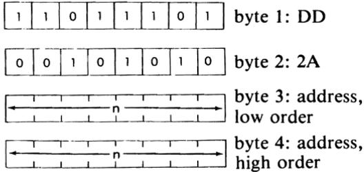
*Descriptions:* The contents of the memory location addressed by the memory locations immediately following the opcode are loaded into the low order of the IX register. The contents of the memory location immediately following the one loaded into the low order are loaded into the high order of the IX register. The low order of the nn address immediately follows the opcode.
