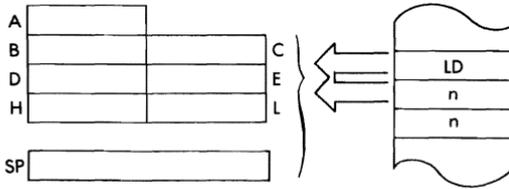
*Timing:* 3 M cycles; 10 T states; 5 usec @ 2 MHz
