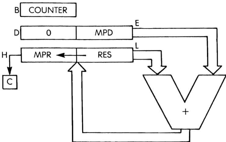
Fig. 3.25: Registers for Improved Multiply
