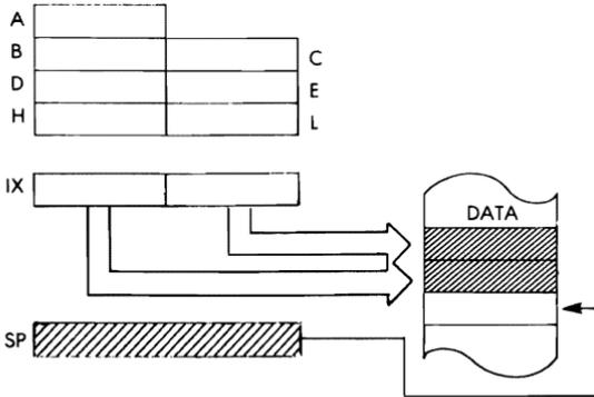
*Timing:* 4 M cycles; 15 T states; 7.5 usec @ 2 MHz
