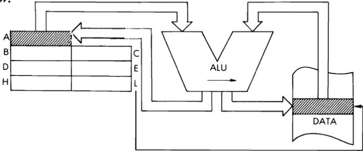
*Timing:* 5 M cycles; 18 T states; 9 usec @ 2 MHz
