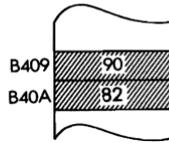
**EX (SP), IX** Exchange IX with top of stack.
