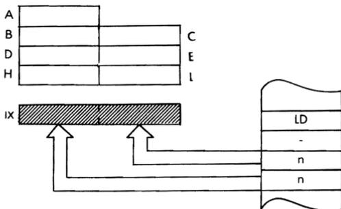
*Timing:* 4 M cycles; 14 T states; 7 usec @ 2 MHz
