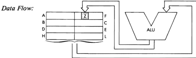
*Timing:* 2 M cycles; 8 T states; 4 usec @ 2 MHz
