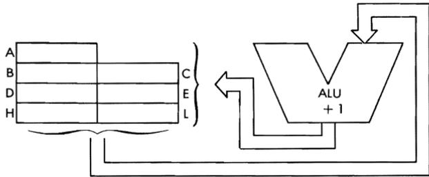
*Timing:*                      1 M cycle; 4 T states; 2 usec @ 2 MHz
