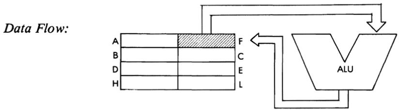
*Timing:* 1 M cycle; 4 T states: 2 usec @ 2 MHz
