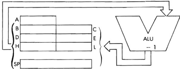
*Timing:*                      1 M cycle; 6 T states; 3 usec @ 2 MHz
