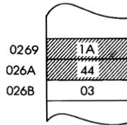
**SBC A, s** Subtract with borrow accumulator and specified operand.
