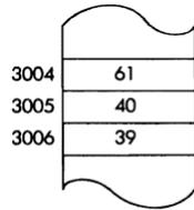
**PUSH qq** Push register pair onto stack.
