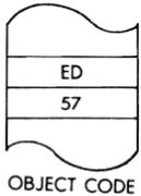
**LD I, A** Load Interrupt Vector register I from the accumulator.
