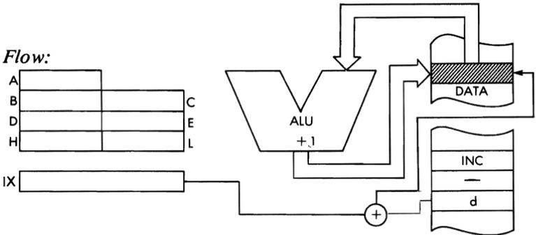
*Timing:* 6 M cycles; 23 T states; 11.5 usec @ 2 MHz
