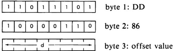
*Description:* The contents of the accumulator are added to the contents of the memory location addressed by the contents of the IX register plus the immediate offset value. The result is stored in the accumulator.
