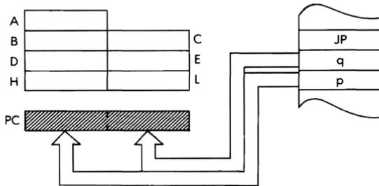
*Timing:*                         3 M cycles; 10 T states; 5 usec @ 2 MHz
