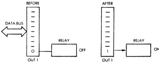
**Fig. 6.1: Turning on a Relay**
