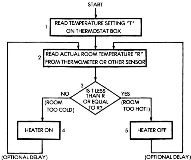
**Fig. 1.1: A Flowchart for Keeping Room Temperature Constant**
