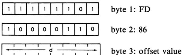
*Description:*            The contents of the accumulator are added to the contents of the memory location addressed by the contents of the IY register plus the given offset value. The result is stored in the accumulator.
