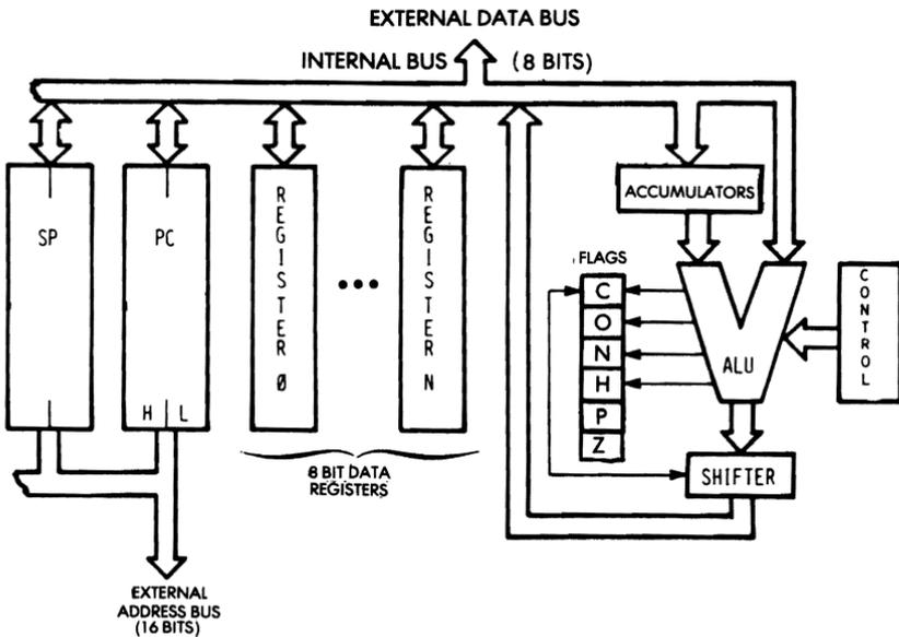
**Fig. 2.2: "Standard" Microprocessor Architecture**
