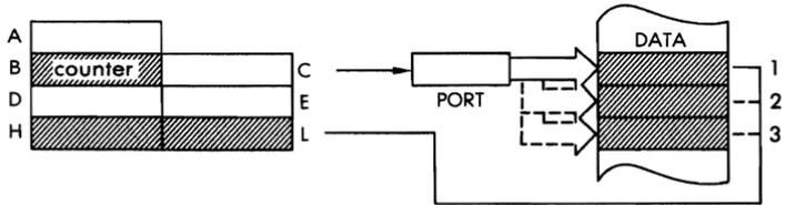
*Timing:* B = 0: 4 M cycles; 16 T states; 8 used @ 2 MHz.
