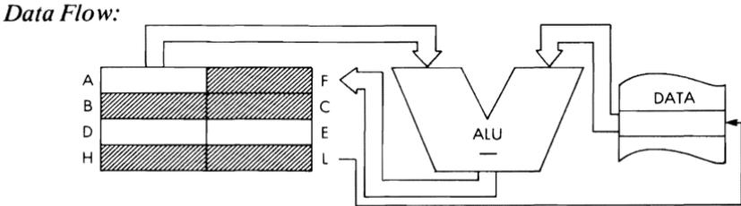
*Timing:* 4 M cycles; 16 T states; 8 usec @ 2 MHz
