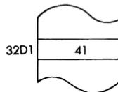
**LD A, (DE)** Load the accumulator from the memory location indirectly addressed by the DE register pair.
