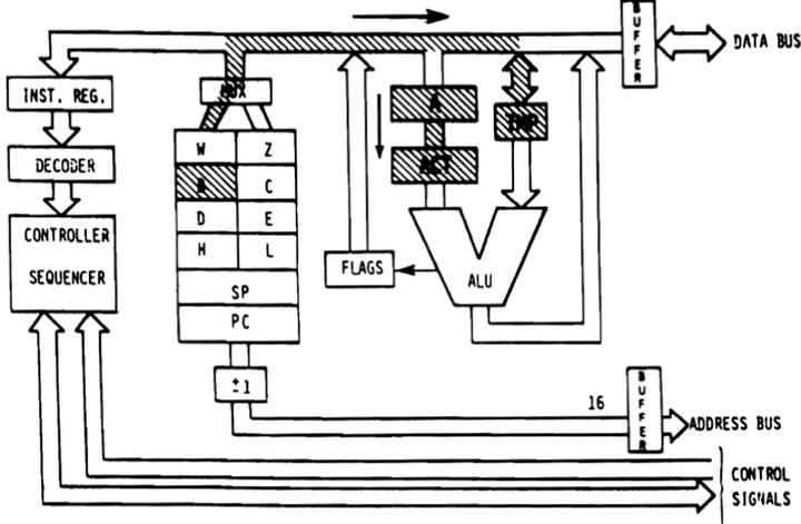
Fig. 2.23: Two Transfers Occur Simultaneously
