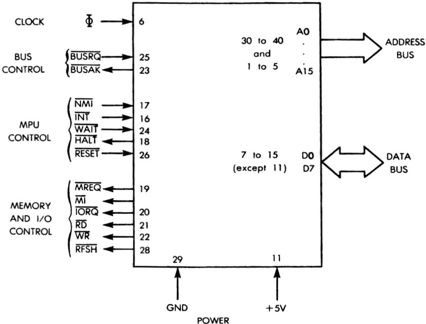
**Fig. 2.33: Z80 MPU Pinout**
