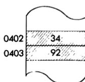
**EX (SP), IY** Exchange IY with top of stack.
