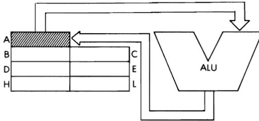
*Timing:* 1 M cycle; 4 T states; 2 usec @ 2 MHz
