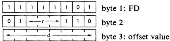
*Description:* The contents of the memory location addressed by the IY index register plus the given offset value, are loaded into the specified register. r may be any one of:
