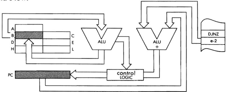
*Timing:*                       $B \neq 0$ : 3 M cycles; 13 T states; 6.5 usec @ 2 MHz.
