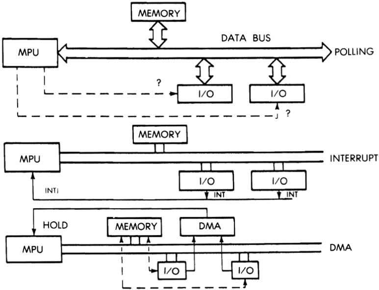
**Fig. 6.18: Three Methods of I/O Control**
