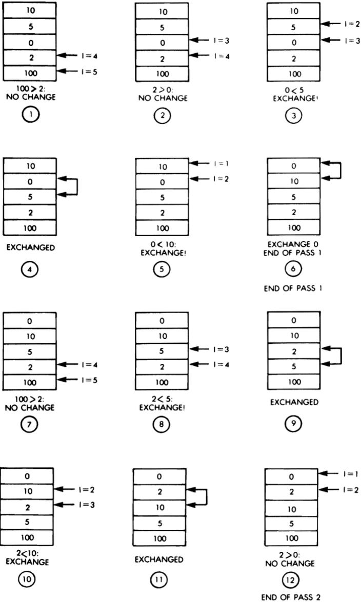
Fig. 8.5: Bubble-Sort Example: Phases 1 to 12
