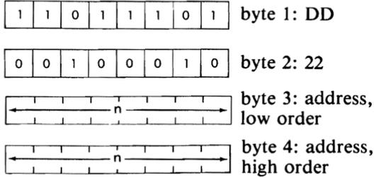
*Description:* The contents of the low order of the IX register are loaded into the memory location addressed by the contents of the memory location immediately following the opcode. The contents of the high order of the IX register are loaded into the memory location immediately following the one loaded from the low order. The low order of the nn address occurs immediately after the op code.
