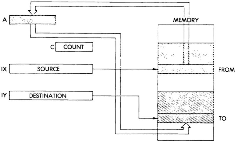
**Fig. 5.7: Block Transfer: Initializing the Register**
