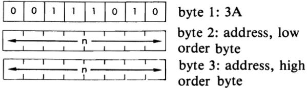
*Description:* The contents of the memory location addressed by the contents of the 2 memory locations immediately following the opcode are loaded into the accumulator. The low byte of the address occurs immediately after the opcode.
