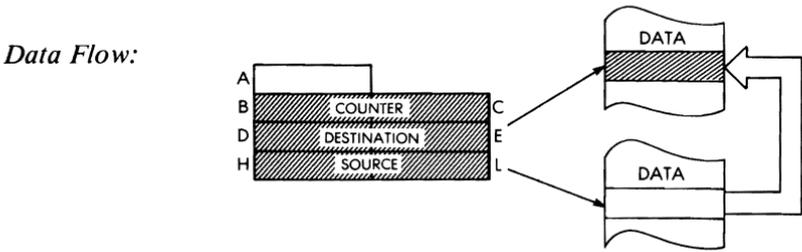
*Timing:* 4 M cycles; 16 T states; 8 usec @ 2 MHz
