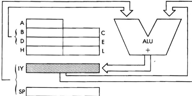
*Timing:*                    4 M cycles; 15 T states: 7.5 usec @ 2 MHz
