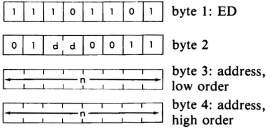
*Descriptions:* The contents of the low order of the specified register pair are loaded into the memory location addressed by the memory locations immediately following the opcode. The contents of the high order of the register pair are loaded into the memory location immediately following the one loaded from the low order. The low order of the nn address occurs immediately after the opcode. dd may be any of:
