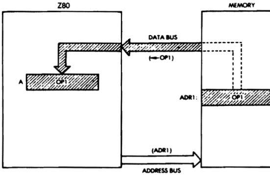
**Fig. 3.2: LD A, (ADR1): OPR is Loaded from Memory**
