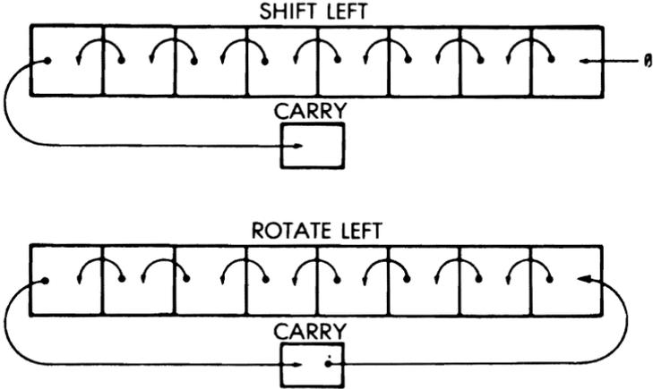
Fig. 4.1: Shift and Rotate
