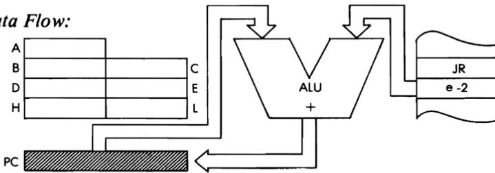
*Timing:*                    3 M cycles; 12 T states; 6 usec @ 2 MHz
