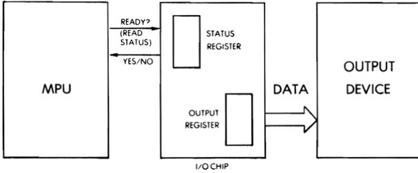
**Fig. 6.8: Handshaking (Output)**
