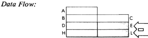
*Timing:* 1 M cycle; 4 T states; 2 usec @ 2 MHz
