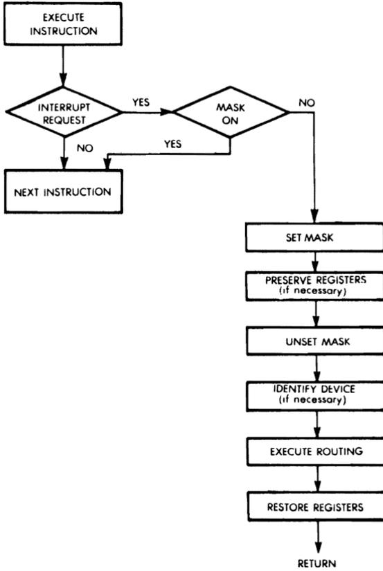
**Fig. 6.34: Interrupt Logic**
