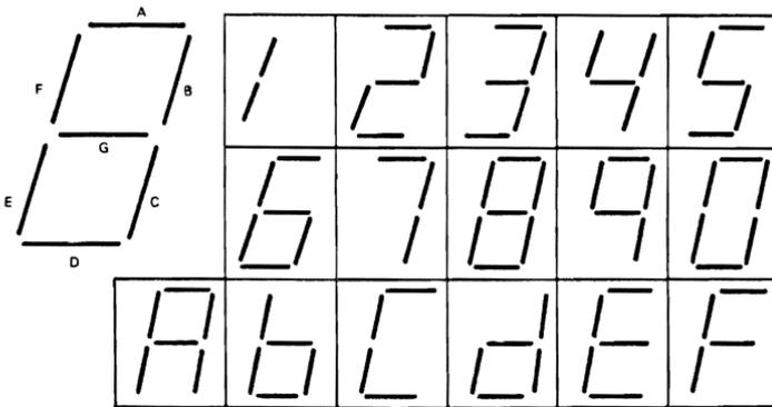
**Fig. 6.11: Hexadecimal Characters Generated with a Seven-Segment LED**
