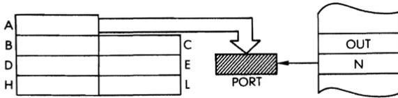
*Timing:*            3 M cycles, 11 T states; 5.5 usec @ 2 MHz
