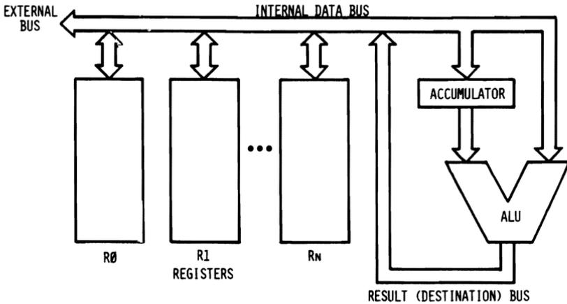
**Fig. 2.8: Single-Bus Architecture**
