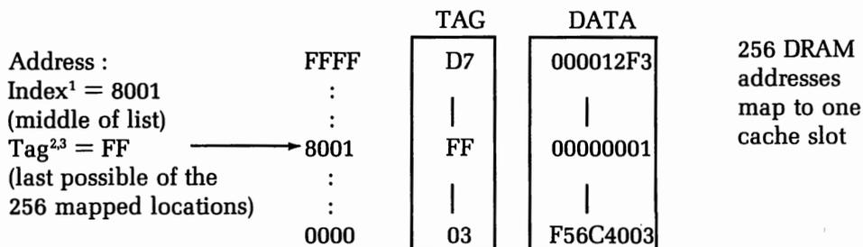
1. 16-bit Index tells which location of 64 K locations in tag SRAM to check.
