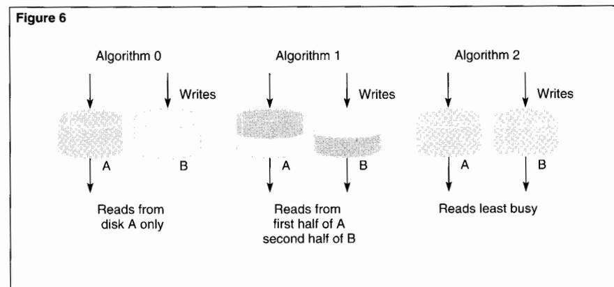
the device on which the head is closest to the data to be read. As shown in Figure 6, the Integrity S2 system implements a number of different read optimization algorithms and allows any of the algorithms to be selected on a partition-by-partition basis.
