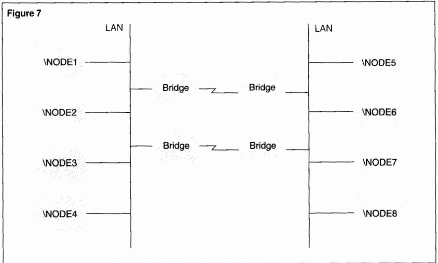
Switching to Expand over TLAM connections and bridge technology improves this configuration. A fully interconnected topology is achieved by installing a LAN at each site and connecting the LANs with a high-speed bridge. Expand processes can use the LAN to communicate with local and remote nodes with no passthrough hops. Improved fault tolerance and enhanced throughput can be achieved by adding more bridges to the configuration.
