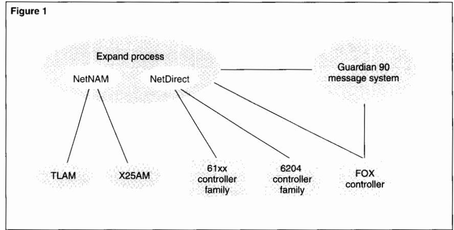
network. However, using a network service provider requires data to travel through another process at each end of a connection. Compared to a direct connection (FOX and NetDirect), additional system resources are needed to move data between nodes. One must weigh these and other considerations when deciding where and how to use the different connectivity options.
