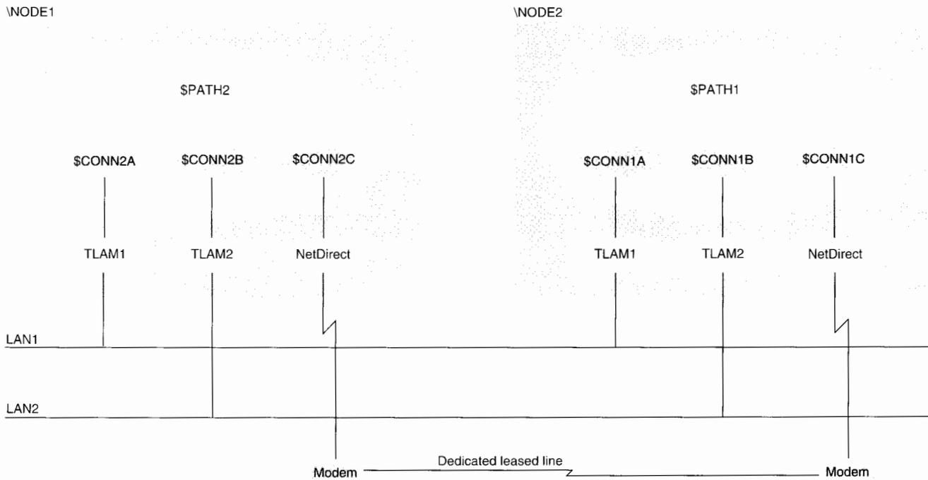
**Figure 6.** Extra fault tolerance is built into this configuration with the additional Expand NetDirect connection. The two Guardian 90 nodes can use NetDirect if the Expand over TLAM connections fail.
