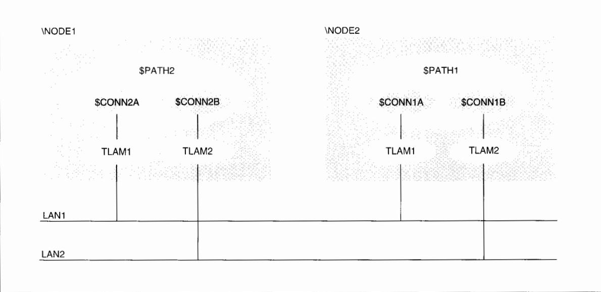
Figure 5. These two Guardian 90 systems use multiple Expand over TLAM connections and two parallel LANs to increase throughput and fault tolerance.
