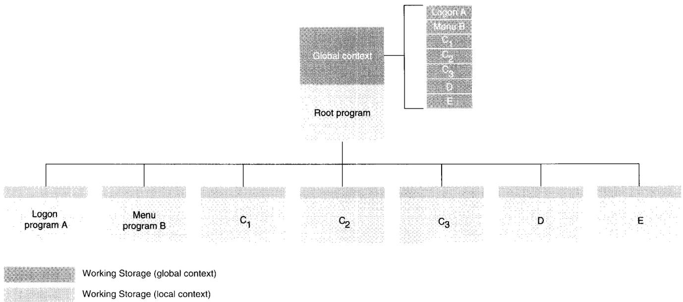
Figure 4 shows an example of a flat application call sequence. To complete its processing, program C<sub>1</sub> informs the root program (through its Linkage Section) that it should call program C<sub>2</sub> the next time it gets control. Program C<sub>1</sub> exits to the root program, which calls program C<sub>2</sub>. The same call sequence occurs to execute program C<sub>3</sub>.
