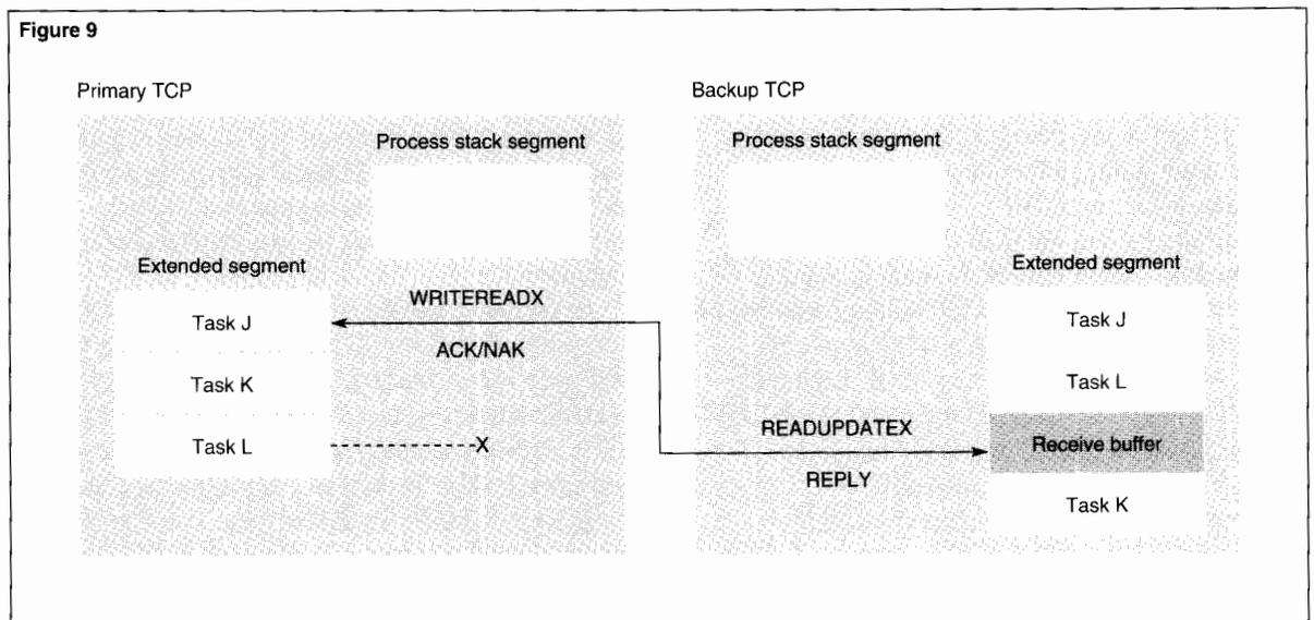
Figure 8 shows the first step in a task context checkpointing operation performed in a C10 (or later) release of Pathway. The TCP maintains a pool of slot areas. The backup TCP dynamically allocates one of the slots in this pool for its checkpoint receive buffer. (The TCP implicitly configures one extra slot so that a slot is always available for this purpose.) Next, it issues a READUPDATEX message and waits for the primary TCP to send checkpoint data.<sup>4</sup>
