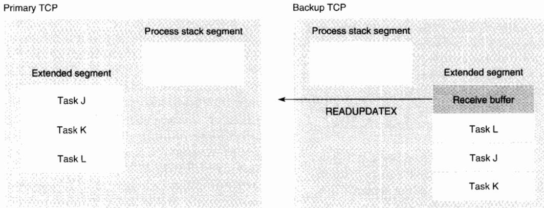
Figure 10. Step 3. The backup TCP commits the completed checkpoint to Task J. The slot that held the old task context of Task J becomes the new checkpoint receive buffer. Task L, which was waiting, can now transfer its task context to the backup TCP.
