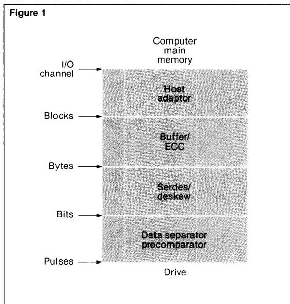
Figure 1. Model of I/O subsystem with computer and drive. The names of the interfaces between the layers of the subsystem correspond to the form in which information is transferred.
