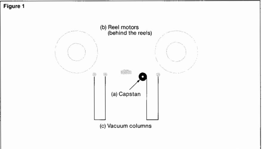
The capstan is a wheel, usually covered with rubber. As it turns, it pulls the tape over the read/write head. The capstan is connected to a motor, a tachometer, and control electronics. These components form a feedback system that controls the tape speed to within a few percent.
