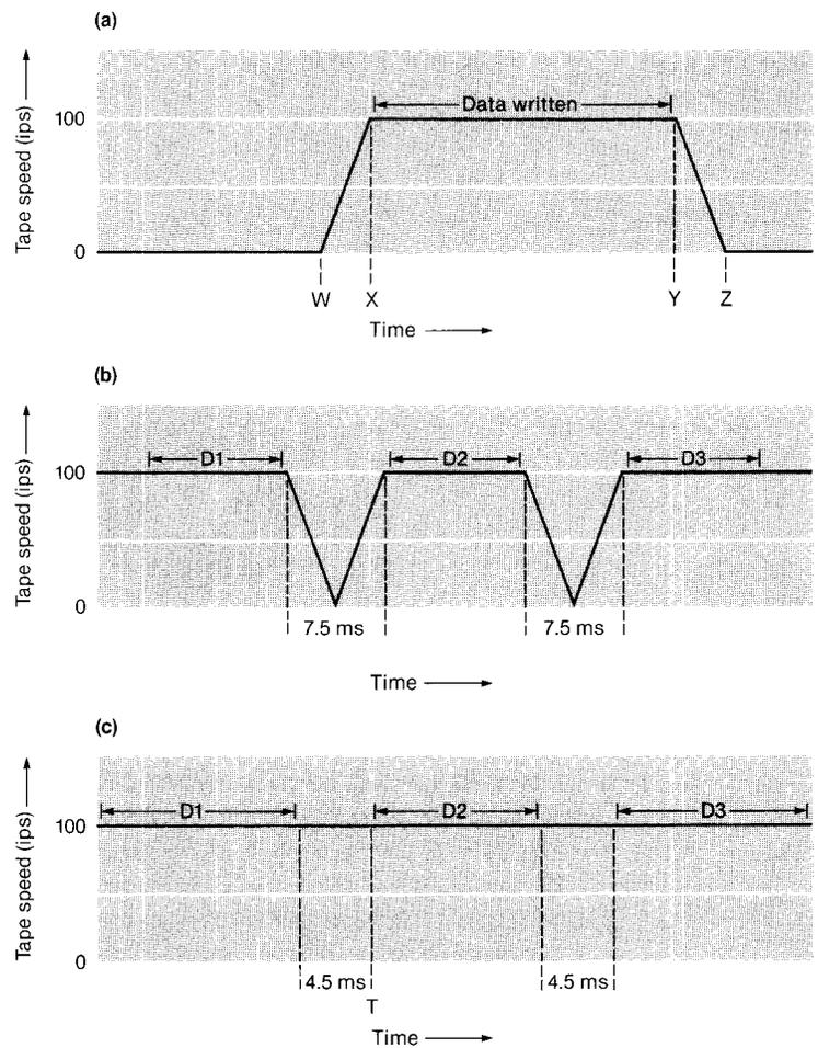
To maintain a standard interblock gap on the tape, the drive will assume that it is to stop after each block unless it is told very soon after writing a block that another is to be written. This delay is called the drive's *reinstruct time*.
