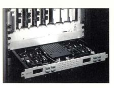
ates over a SCSI 1 or SCSI 2 host channel with burst rates of up to 20 MB/s, while Imager 2 runs at up to 40 MB/s (UltraSCSI) from the host to the drive and supports robotic tape libraries.
