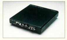
FLX-2000 is offered in four versions: Fibre Channel (1.062 Gb/s), Gigabit Ethernet (1.25 Gb/s) and ATM (155 or 622 Mb/s). Pricing starts at \$7,500.
