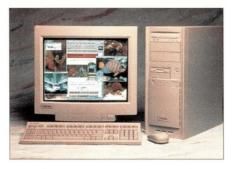
Designed for high-end applications in the engineering, medical research, animation, geophysics and finance industries, the COMPstation U10-300 has 512 KB of external cache, 64 MB of memory (expandable to 1 GB), one 4.3-GB hard drive, one 1.44-MB floppy drive and one PCI graphics card. In addition, it supports
