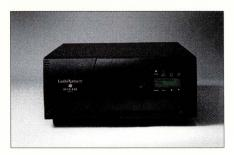
All LoaderXpress functions can be managed via front-panel controls that provide direct access to magazine, cartridge and drive status information. For extra security, the loader can be locked, preventing unauthorized access to critical company data, Overland says.
