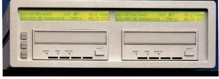
**STRIPING MODE** maximize performance by writing to multiple tapes simultaneously
