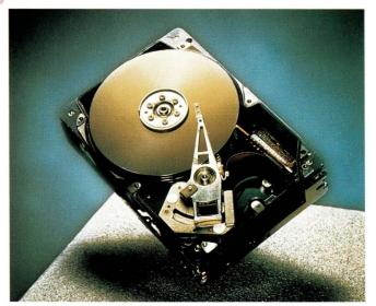
In addition to developing a version of Giant Magneto-Resistive heads, Fujitsu plans eventually to include stictionfree slider technology in all its disk drives.
