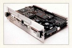
tained bandwidth: the Visual Instruction Set (VIS); up to 1 GB of RAM and 1 MB of FLASH memory; dual Ethernet, dual Fast SCSI-2 ports, and two RS-232 or RS-423 ports; and a high-performance VME64 interface.
