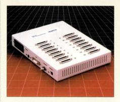
Model 466 features up to four network connections per port, for a maximum of 64 connections per 16-port unit. Ports can be configured as dedicated connections, Telebyte says.
