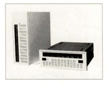
RAID controller. The SA-H335 comes in tower and rack-mount configuration. In either design, the product supports eight hot-plug drive slots with steel canisters for the disk drives. It also has dual redundant hot-pluggable power supplies, a fast/wide SCSI interface, automatic drive bay power sequencing, support for multiple SCSI hosts, mounting and power for a RAID controller and an optional 3½-inch tape/optical drive canister.
