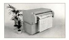
Document Folder. The document folder automatically activates when the plotter outputs a D- or E-size plot. The folder senses the plot size and adjusts itself to fold the plot into an 8½-by-11 inch or 9-by-12 inch packet, then stacks it with the title block out. When the print flow stops, the document folder shuts down and reactivates upon the next plot's output.
