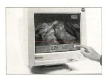
The company says the IntelliTouch may find roles in applications such as public information kiosks, process control and computer-based training. The monitor has a 1,280-by-1,024 resolution and a vertical refresh rate of up to 100 Hz. Pricing begins at \$1,980.
