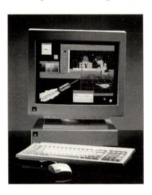
DataStation 20 comes in single-, dualand quad-processor models. It is based on the 50-MHz and 60-MHz versions of the SuperSPARC.
