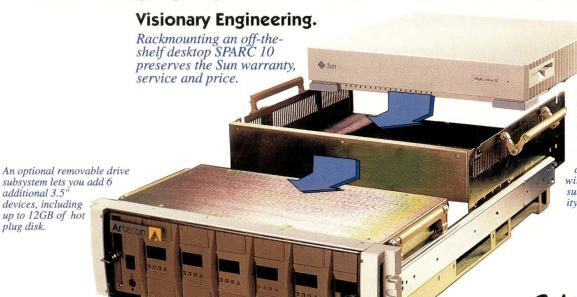
With essentially the same footprint as a SPARC 10, the Sphinx adds two additional 3.5" or half height 5.25" devices, and serves as either a stand alone chassis or mates with the removable drive subsystem for high capacity requirements.
