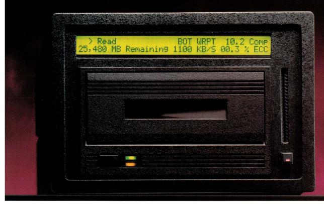
The CY-8500 can store up to 25 GB on a single tape, at speeds of up to 90 MB per minute, completely unattended.
