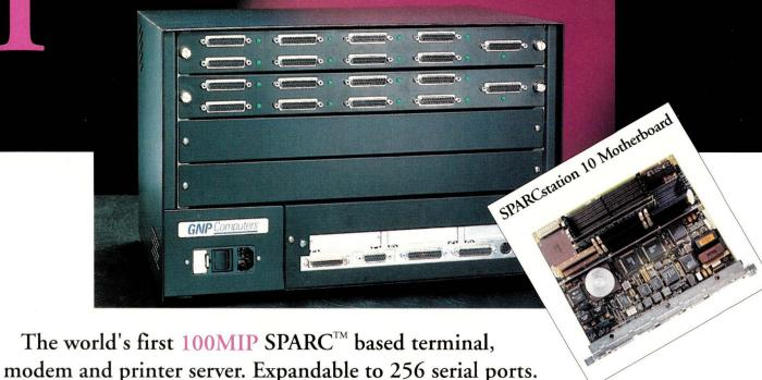
The DEI-10 WorkServer is a computer that combines the 100 MIP performance of a Sun SPARCstation™ 10 motherboard with GNP's expandable multiport serial and parallel device.
