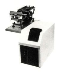
Circa 1972, 2,000 bytes per card magnetic card readers were the "state of the art" in storage and retreival. And we were there with the technical sales support and service needed in the emerging technologies of the 70's & 80's.
