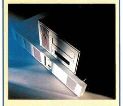
Fujitsu's 3480 Compatible Tape System provides high speed tape transfer in a rack mount or table top configuration. Up to 4 GB capacity with ACL and compression. Includes SCSI, Pertec and STC interfaces. Easy-to-use control panel allows access to extensive diagnostics.
