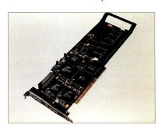
Mylex's own intelligent firmware, the controller decouples disk drive I/O management tasks from the network operating system, freeing the operating system to service other applications, the company says. The controller further eliminates potential I/O bottlenecks by incorporating a 33/66-MHz 64-bit PCI bus, which doubles sustained transfer data rates to more than 190 MB/s. The bus itself provides burst data transfer rates up to 266 MB/s.
