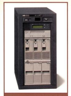
The SureStore HD Server 4000 is HP's first foray into the network-attatched storage market. The new system connects directly to Ethernet LANs and offers 18 to 90 GB of RAID 5 storage.
