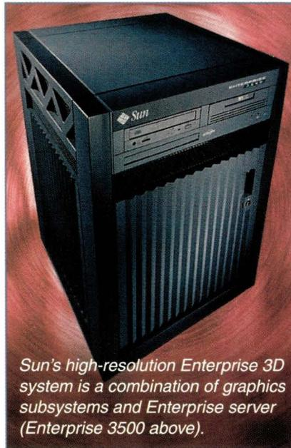
*Sun's high-resolution Enterprise 3D system is a combination of graphics subsystems and Enterprise server (Enterprise 3500 above).*
