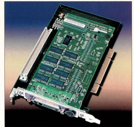
ator offers resolutions of 640-by-480 to 1,280-by-1,024 pixels and 8-, 16- or 32-bit color per pixel for Solaris 2.5.1/2.6-based systems. The EclipsePCI includes a built-in Sun 4/5 keyboard port, enabling multiple users to interface directly with the server without the addition of client workstation, and comes with either 2 or 4 MB of EDO DRAM.
