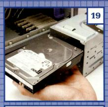
Let's get our hard and floppy drives installed in the two removable drive bays. Starting with the HD, simply slide in the drive so that its "rear end" is sticking out the back. Then just screw it in. Huh huh.
