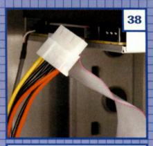
Each drive in your system needs to be connected to a power cable. Hard drives and CD/DVD-ROM drives take the same type of power cable, shown here. They go in only one way - unlike The Vede.
