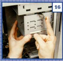
The plates come out from inside, so we're going to need to gain access. This Antec case makes things a cinch by allowing us to pull out its two 3.5-inch drive bays.
