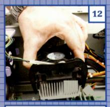
Flip the heatsink's levers into the "open" position. Line up the four corners with the four posts coming up from your mobo. Make sure the heatsink's "teeth" latch on to each of these four corners.
