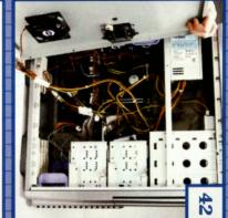
System is built. All parts are installed, cabled, and juiced. Yeah, it's damn ugly, but then, we're lazy. To ensure better airflow inside your case, conside wrapping up loose wires with cable wraps or ties
