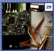
Read your motherboard manual carefully to learn where each cable goes. If a button or light isn't working after the system is completed, try turning the offending cable around.
