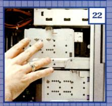
Make sure your floppy drive is sticking out just far enough from the end of the drive bay so that it'll be flush with the outside of the case once it's back inside the tower.
