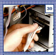
The floppy drive ribbon works only one way, but it may fit in backward or reversed. If your drive doesn't work once you've powered up, turn the PC off and switch the ribbon around until the drive works.
