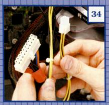
Now plug the system's power supply into the motherboard. P4-based motherboards use two different power cables. Both need to be plugged into the motherboard before you turn on the system.
