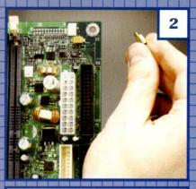
Install one mounting screw in your case for each one of your motherboard's screw holes. Line them up properly! Place one under the motherboard in the wrong place, and the system may not boot.
