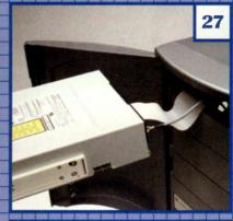
Now that the jumper is set and the cables are plugged in, feed those cables right through the front of the tower and snap the drive itself into place so that the drive face is flush with the case.
