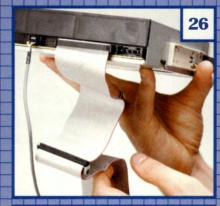
Most IDE cables come with a blue end and one or two black ends (one each for each of the two devices you can use per IDE channel). Plug one of the black connectors into the drive as-shown.
