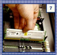
Your RAM and C-RIMMs fit in only one way. The levers on each side of the RIMM slot should be in the "open" position. Push the sticks straight down into the motherboard until both levers snap up.
