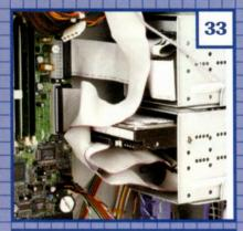
Plug the blue connector from the hard drive into the primary IDE slot and the blue connector from the DVD drive into the secondary slot on the mobo. Plug the ribbon from the floppy drive into its slot.
