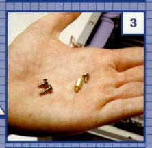
Your case comes with many screws. Make sure to use the right ones. In this instance, the small screw with fine threads is made to work with the gold-colored motherboard mounts.
