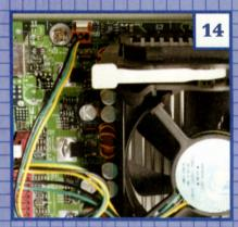
Plug the fan's power cable into the little threepronged connector on the motherboard next to the CPU socket. Depending on the motherboard, it'll usually say "CPU FAN" right next to it.
