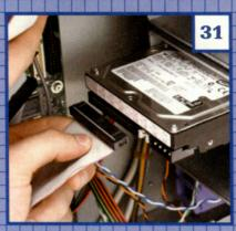
Almost without exception, IDE cables fit in only one way. Make sure you've lined things up properly and plug one of the black connectors from your second IDE ribbon into your hard drive
