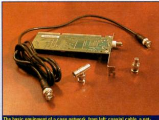
The basic equipment of a coax network, from left: coaxial cable, a network interface card, a t-connector, and a 50-ohm terminating resistor
