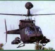
This state-of-the-art scout helo is the Longbow's eye in the sky. It uses a mast-mounted (i.e. above the main rotor) Target Acquisition and Display System to peer over ridge lines and get a detailed picture of enemy positions without exposing itself to anti-aircraft fire.
