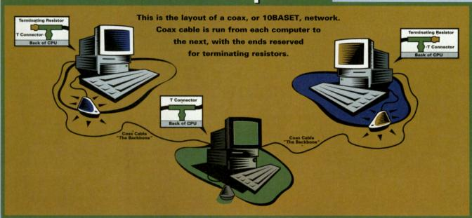
the network we are building; PCI NICs do not offer any advantages on this type of network.
