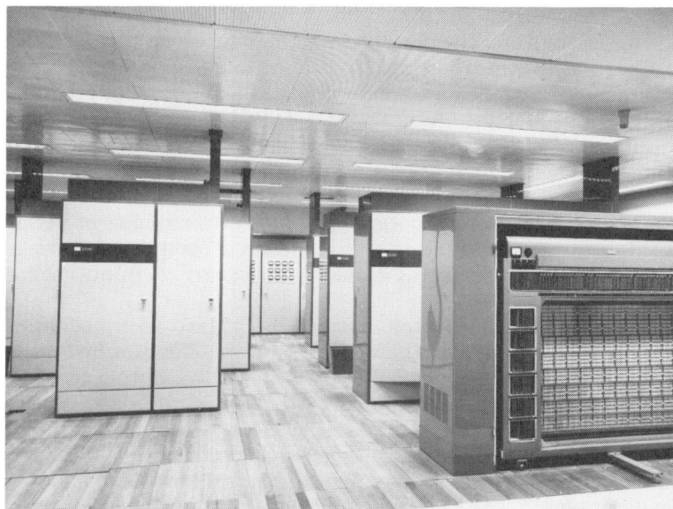
Fig. 5 The London University Atlas installation c. 1963 (Lower floor, showing main processing units)
