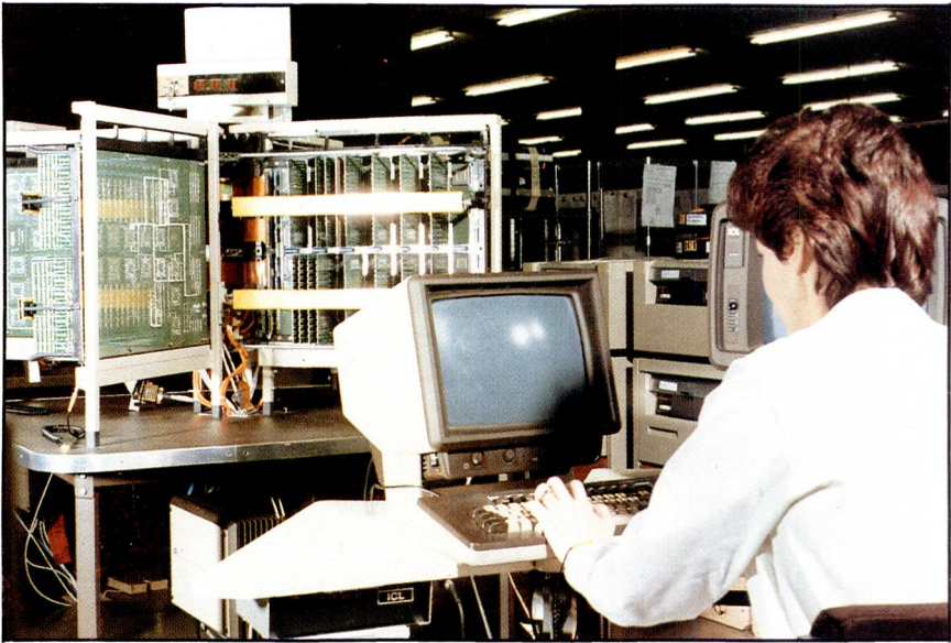
Fig. 3 Opened-out node test rig after assembly and prior to installation in cabinet
