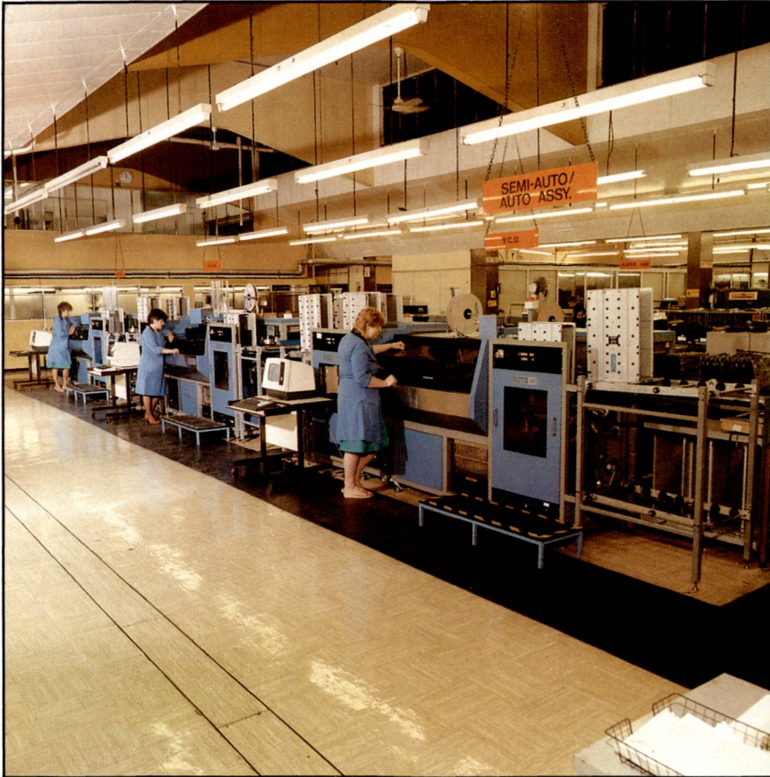
Fig. 3 Universal multi-mod automatic insertion machines
