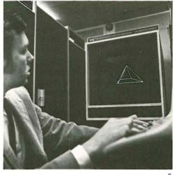
Operating the LDS-1 display is only one of the tasks that the PDP-10 can perform. At the same time that the display is in operation, graphics and other programs can be developed on-line by as many as 63 simultaneous users; batch processing can be performed for multiple program streams, or the system can handle other real-time
