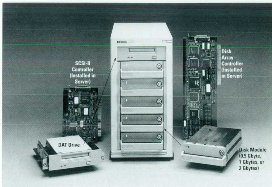
Fig. 2. The components of an HP storage system. The SCSI-II controller, the disk array controller, and the disk module make up the HP Disk Array.
