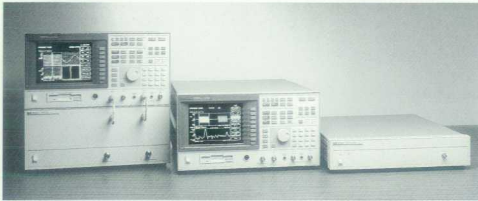
Fig. 1. The HP 89410A vector signal analyzer (center) is a 10-MHz baseband analyzer. It acts as the user interface, final digital IF, signal processor, and display section for the HP 894xxA family of analyzers. The HP 89440A RF section (bottom left) extends the analyzer's capabilities up to 1.8 GHz. The HP 89411A (right) is used with a higher-frequency analyzer to extend measurement coverage to frequency ranges above 1.8 GHz.
