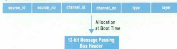
Fig. 6. Every message has a composite symbolic identification, which is evaluated at boot time, when message headers are allocated.
