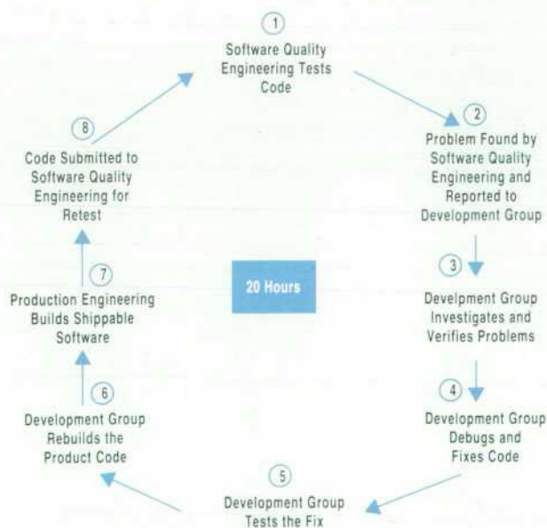
Fig. 2. Software defect find and fix cycle.
