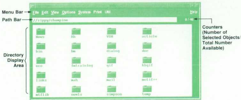
Fig. 3. The main window of the visual shell.
