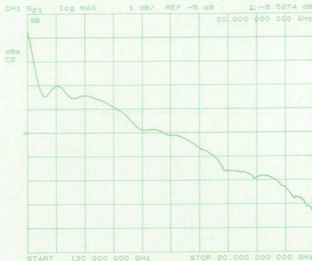
Fig. 7. Optical modulator RF insertion loss.
