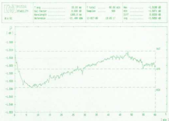
Fig. 12. Plot showing the results of an HP 8153A A/B stability measurement, produced without programming.
