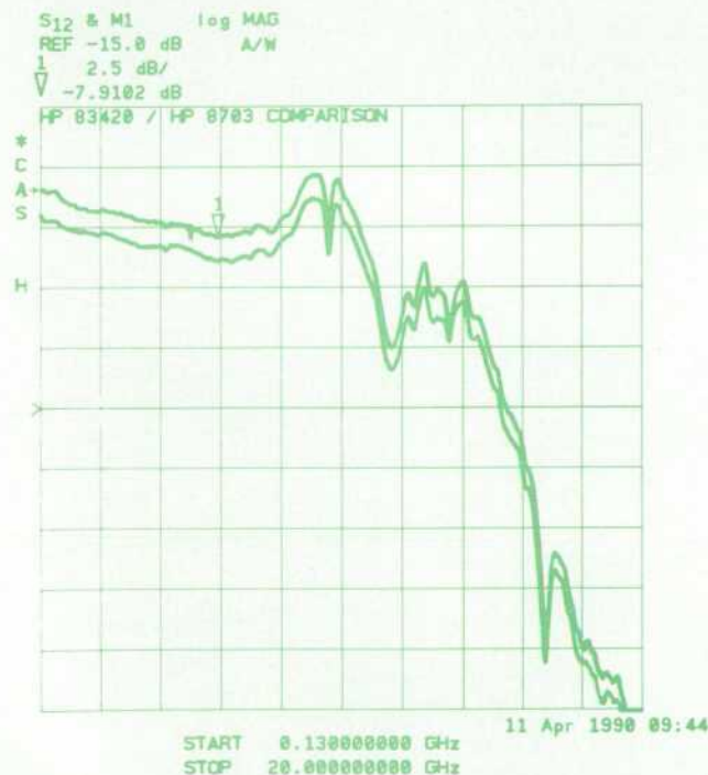
Fig. 12. Measurements of the same photodiode receiver by an HP 8703A lightwave component analyzer and by an HP 83420A/HP 8510B system. The differences are similar to these between HP 8703A analyzers.
