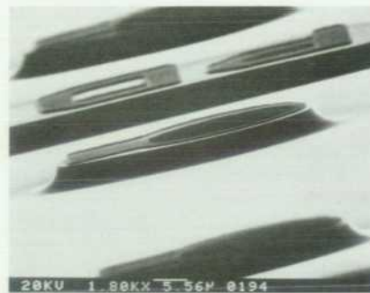
Photodiode Mesa Surface 1:1:1 (1N)K_2Cr_2O_7:CH_3COOH:HBr
