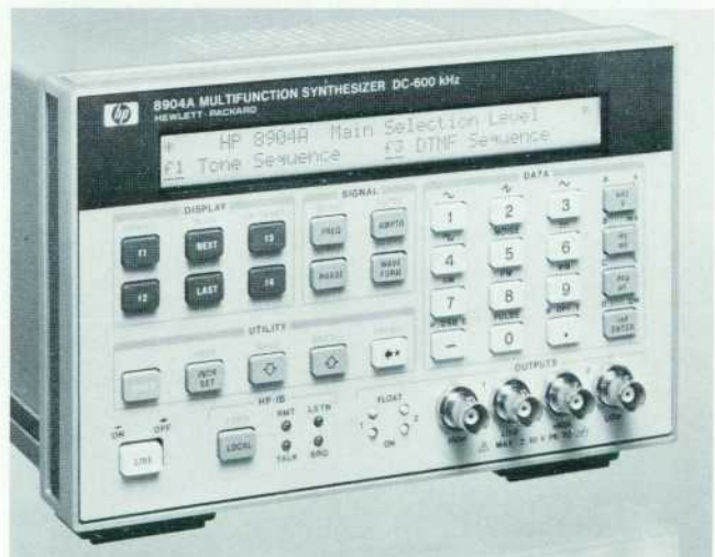
Fig. 1. The HP 8904A Multifunction Synthesizer uses the latest VLSI technology to create complex waveforms from digitally synthesized sine, square, triangle, ramp, Gaussian white noise, and dc waveforms. In addition to the standard internal synthesizer (channel), three more identical internal synthesizers can be added. The option that adds the three additional synthesizers also provides AM, FM, \phi M, DSBSC, and pulse modulation. Application areas for the HP 8904A include audio testing, navigation, commercial electronics and communications.
