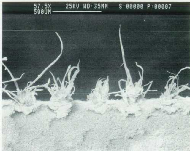
Fig. 8. Depending on the paper and other factors, fibers in the paper can be separated in the perforation process.
