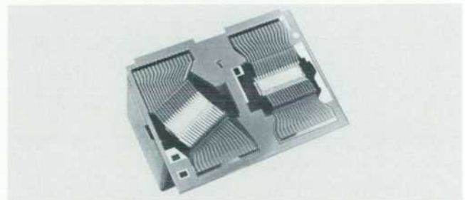
Fig. 7. A leadframe in contact with print cartridges.
