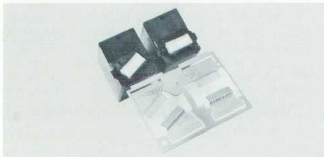
Fig. 6. The leadframe has 64 contacts in four groups.
