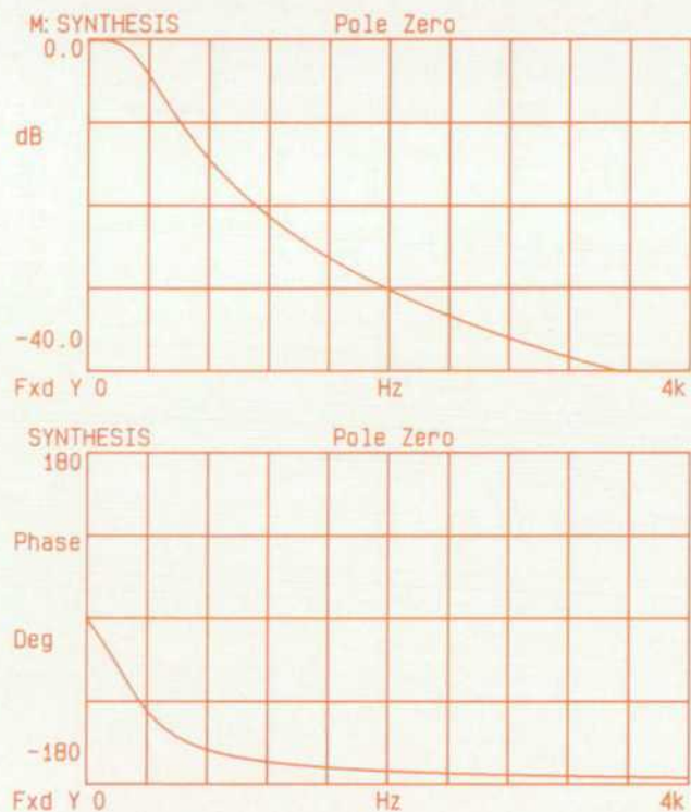
Fig. 13. Response of additional G_1 element designed to meet loop roll-off goals.
