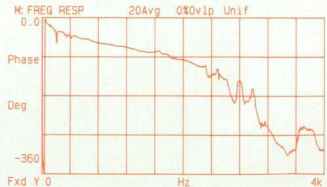
Fig. 12. Compensated open loop system response.
